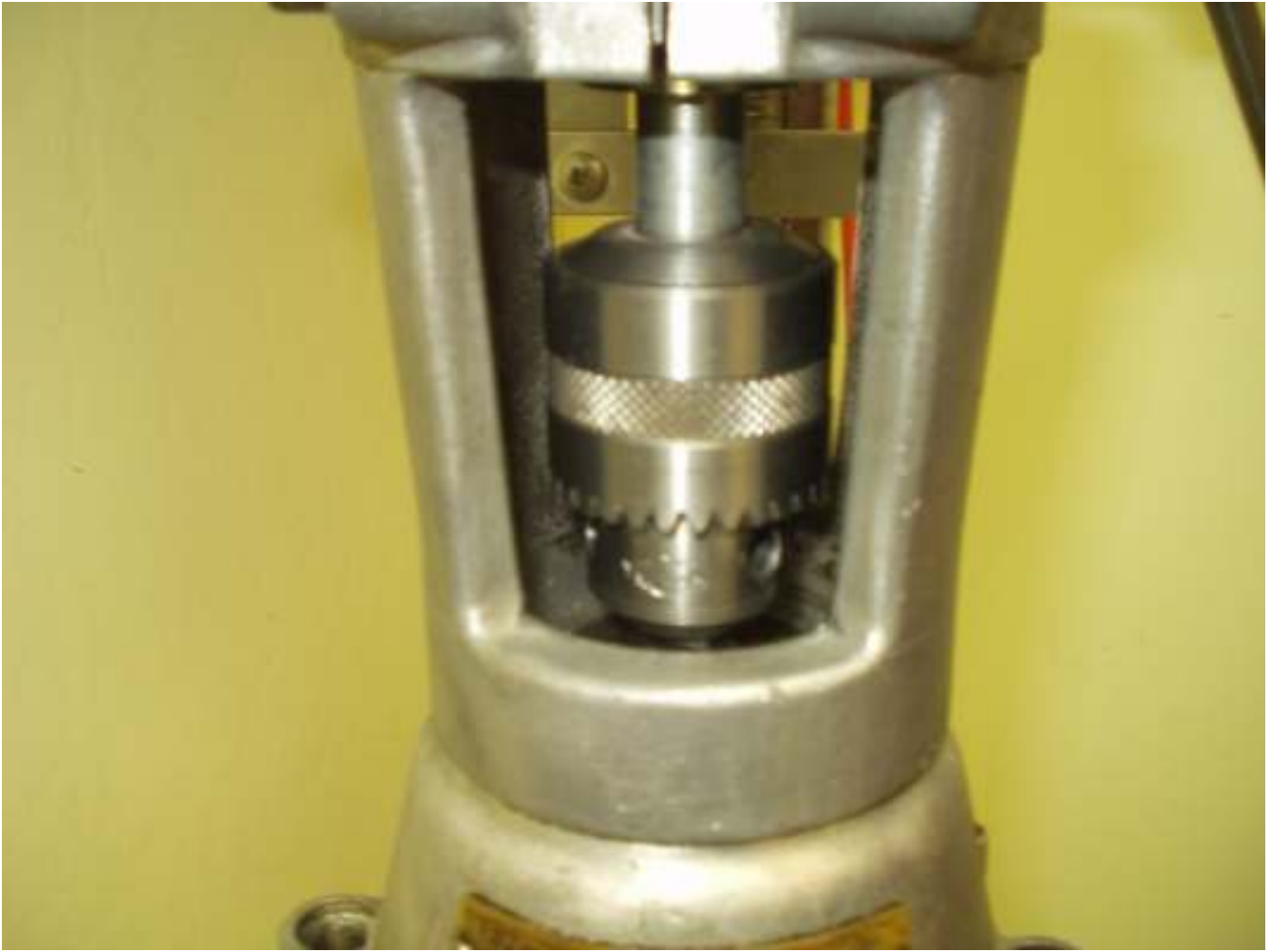
Here you can see a little of how the drill chuck attaches to the tapping head.
