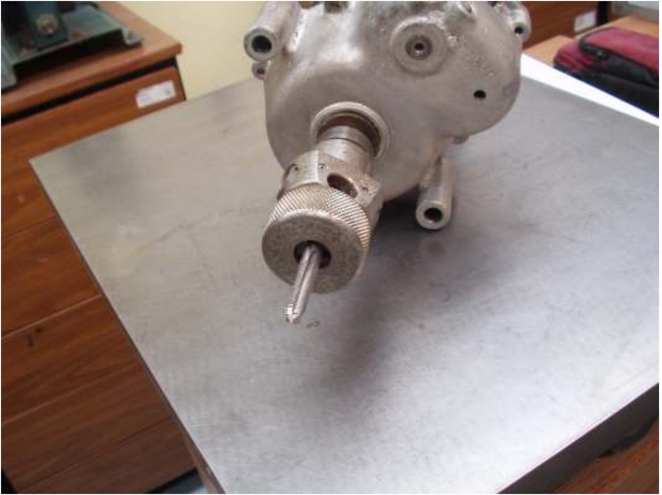
The tap chuck has 3 spring loaded fingers that adjust to hold a little less than 1/4" to maybe 1/2".
