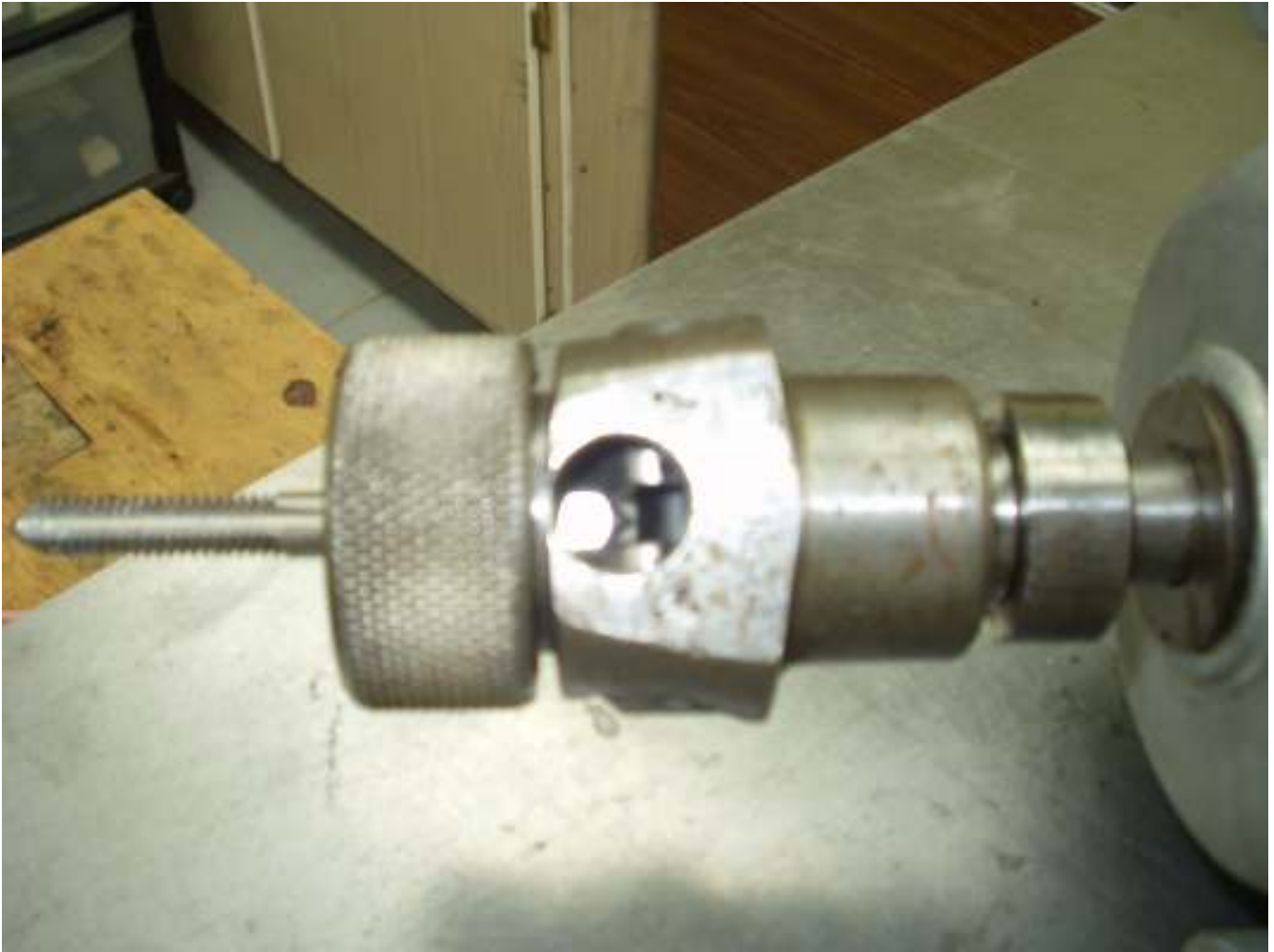
You can see the floating vise that holds the square shank of the tap to the right of the chuck.
