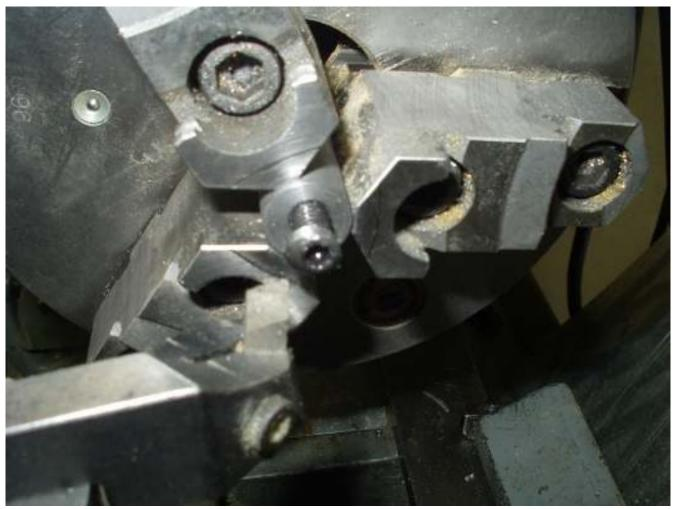
The head of the screw has been cut and you can see the eccentric that forms. These screws came from Enco and were very easy to machine.
