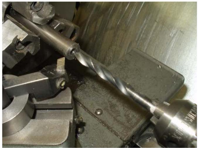
I started by drilling a through hole 5/16". This permits the washer to freely move on the screw body as it clamps the block being machined. Since I'm making 6 of these washers, it was most efficient to just drill as deep as possible.
