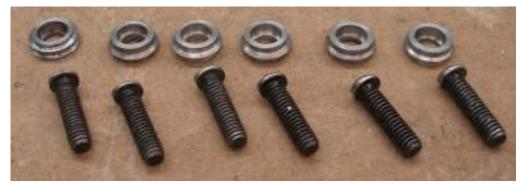
Along the top you see a set of cup like washers. They have a ridge around their perimeter that can cut into the metal being held. The screws started as button head screws but have been machined so the heads are eccentric. These screws have a hex hole in the top and are driven with an Allan key.
