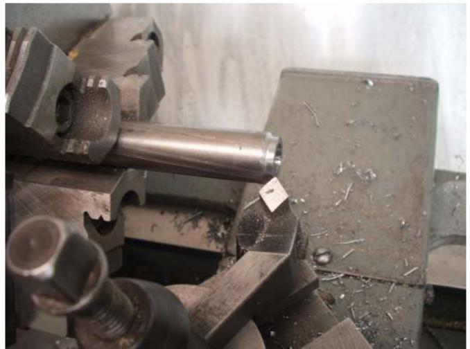
Forming the outside cutting edge was simple. I started by positioning my cutter as shown above. Then I measured over 1/8" from the edge. The lathe was started and I fed in just enough to make a line. The cutter was then moved to the right and fed in about 50 thou. I then fed in until I reached the line. The cutter was backed off and the lathe stopped.
