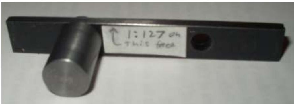
The goal is to make a sine bar with a slope of around 1:100. Mine came out 1:127, which is just fine. The error was due to the fact that the hole is not centered but I assumed it was. The critical bit is that the top surface of the parallel be perfectly flat and that the slope be accurately known. The best way to measure the slope is to measure the height at each end and divide by the length of the parallel.
