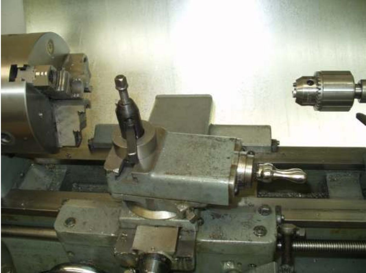
You simply set the compound so the feed is almost parallel to the ways. A large feed-in on the compound results in a small feed into the work. I'm sure this trick is as old as the compound.
