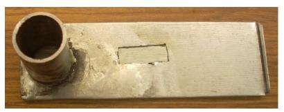
I first built it from card stock to be sure there were no obvious errors. Then the sheet metal was cut out and partially folded. The top piece shown above was drilled with a ¼" hole around the location of the pipe. This end was also sanded to remove most of the galvanized coating. A bolt was run through this hole to secure the pipe in position. With all surfaces clean, a bit of flux made the silver solder job easy. I did do this work outside just in case any of that zinc should burn off.
