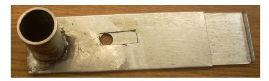
Here you see the slide plate in the open position. This punched hole was an afterthought and turned out to be a good one. I could have avoided cutting that square hole and just punched through both pieces. Then when the hole appears, I know the pipe is open.
