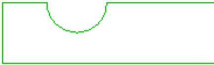
Here we have an end view of the block. As the cutter moves across the block's surface, we get a dished cut.
