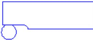
Set your axis indicator to zero and take a standard depth light cut with your end mill.
