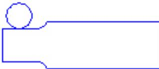
Move the end mill to the backside of the block. Take another standard depth light cut. Note the change in position front to back and call it D1.
