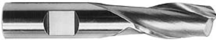
Vertical mills often use end mills. They come in a variety of styles and diameters. Although end mill diameter is typically specified as a given fraction of an inch, say  $7/16$ " , they are in fact typically ground to a precise diameter. Using a micrometer to measure a new  $7/16$ " end mill should show  $.4375$ ". That value is useful when you make a cut on the side of an end mill if you have defined zero as the center of the spindle.
