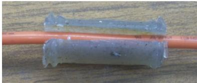
An alternative is to do a double mold. The first mold is a cylinder with a slot in it. I put a red wire in the slot to make it easier to see.
