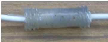
The second mold contains the wire and additional plastic to fill the slot.
