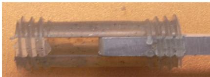
In this picture I have trimmed the part and partially inserted the aluminum bar so you can see the molded in slot. The threads cover the ends of the slot but are easily broken.
