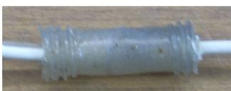
This is a later double shot mold that worked. The second molding does seem to be fused into the first one.
