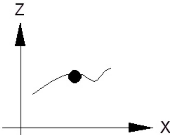
In the general case, the line is not straight. If you use your best measurement instrument and technique, the most you can hope for is that the line is straight and flat to the limits of your equipment. Look close enough and you will always see a line that is not perfect.
