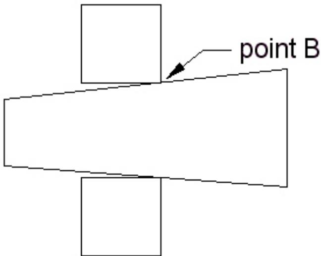
You can see that the mic's anvils only make contact on the up hill side of the block. A small movement of the mic will produce a different reading of the block's thickness.
