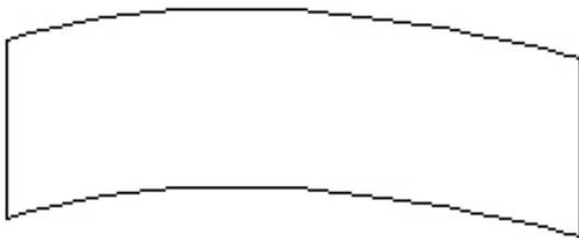
Consider the case of a 2D box that is curved on the top and bottom. You can mic the thickness and find it uniform. Yet if you put it on a surface and measure the height at various points, you will see the bend.
