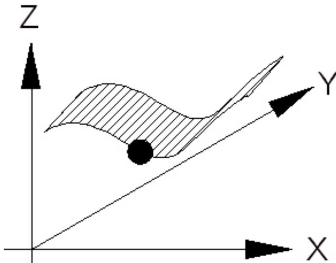
you a good idea of its contour. For a clearer picture of how the surface deviates from ideal, place the part on a surface plate and use a finger Dial Test Indicator to search the top for lows and highs. The finger is typically in contact with a much smaller area than the area of a square ended mic anvil and often is smaller than even the ball attachment to
