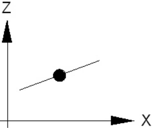
Consider the case of a line with a slope. At our control point, the distance from the X axis is known. But when we move away from this point, the distance to the X axis will either increase or decrease.
