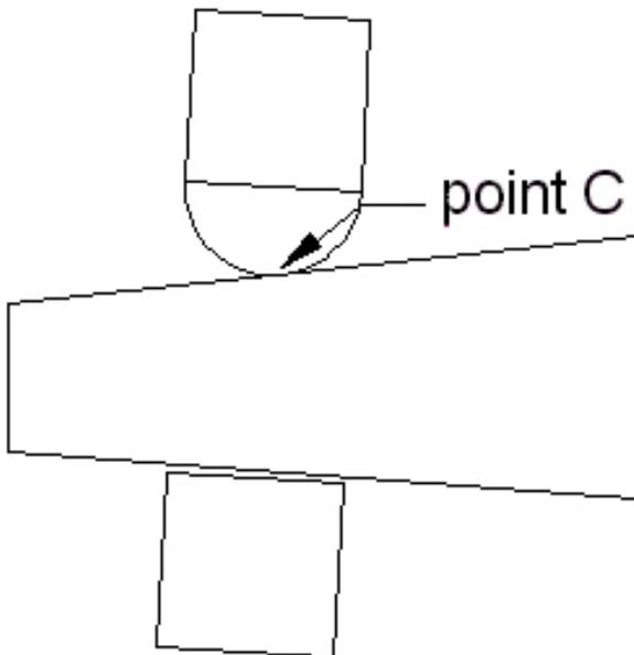
One solution to the problem of having a poorly defined set of contact points is to put a precision ball on the end of the mic's anvil.
