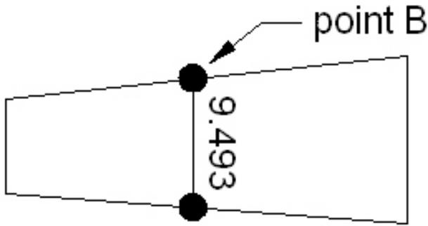
Now consider a block of the type type found in my shop. It is never perfectly square. I can pick a "point B", and put my mic on it. The reading is an accurate measure of a thickness only at this point. If
