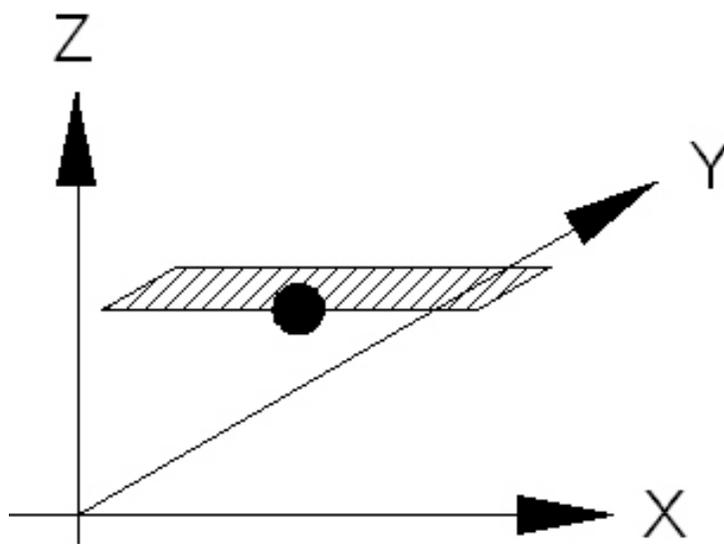
Entering the world of three dimensions means adding the Y-axis to our existing model of X and Z axes. Our line now expands to become a plane. All of our discussion related to two dimensions will apply here. We can define a single control point on our plane and use it to monitor and control the distance this point is from
