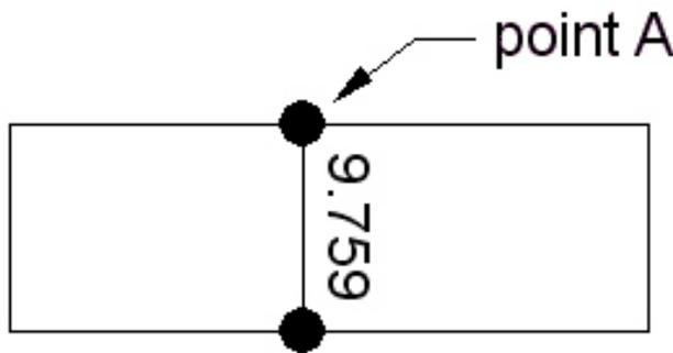
Consider a block of metal that is perfectly square. We can put a mic at "point A" and measure a thickness. Since the block is perfectly square, this measurement accurately represents the thickness of the block from end to end. I will call
