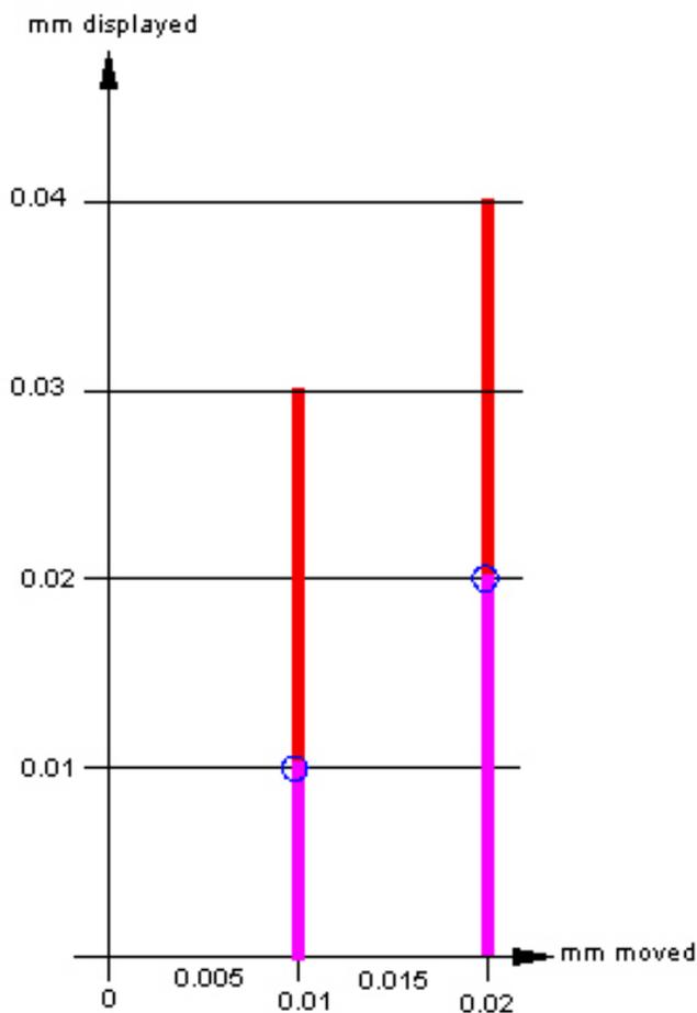
Ideal behavior is marked with the two small circles. The thick vertical bars are our uncertainty due to our error limits. The red part of each line shows possible values that are between ideal, 0 error, and the maximum of +0.02 mm. The purple line segment shows possible values that are between ideal and the maximum of -0.02 mm.
