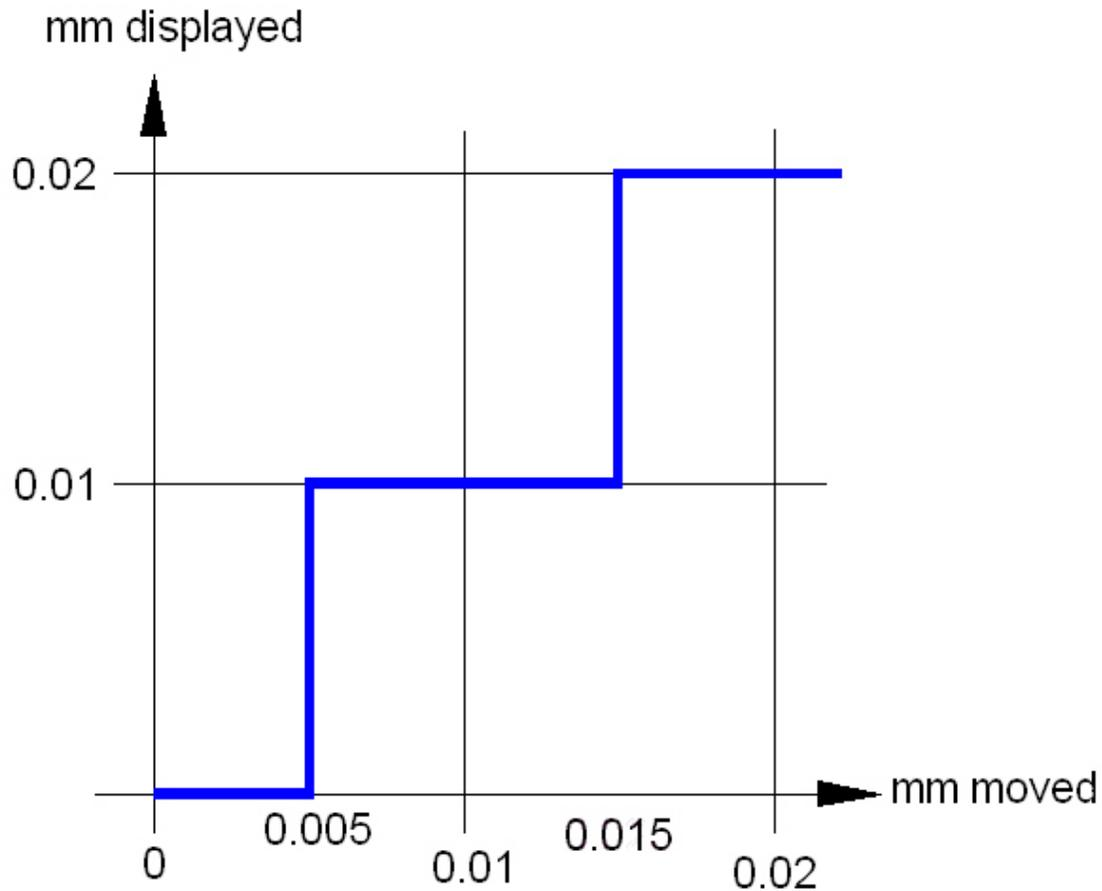
Now reset the caliper to 0 and slowly open the jaws. When we have moved to 0.005 mm the display will change from 0.00 to 0.01 mm. This is the point where we have an equal magnitude of round off error.
