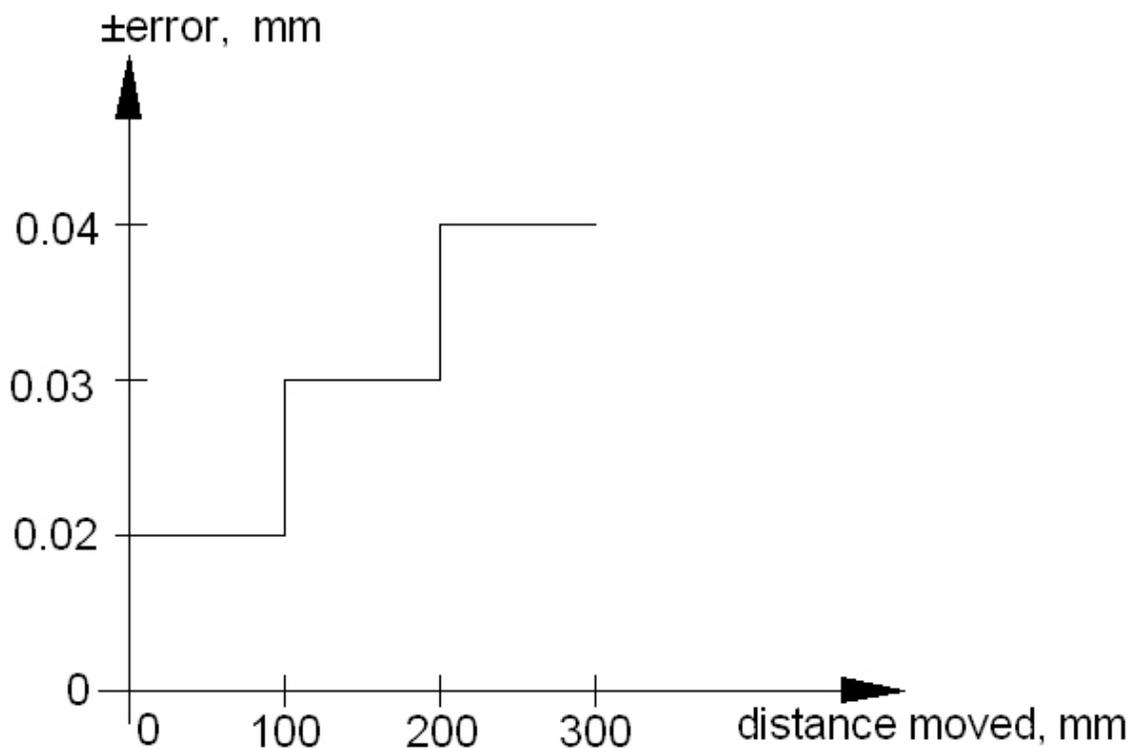
Between a distance moved of 0 and 100 mm, the actual error for a given caliper is bounded between  $\pm 0.02$  mm. When we move to between 100 and 200 mm, the actual error gets new boundaries of between  $\pm 0.03$  mm. Clearly there is a component of the error limit that is a function of distance moved.
