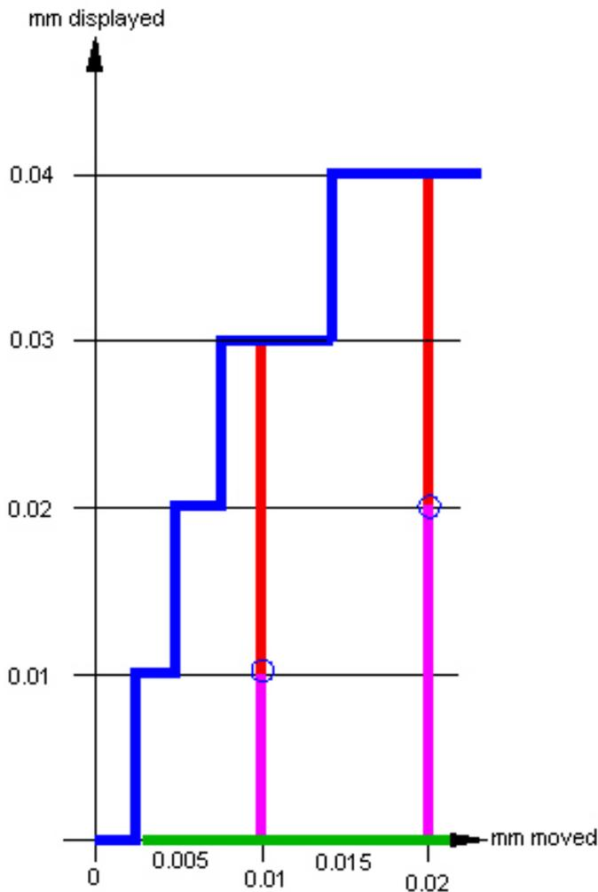
Now think about what this does to the display. At zero set it must read 0 but by moving 0.01 mm it must read 0.03 mm. It can only get there by first showing 0.01 mm and then showing 0.02 mm. Clearly the error associated with each 0.01 mm step can be large. For example, we could read 0.03 mm yet move less than 0.005 mm. We just have to display 0.03 mm at or before a movement of 0.01 mm.
