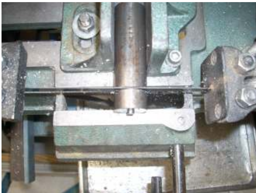
One end of a length of 1 1/8" CRS has a 1/4" diameter button machined into it. I then sawed off a length 5/8" long.
