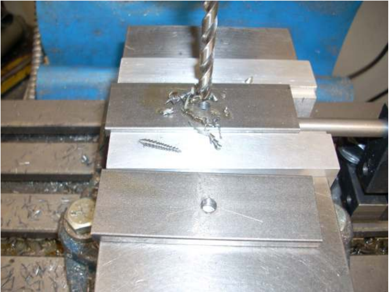
I drilled a 1/4" hole in the center of each bar to make alignment of the boss easier.
