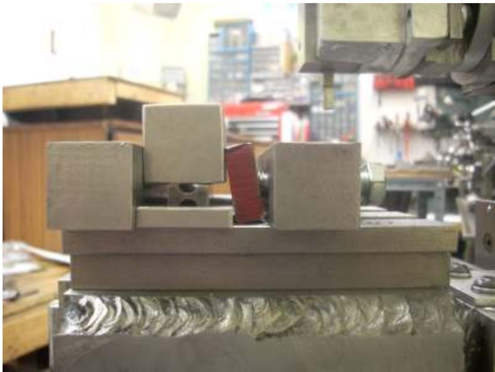
Here is a side view. My goal was to raise the block up enough to cut the V. This didn't work well as the block lifted a bit when hit with the cutter. The idea was to have a "Kurt Vise" action from the movable jaw (the tilting red bar).
