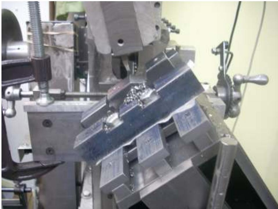
This time all went well. I'm using a sheet of paper between vise jaws and table. No more slipping jaws. I also did away with the sloping block between screws and block. The block stayed down much better with just a bar parallel to the part being cut.
