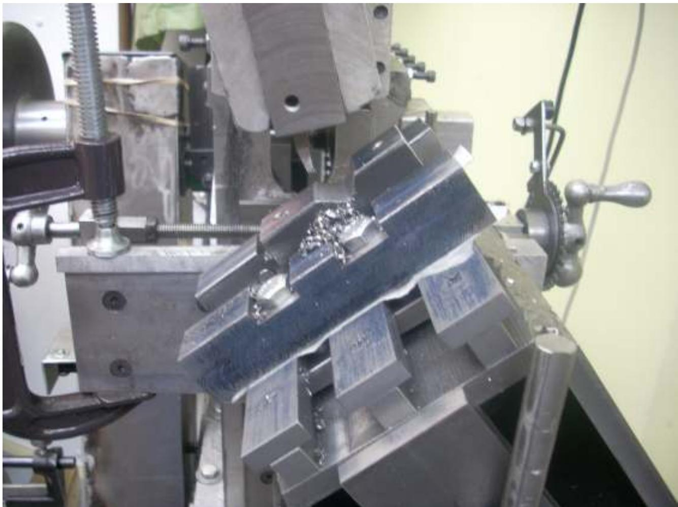
The shaper is a lot more useful when I can actually hold parts to be cut. Here you see my new vise holding a block of CRS as I machine a V into it. The C clamp on the left is a horizontal stop. One of my next projects will be to make a nicer stop.
