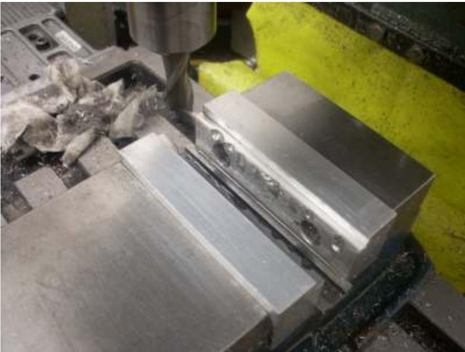
The first step in making the vise is to true up the soft jaws on my mill/drill vise. Note the parallel clamped in the bottom of the vise. This width is about the same as the blocks I will machine.
