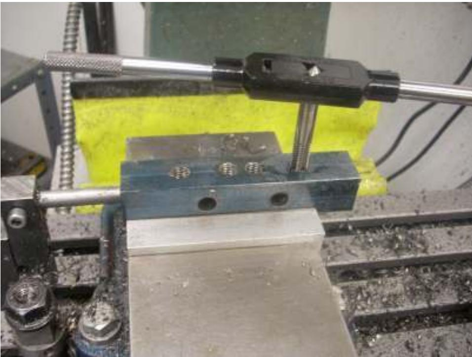
The horizontal holes are a loose fit to the bolts I have selected. These bolts will engage the T nuts. The holes being tapped use the same size bolts and will clamp the part being machined. I placed the tapped holes so there are 0.5" from the T nut bolt holes. Only later did I realize that the two center tapped holes are too close together. If I try to put a bolt in each hole, the heads hit.
