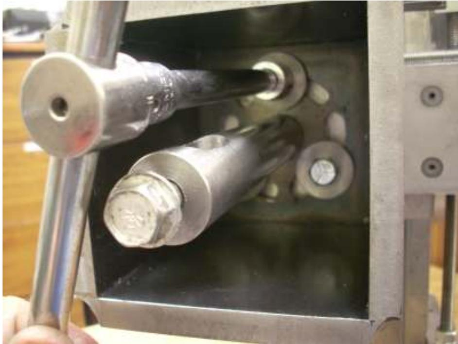
Here you can see how easy it is to loosen these bolts. The bolt heads are the same size as all other bolts needing adjustment in the shaper. The extension is long enough to clear the pivot pin.
