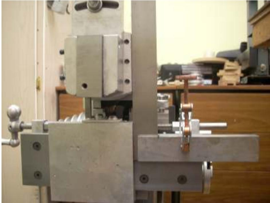
To locate the scale, I first set the head true with respect to the cross slide. You can see my square clamped in place and the head touching it.
