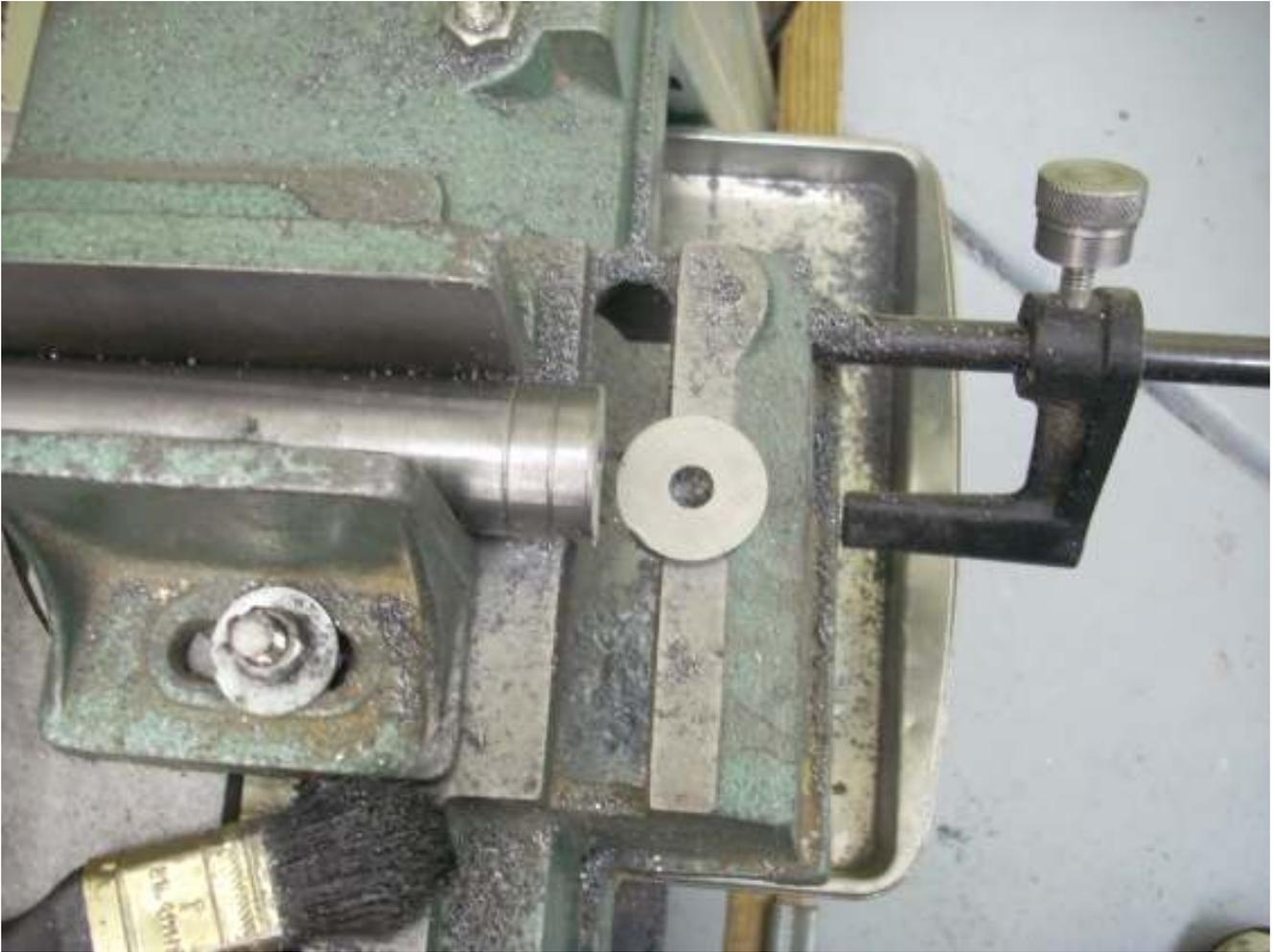
The first washer has been cut. One side was faced on the lathe and the other face is rough and probably not true.
