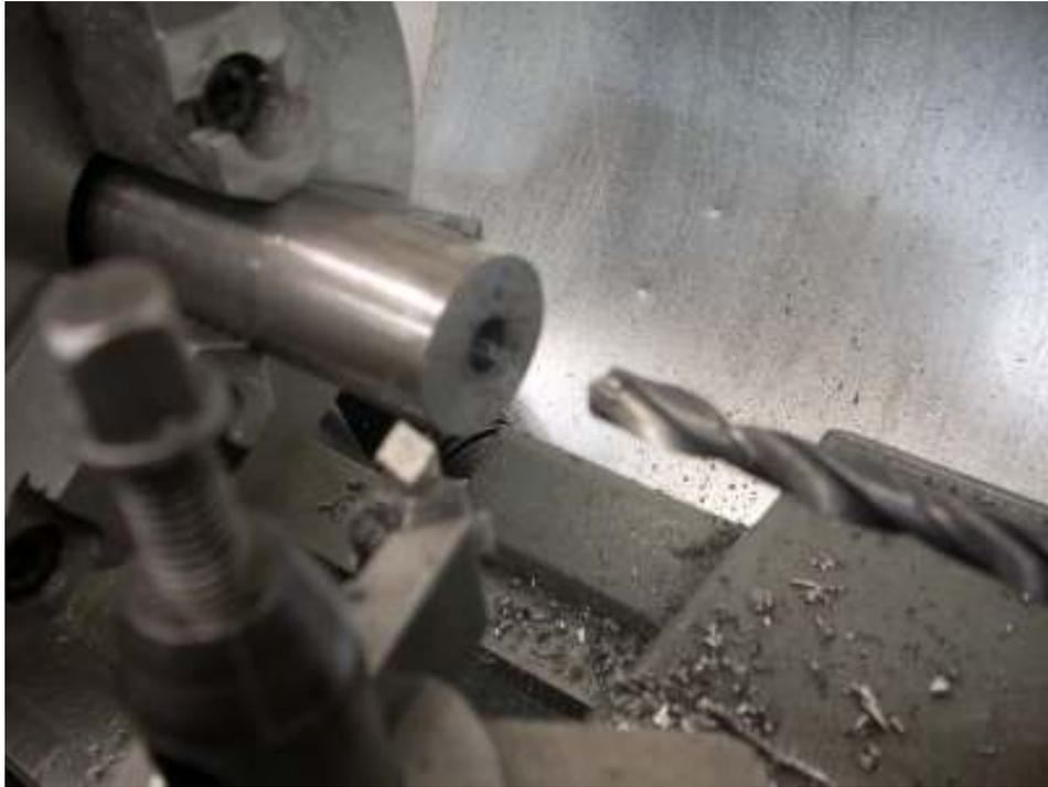
I then drilled a  $5/16$ " holes 1" deep and tapped it  $3/8$ " -16 to accept the locking screw. This was a mistake as I found out later.
