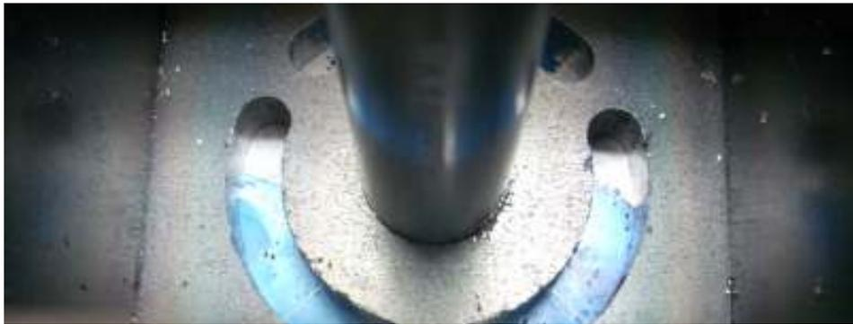
You might be able to just make out the scribed lines here. We are looking down into the cube which has been mounted on the pivot pin. The trick is to mark the center line of each arc on the line.
