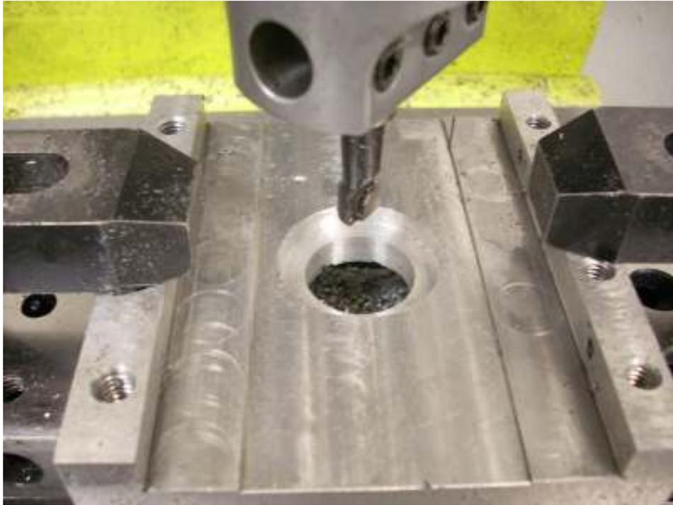
I decided to go with a D ring that would snap into a groove in the pivot pin. The D ring fits snugly into a recess which will keep it closed. This required me to flip the casting over since the recess, which must be concentric with the 1" hole, had to be on the other side.
