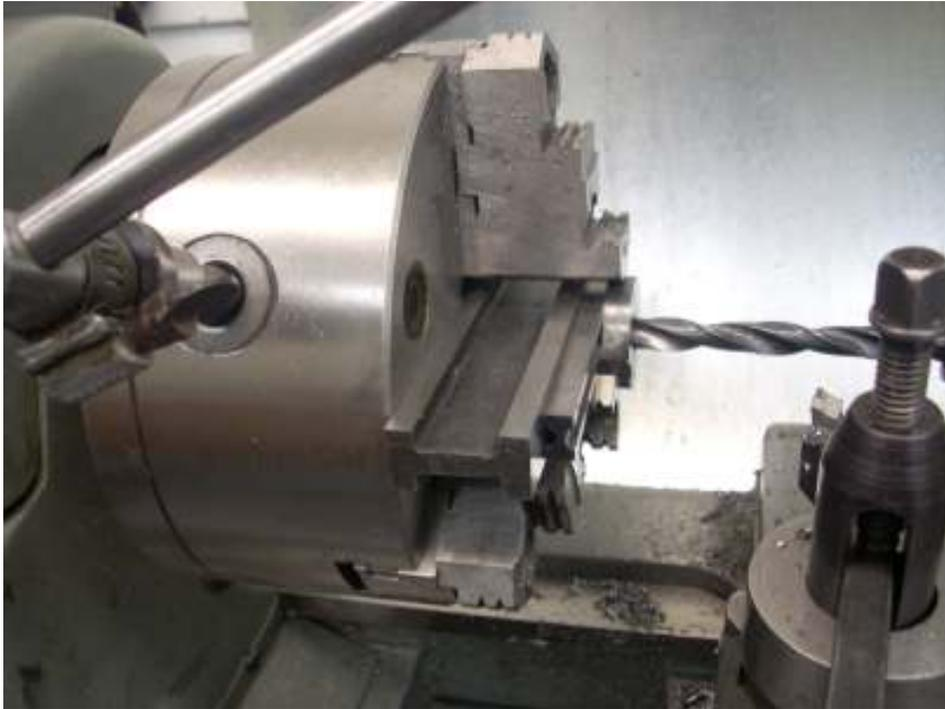
I am using the drill to hold the washer and a set of parallels to set it true in the chuck. The parallels *are* removed before the lathe is turned on.
