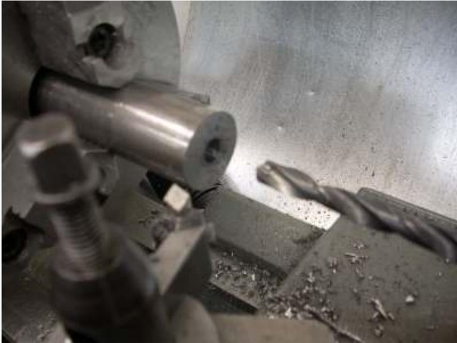
I had some 12L14 of the correct diameter. After facing off, I drilled a 3/8" hole about 1" deep. The cutter was then used to mark off slabs 0.3" wide.
