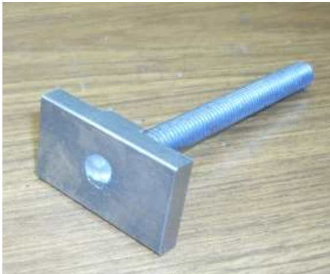
After the threaded rod was cut to size, I used red Loctite to secure it to the "bolt".
