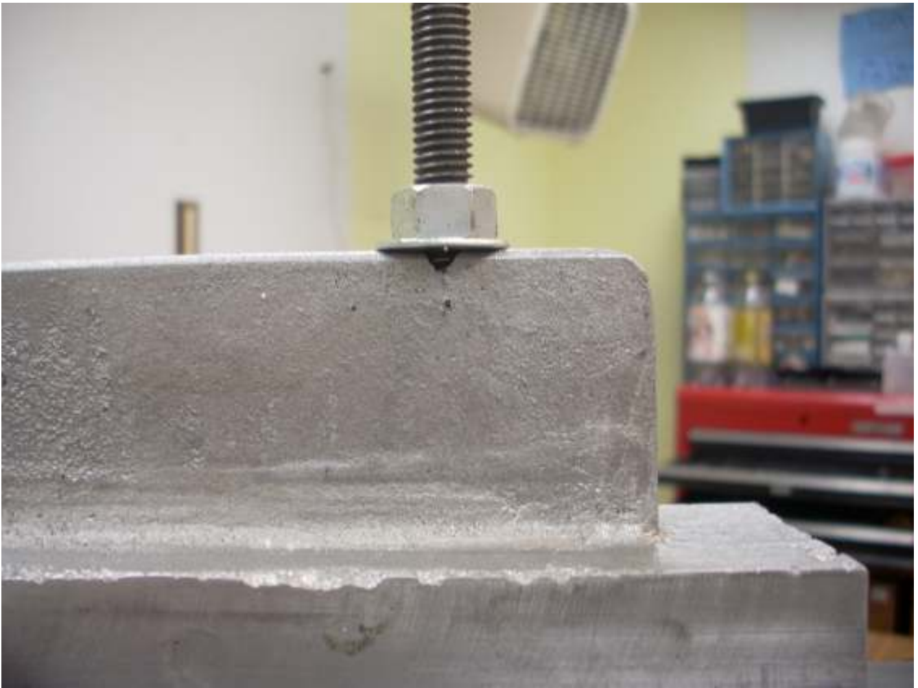
Here is the messed up side. You can see the side of the hole just breaking through at the top.
