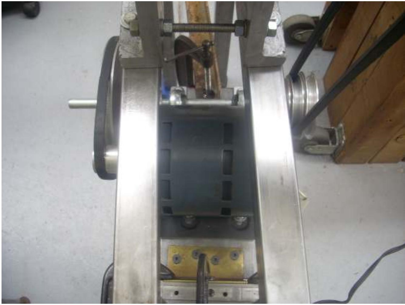
The view from the top. In order to tension the belt on the left, I tighten the lower right mounting bolt on the motor base. On the far side is a screw set in a block that pushes on the back left corner. The motor can then pivot and tighten the belt.
