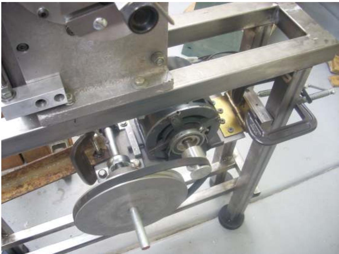
You can see that block and screw to the left of the motor. I wasn't thinking clearly about the forces in play so originally had two screws to push on the motor. That could only work if the motor was on a sliding track.
