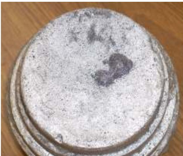
An essential first step in machining a casting, especially the sad looking ones that I make, is to figure out its initial shape. This means taking measurements so it becomes clear how best to cut your reference surfaces. In the case of a pulley, the reference is the centerline.
