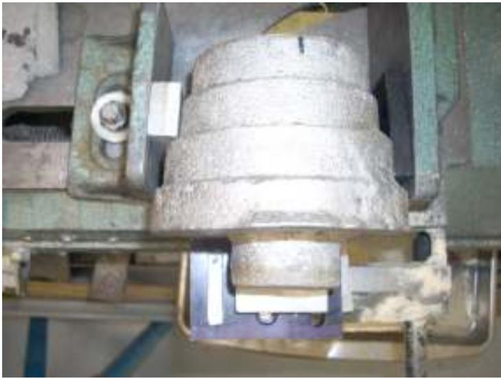
The casting has been securely clamped into my horizontal/vertical bandsaw. Note the packing in mostly blue under the sprue. Without this packing the casting would soon pivot, pinch the blade, and the blade would either pop off of the drive wheel or snap. A bit more time now avoids that excitement.
