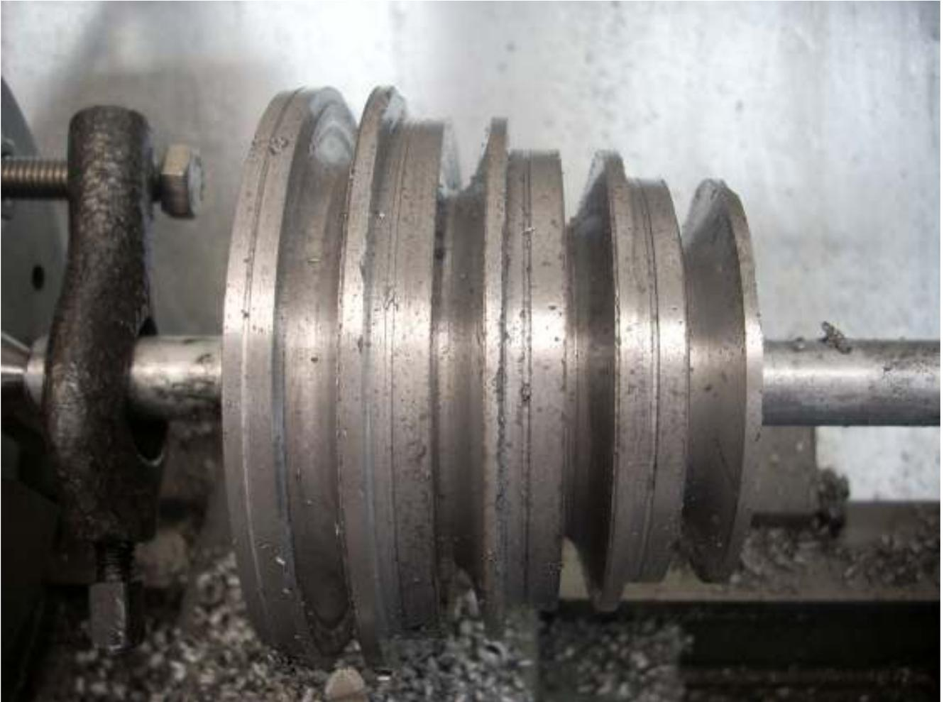
The compound was set to 17 degrees. I initially mounted a round nose cutter at this same angle. This worked OK but I later realized that the cutter is best set perpendicular to the mandrel or even pointing towards the surface being cut if there is no interference with the opposite face of the groove. Here you see the right face of each groove done. I eyeballed its placement. The left face will be set, as per the plans, to the width of 0.494".
