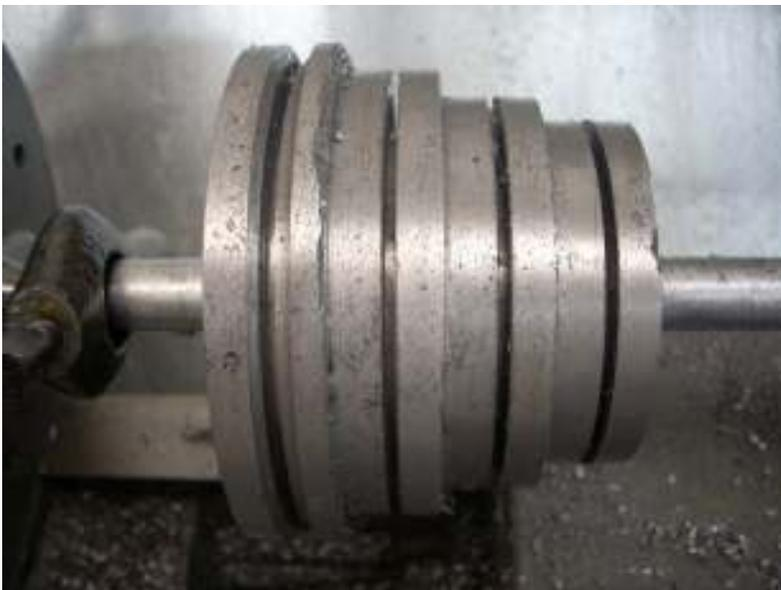
I've skipped a few steps. You see here that all four steps have been finished to their final diameter and the narrow end faced off. I measured the over all length of the part and calculated the center line of each groove. My cut off tool was then used at each centerline to cut down to the bottom of each groove. A second pulley will be made later and it will match this spacing of grooves.
