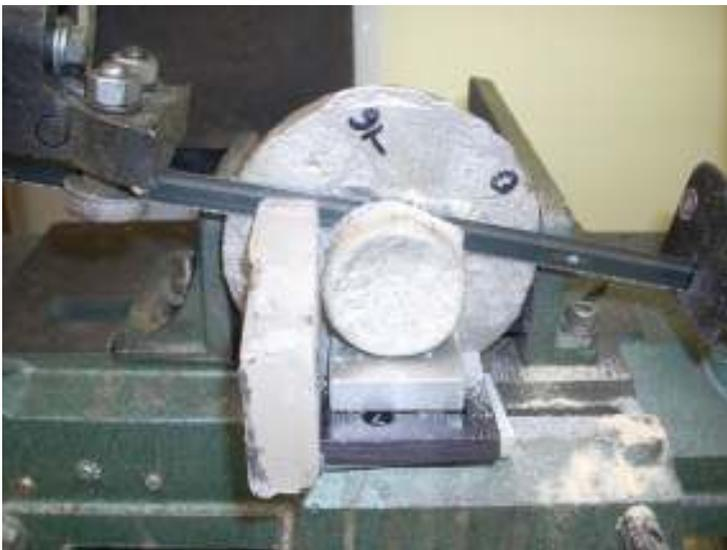
The saw is now starting to cut through the sprue. Note the white block of paraffin wax to the left of the sprue. It is just resting there and is being cut by the blade at the same time. This is a clean and easy way to lubricate the blade. The bits of cut metal coated with wax fall out the other side. The blade does not pick up any wax.
