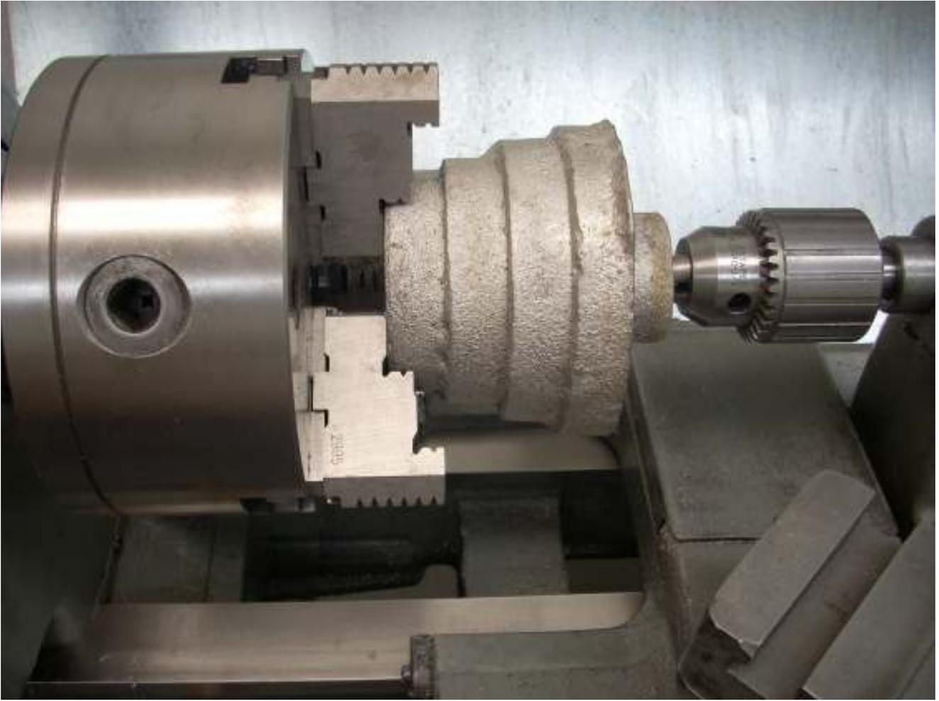
Being careful to avoid the lump on the small end's surface, I am bedding the casting into my 3 jaw chuck. My drill chuck is applying light pressure as I tighten the jaws. Careful inspection of the contact between jaws and casting insures the part is properly bedded.
