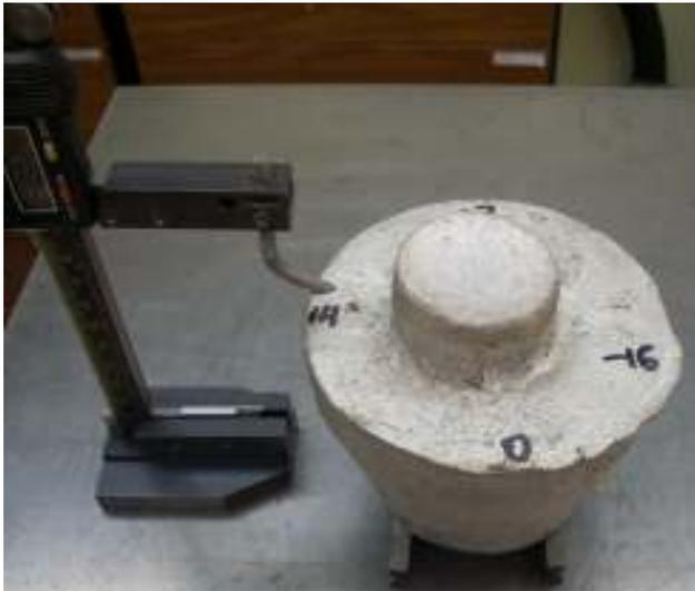
Much to my surprise and delight, the wide face was high at one side by only 0.014" and low on the opposite side by 0.016". This can easily be removed without seriously effecting the width of each step.
