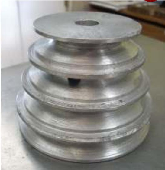
In hindsight, it would have been easier to first plunge cut the full width of the bottom of each groove. This would provide the maximum space for the cutter to form the sides of the groove. A second realization was that my cutter for the sides of the groove had a small chip in it. This caused the finished surface to be rough. The cutter was resharpened on my belt sander and then finished with a stone. It now cuts a nice smooth finish when WD-40 is applied as a cutting fluid.
