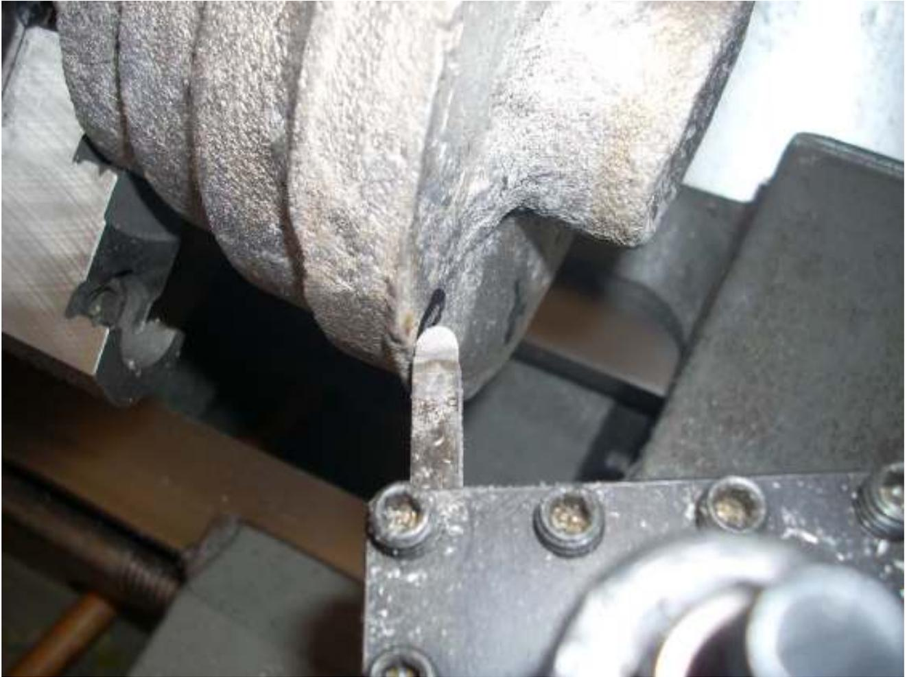
No, I'm not taking a cut, just using my cutter to verify the casting is bedded. By slowly turning the chuck by hand, I can see the gap between cutter and wide face vary. It looks good.
