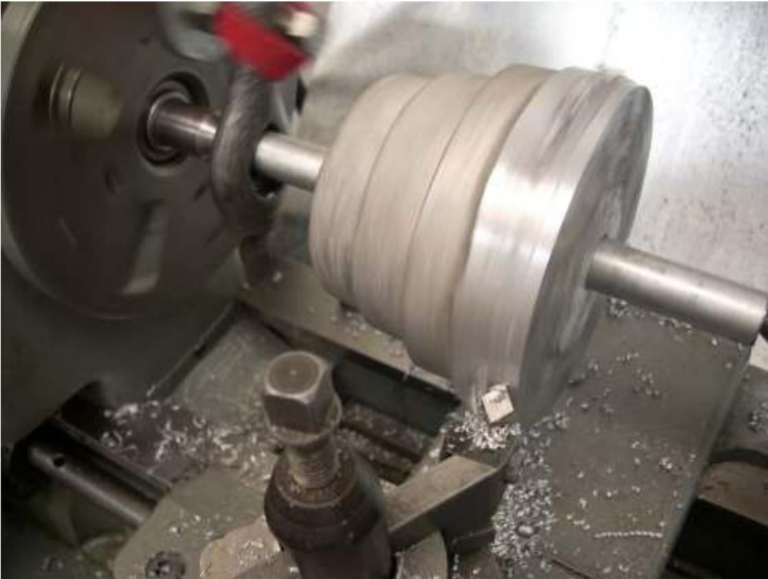
Initially I used a generic cutting fluid from Enco which worked OK but WD-40 gave better results so the remaining work was with it.
