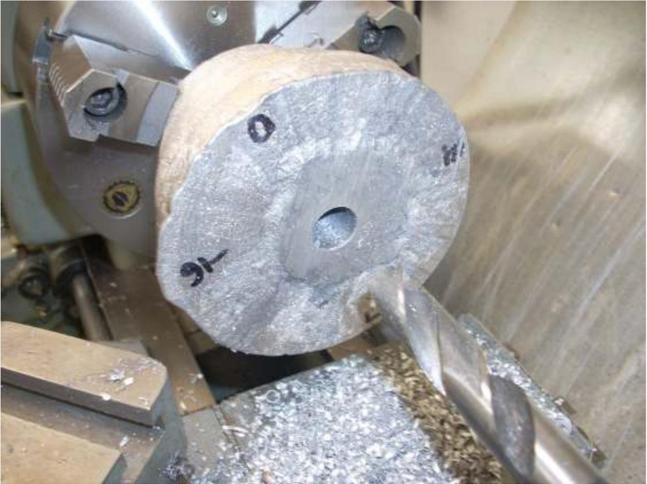
Step drilling minimizes the force on the chuck to avoid any “excitement”. Given enough twisting force from a large drill being used to hog out the hole, the casting can fly off.
