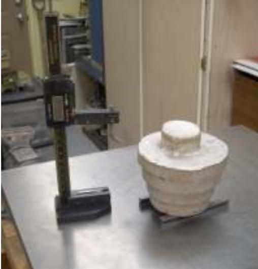
I don't want that lump in my way so have put the casting on small parallels which rest on my surface plate. I then used my surface gage to see how true the wide end is with respect to the narrow end. The more I must remove from the ends, the less thickness I'll have for the individual steps of the pulley.
