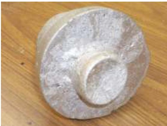
The wide end of the casting has the sprue attached. It does not look like a normal sprue because I almost ran out of aluminum during the pour. The lack of a longer sprue means that the molten metal's pressure is less so the surface is not as smooth. No matter, I am going to cut all of the surface away. Note how the sprue is concave. This is due to shrinkage as the metal changed from liquid to solid. Fortunately, only the sprue shrunk and not any of the casting.
