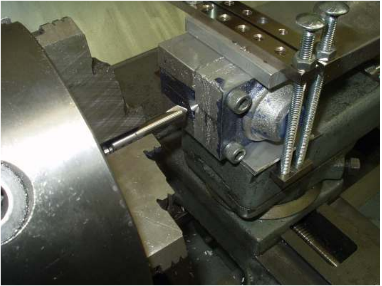
The center drill went into the 3 jaw chuck first.
