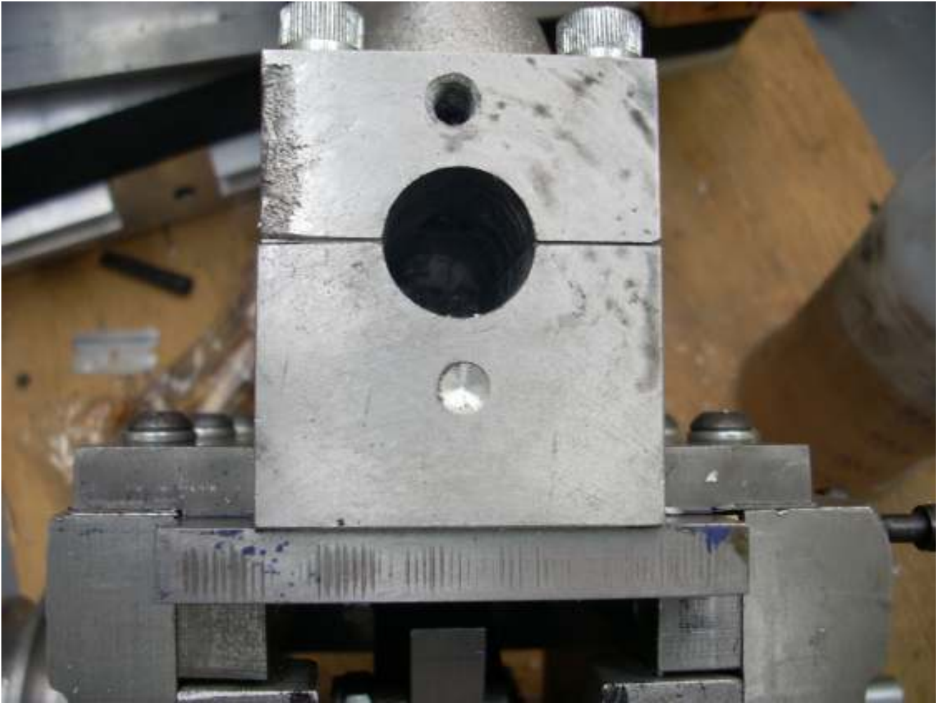
You can see the cone left by the end of the clearance drill.
