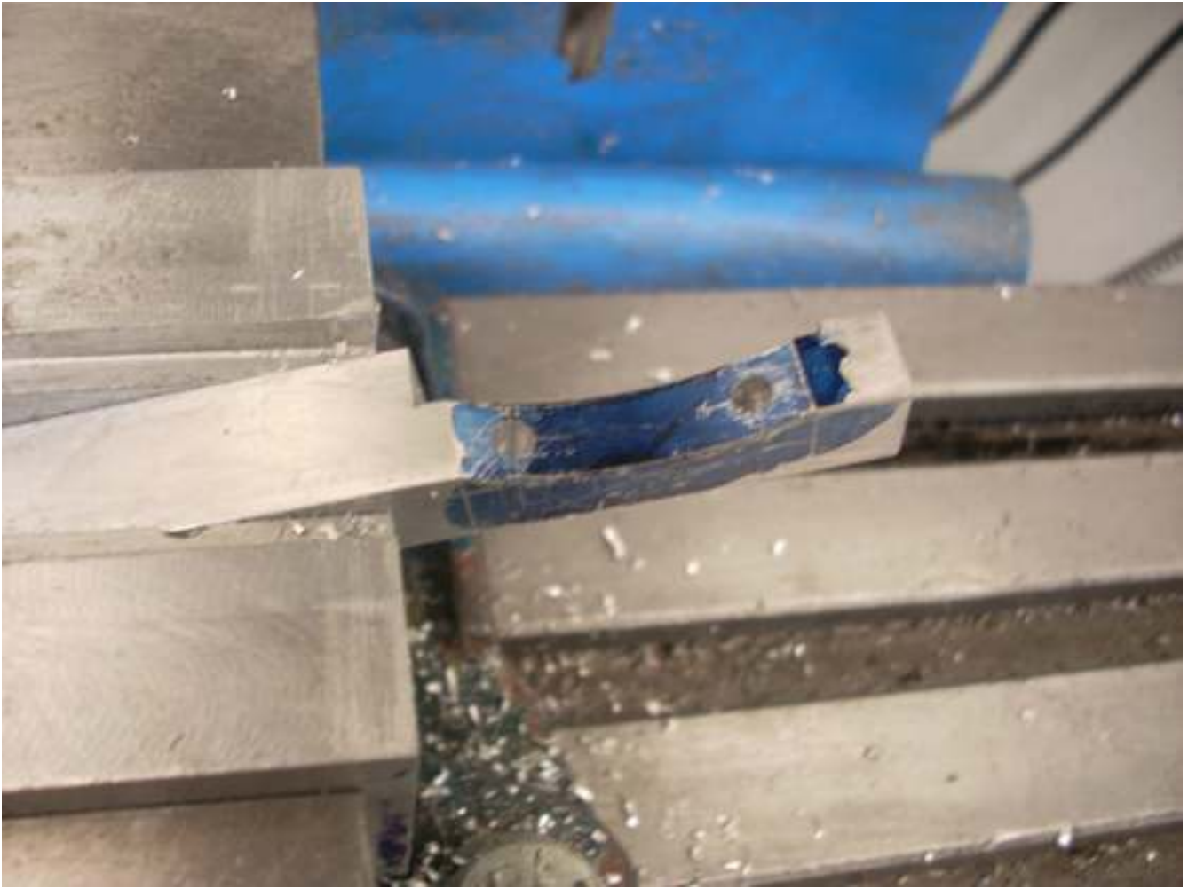
I have now drilled both clearance holes.
