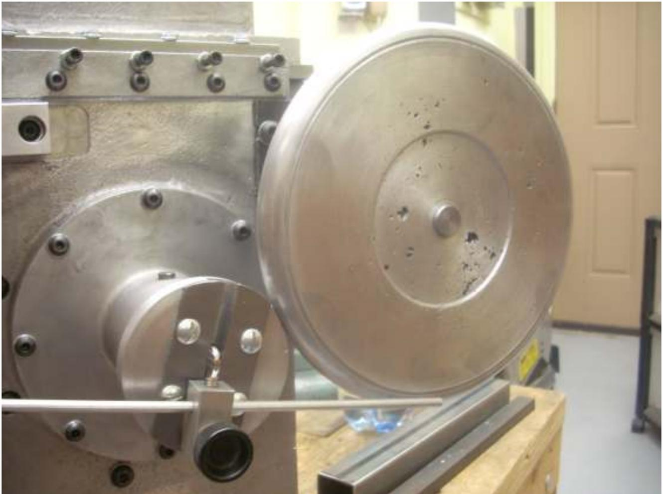
I have temporarily mounted the finished handwheel on the right side of the machine but this is not a good place for it. A finger can easily get caught between this spinning handwheel and the
