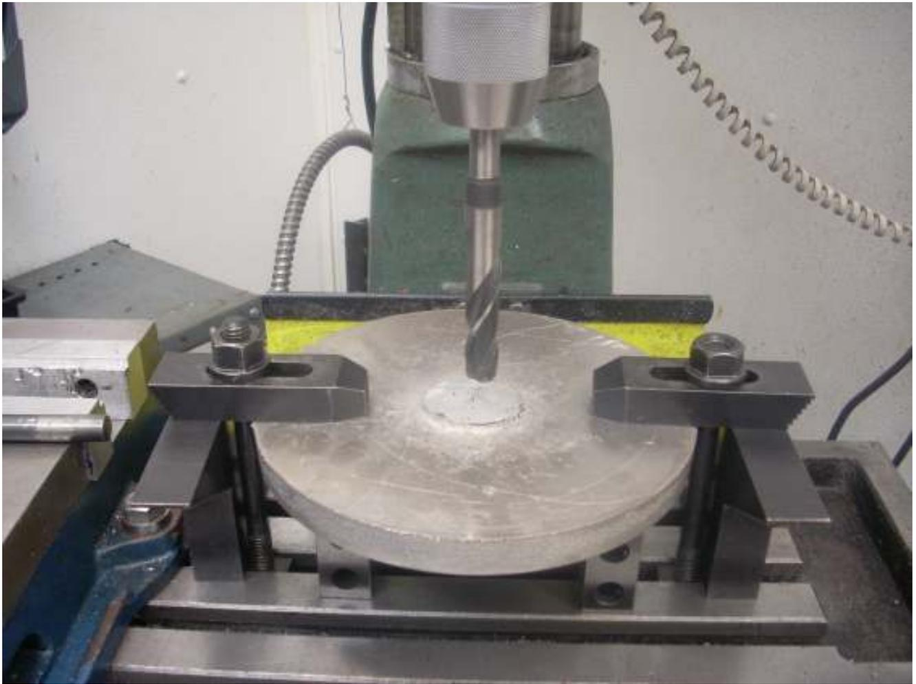
Last time I went for a bored hole that was a nice sliding fit on the mandrel. Not such a good idea since the mandrel distorted slightly and jammed in the hole. This time I'm simply step drilling with a  $\frac{1}{4}$ " ,  $\frac{1}{2}$ " , and finally a  $\frac{5}{8}$ " drill. Quick and a bit more room in the hole.
