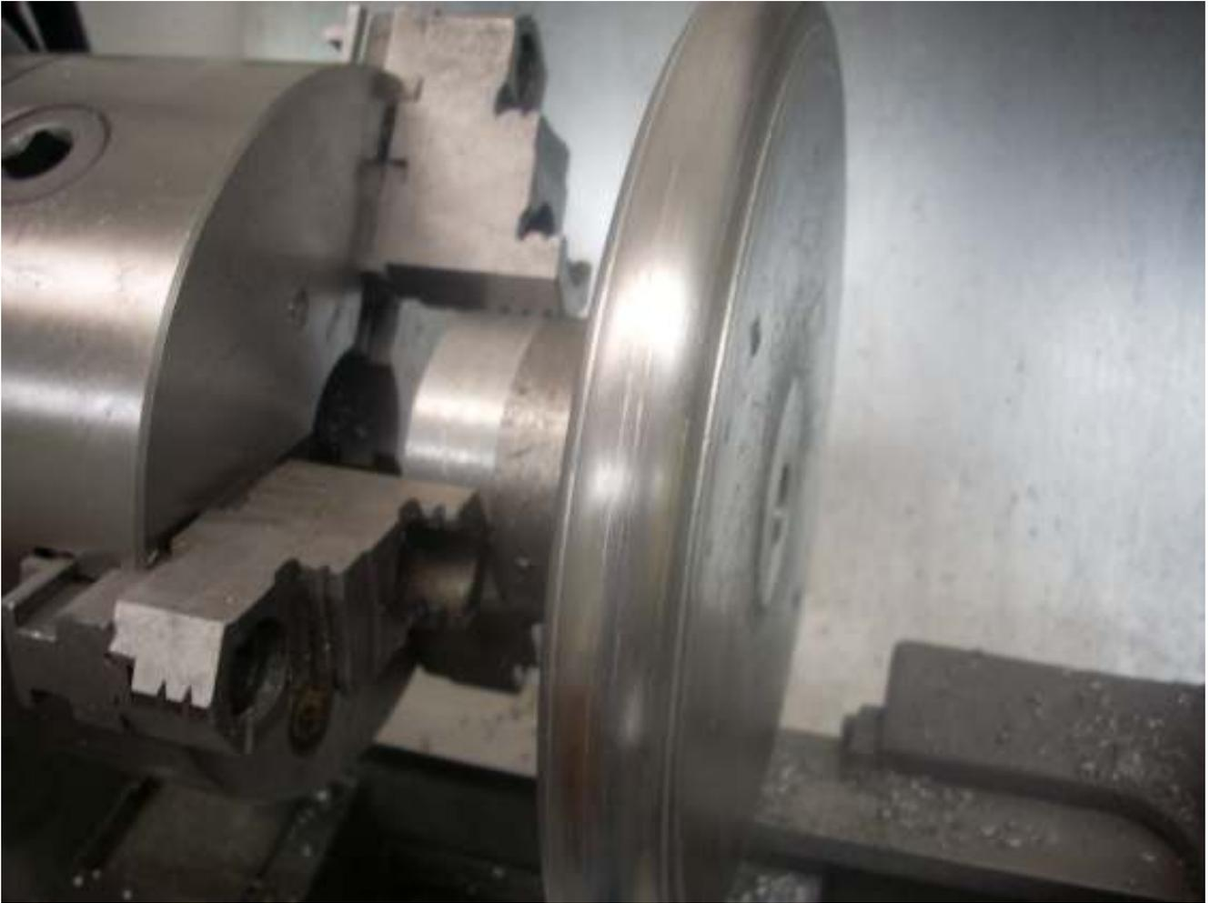
After rough cutting the right side, I moved the cutter over and cut the left side. Here you see the perimeter cleaned up with a file. That groove on the left is where I got confused and turned the dial the wrong way. Such is life.
