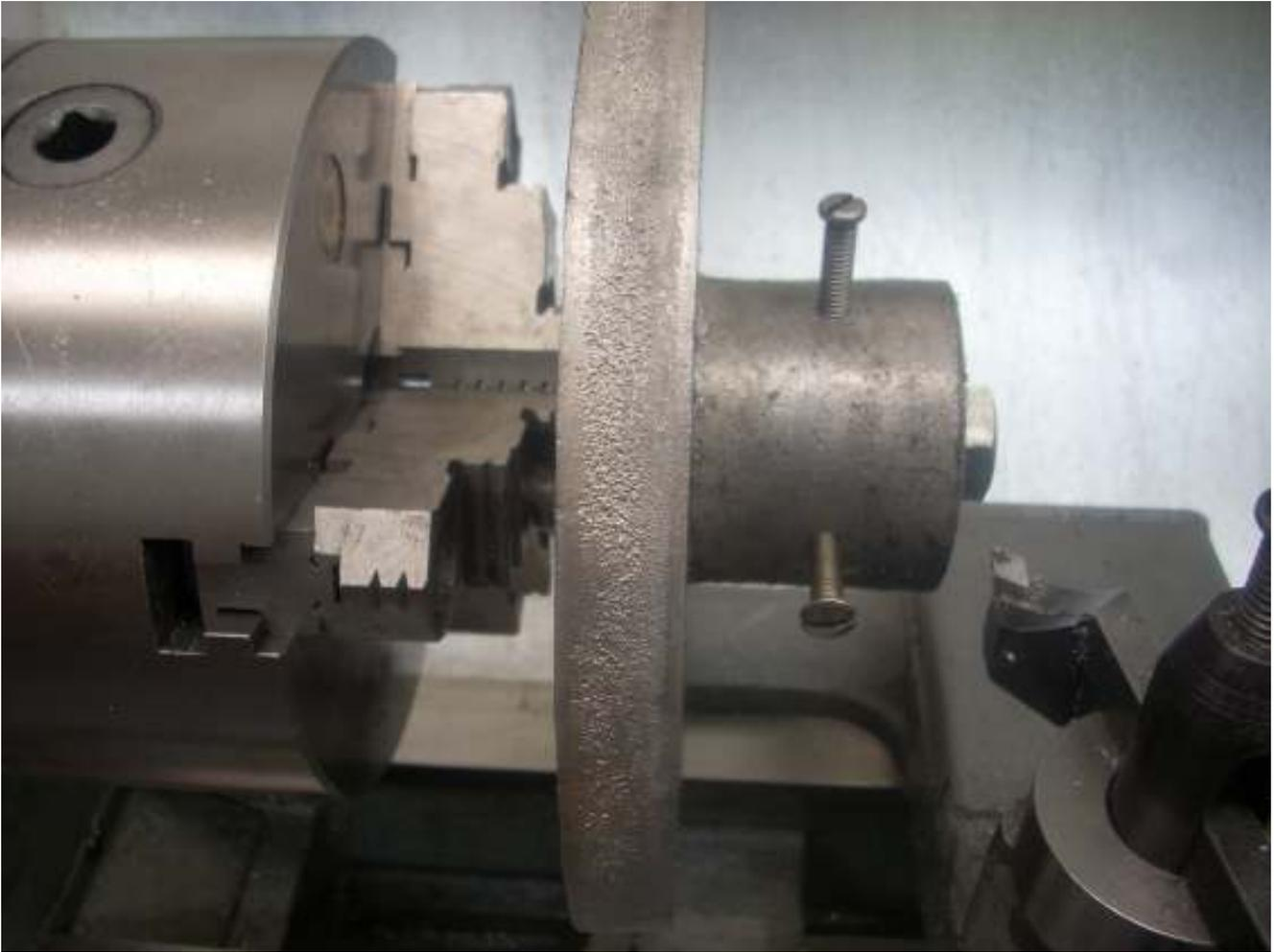
This time I'm using a mandrel secured by screws but will only face the end of the hub and turn the perimeter of part of the hub true. I would have cut more of the hub but my  $\frac{1}{4}$ -20 grub screws have not arrived from Enco yet. Those bolts sticking out are not "cutter friendly". In fact, they aren't knuckle friendly either.
