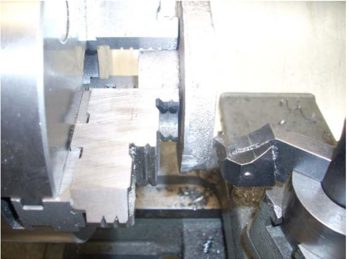
Next it was time to assess how best to machine the casting. Somewhere inside this rough casting is a perfect feed crank. The trick is to find it.
