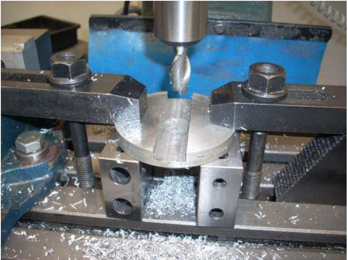
The next step was to machine the 3/4" slot. This is an easy task on a mill/drill. Since Gingery just used the cast in slot, I figure this is not a critical machining task. I just eyeballed it.
