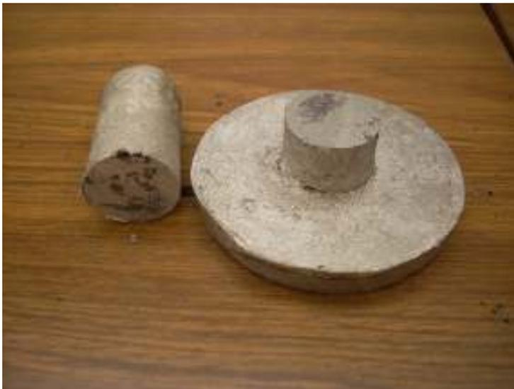
The sprue was sawed off at about  $3/4$ ". That leaves plenty of room for a finished length of  $1/2$ ".
