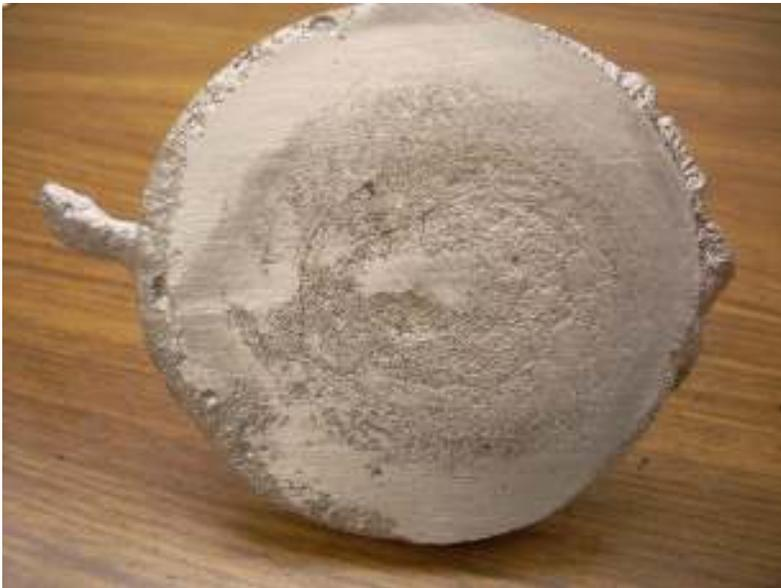
The casting came out usable. The center of the bottom was a little higher than around the end. This is probably because the melt dropped down the sprue and struck the sand at the bottom of the mold. That pushed down the sand resulting in a bulge in the casting.
