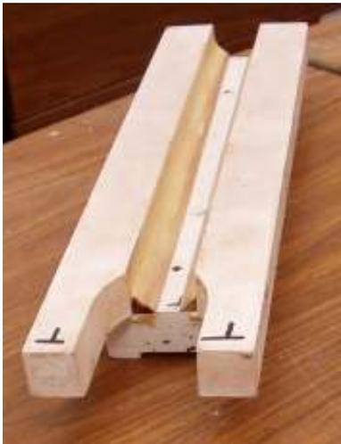
The problems started when it came to ramming up this pattern. I used the same flask as used for the side column plates. Two bars were placed across the cope to hold gagers and I rammed the cope very hard. No joy. The cope dropped out soon after I cut the sprue. Fortunately the drag was spared.
