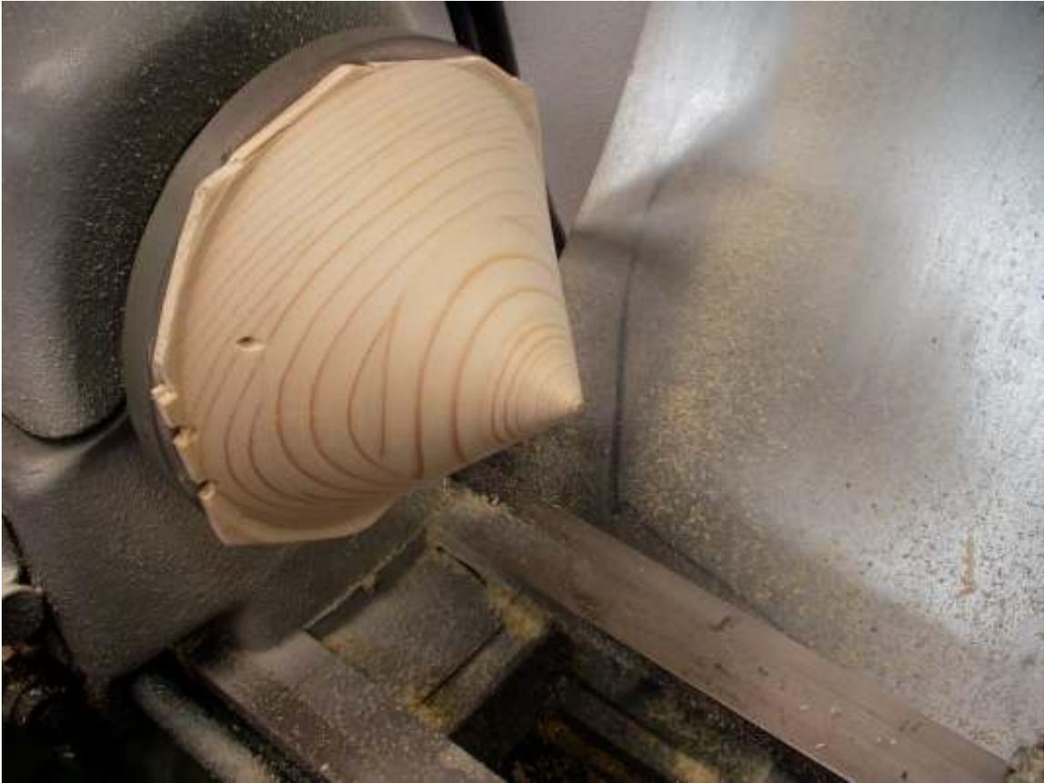
It made a mess of my lathe and shop, but I turned a very nice looking cone. The hole in the side of the cone is from pilot holes for wood screws that hold the wood to the faceplate.
