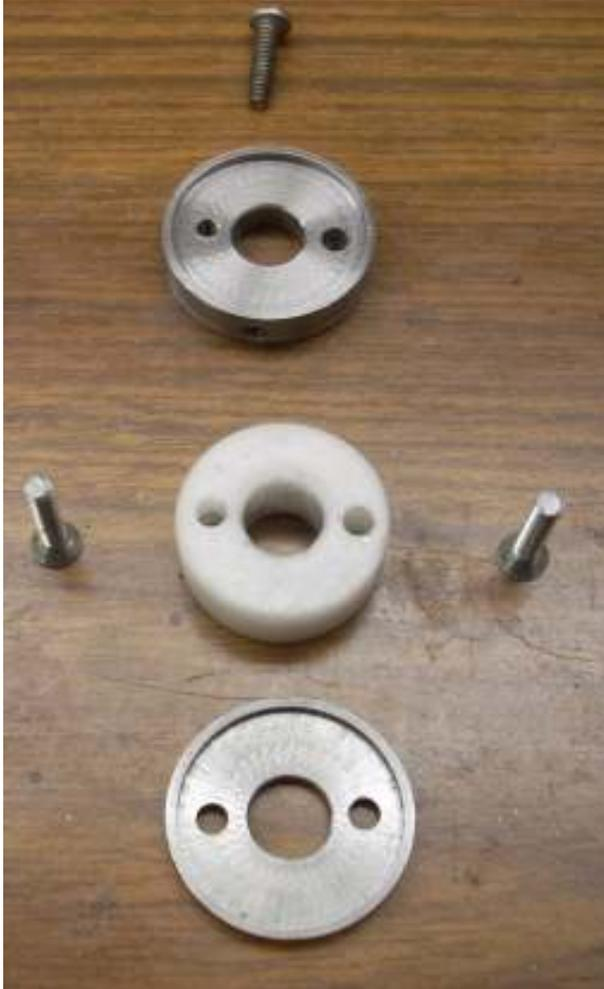
Nothing special about the lathe work. The top and bottom are CRS. The recesses are 0.05" deep and cut with a boring bar. The plastic is Delron®. The plastic scale is 0.005" thick so there
