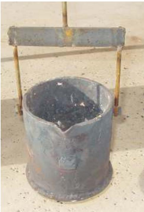
To lift the crucible from the furnace, I use a double hook lifting bar.
