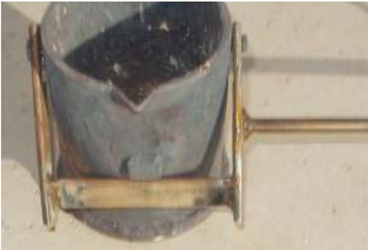
You can see how the handle engages the lifting bolts and the chock. For any reasonable position of the crucible, the handle is locked securely to the crucible.
