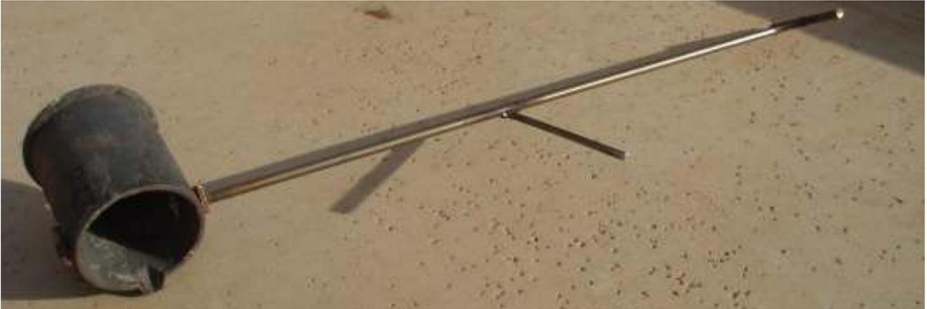
During the pour, my left hand is rotating the perpendicular bar while my right hand is holding the handle closer to the crucible.
