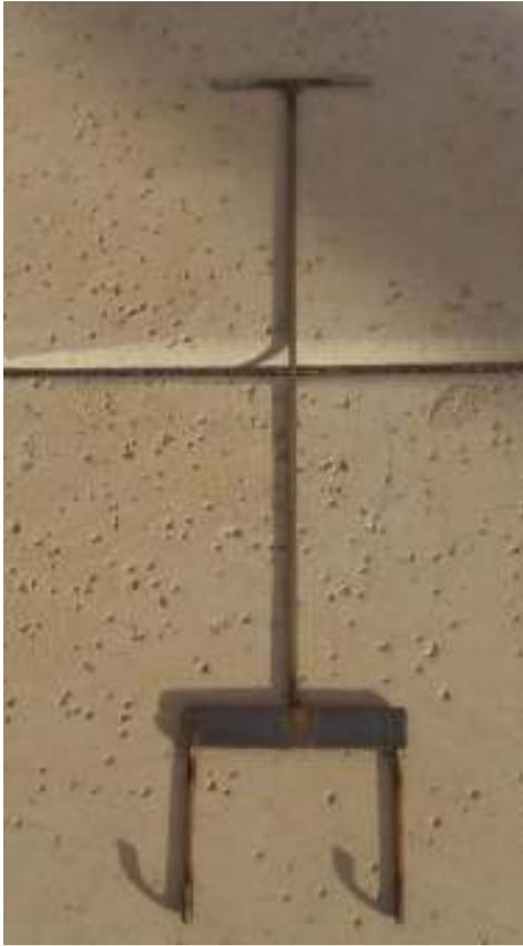
Shadows at the bottom of the picture are a bit confusing but you can see that the top of my lifting bar has a T handle. I used  $\frac{1}{4}$ " CRS rod for most of it and the cross piece is  $\frac{3}{16}$ " x 1" x 6" CRS.
