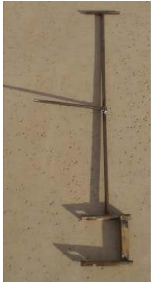
When this bar is fitted to the crucible and both are cold, it is a tight fit. However, when the crucible is hot, I get a loose fit. I had to do some quick adjustments the first time I tried to use this handle. The crucible's diameter increases about  $\frac{1}{16}$ " when at  $1450^{\circ}$  F.
