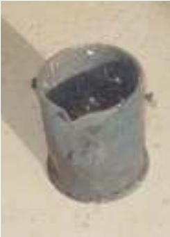
My crucible is made from 6" pipe with a  $\frac{1}{4}$ " thick wall. The bottom is  $\frac{1}{4}$ " plate. I can safely pour 9 pounds of aluminum in there and have  $1\frac{1}{2}$ " from the surface of the melt to the lip.
