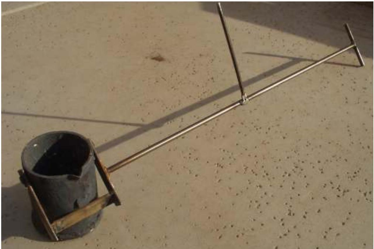
Here you can see the “big” picture. I have used this handle over 10 times with a Visegrip® in place of the perpendicular bar and it worked fine. The last time I had my welder set up, I replaced the Visegrip with the perpendicular bar. I may need to shorten this bar a little as it may interfere with the action of hooking onto the lifting bolts.
