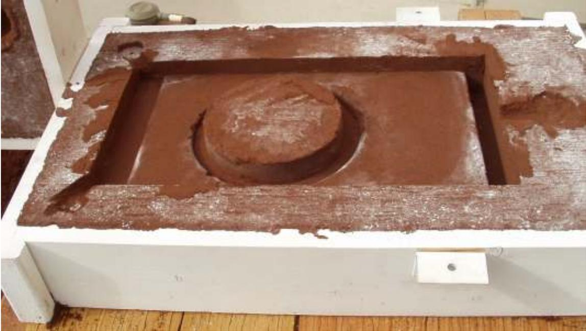
Here you can see the sprue on the right cut into the heaviest part of the pattern void. On the left are my two risers. When metal shows up in these riser holes, I know my void is full. The sprue and riser forms were not pulled out at this time.
