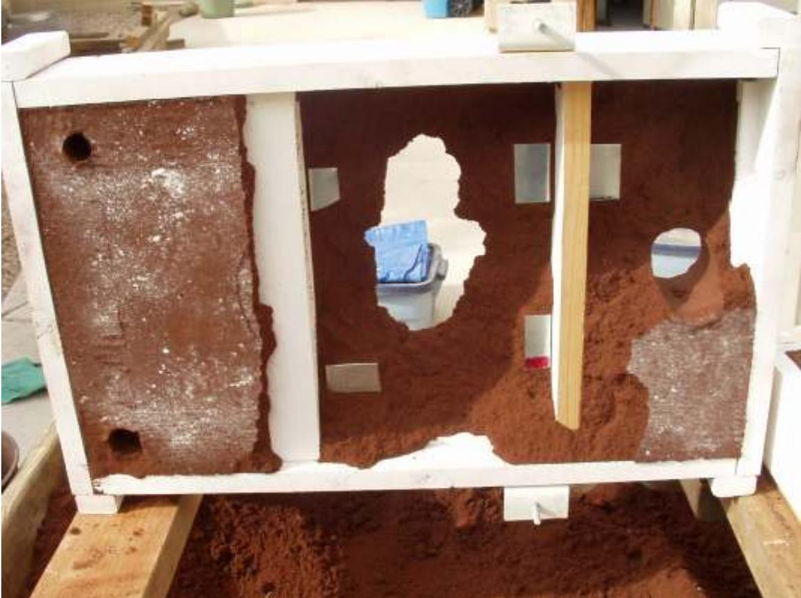
Not a big set back. I just cleaned out the sand, put the cope back on the drag, dusted, and began ramming again. This time I paid more attention to ramming each corner and using more force. It paid off as there were no more dropouts during the day.
