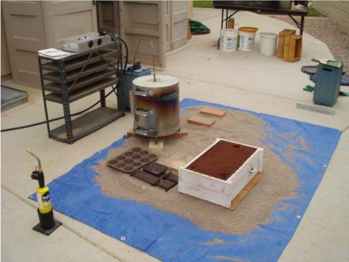
The flask is ready for pouring. I have about 75 pounds of sand in that flask. It was not easy to carry from my sandbox seen in the background to the casting area. It was murder gently lowering it down to the ground. My back is a bit tender now. *Next time* I will ram flasks this size on my wagon and then wheel them over. I will still have to flip the drag over but that is not nearly as bad.
