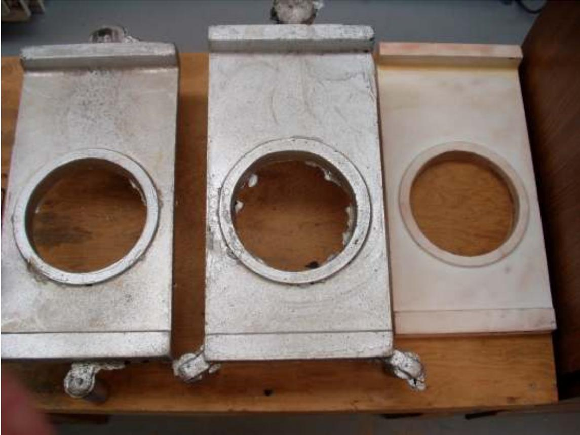
These are the faces that everyone will see. The center casting has some damage near the hole. It is ugly but will not effect the part's strength. A bit of Bondo and paint can cover this sin. At this time, I'm not interested in casting another side plate.
