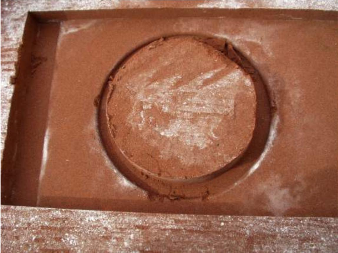
With the pattern drawn, you can see some damage to the edge around the hole. I did not ram hard enough. On my second casting with this pattern I rammed much harder. I used my narrowest tool and worked the sand into the pattern at a 45-degree angle. It greatly reduced this problem.
