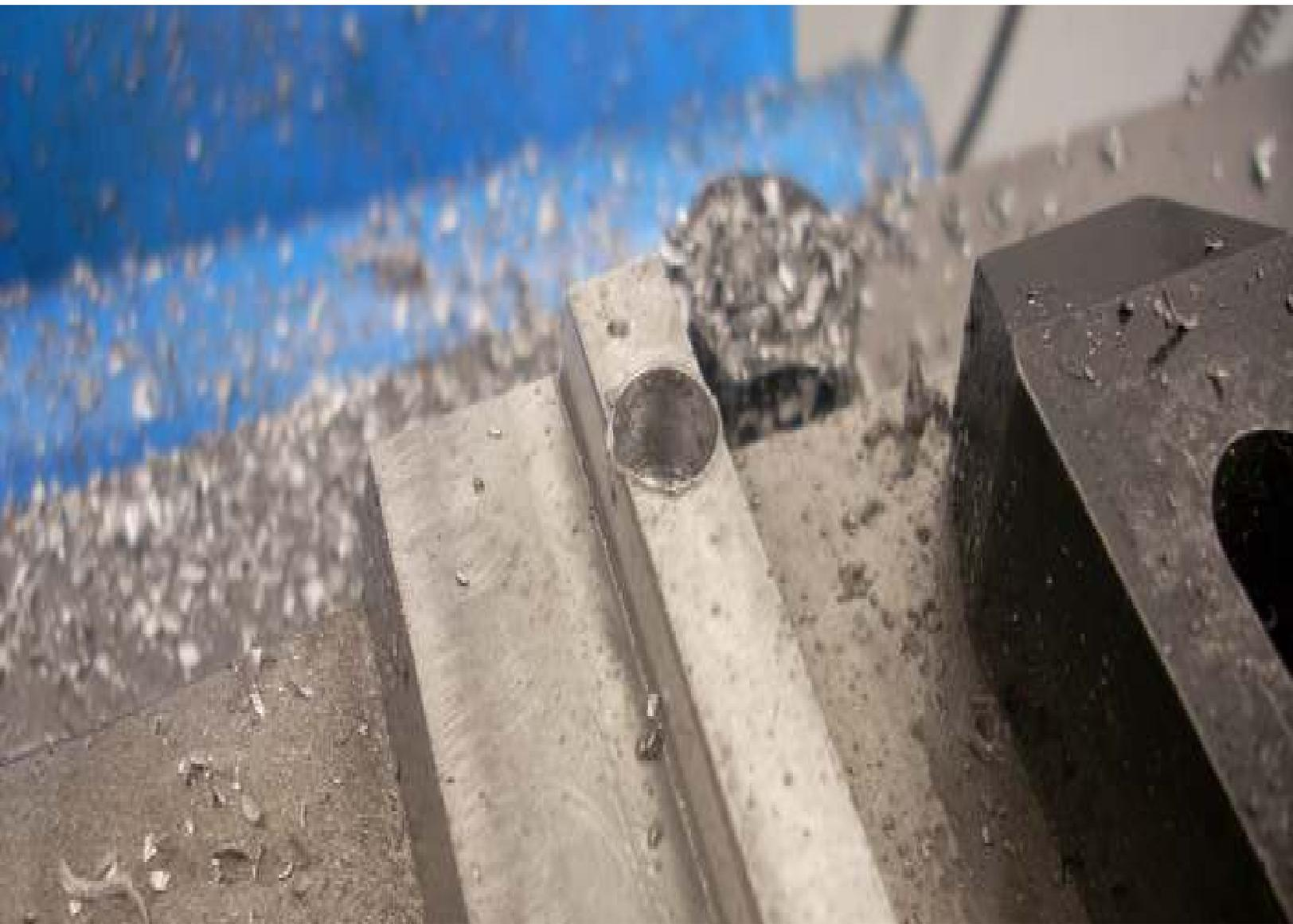
I knew that the narrow pad would be trouble even with 0.02" of metal between hole and outer face. After drilling the tap hole, I went back and used a clearance drill for the first 1/4" in hopes of not having the tap blow the sides of the hole out. It did help but still bulged the side out. On the next hole I used a drill one letter smaller than the clearance hole and that helped. A few passes with a file removed the bulged areas.
