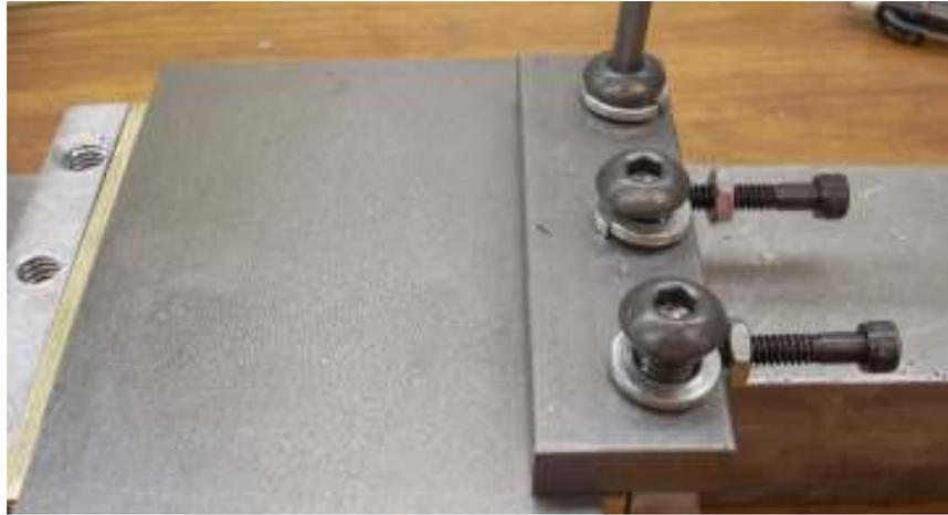
I had room for a brass gib on both the left and right edges. The left gib is held in place with Locktite<sup>®</sup>. The right gib has two shallow holes drilled in it to accept the gib screws.
