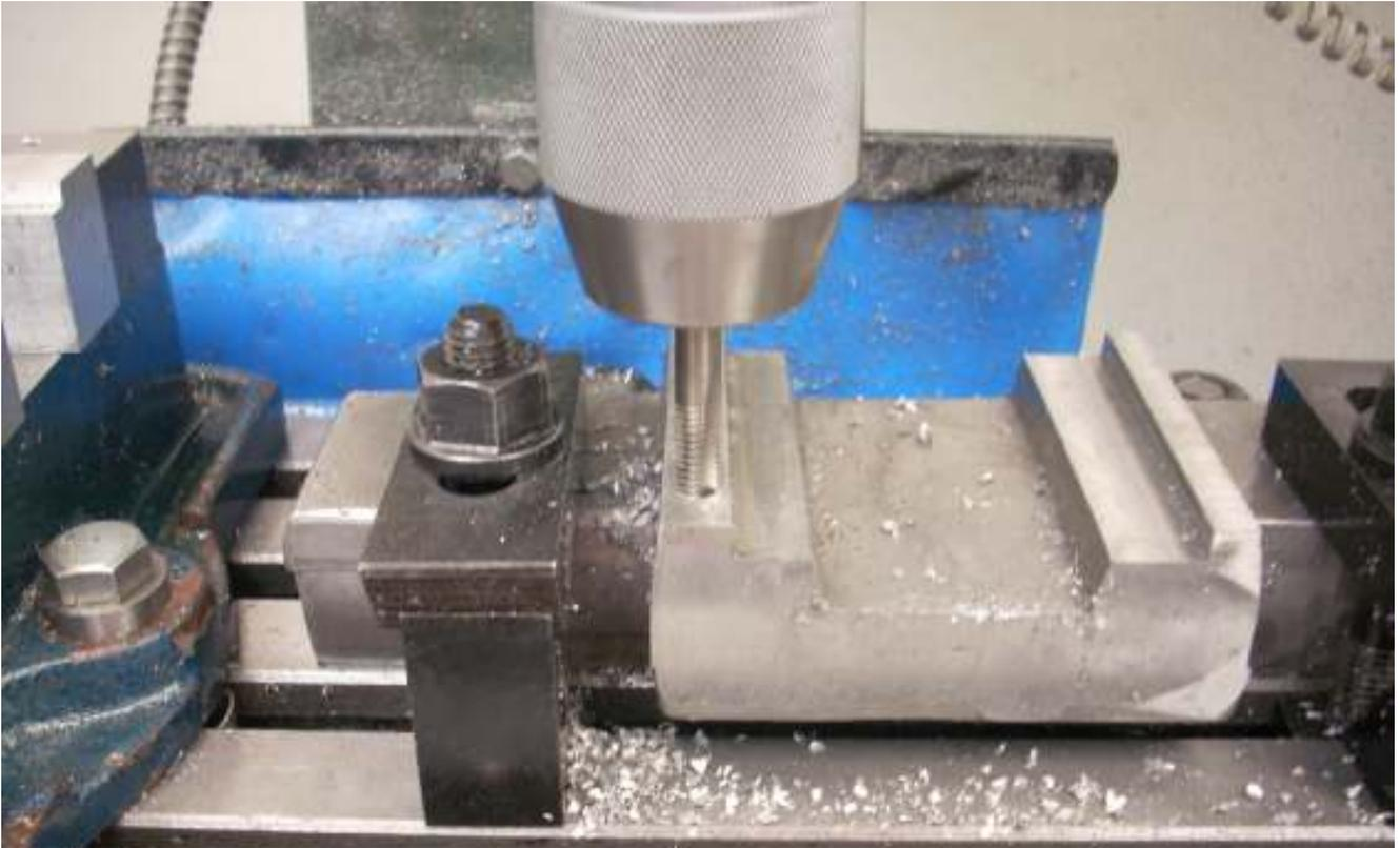
I used my DRO to find the center of the left pad. With my clearance drill mounted in my drill chuck, I used one of the clamps as a guide to set my Y location. I want the clamp to be close to true but most important is that all 3 screws cleanly fit through the clamp and into the casting. After center drilling, I drilled the tap hole to a depth of 1.5". I then used a spiral tap to go in 1". This leaves me 0.5" to hold the swarf since spiral taps push the swarf ahead.
