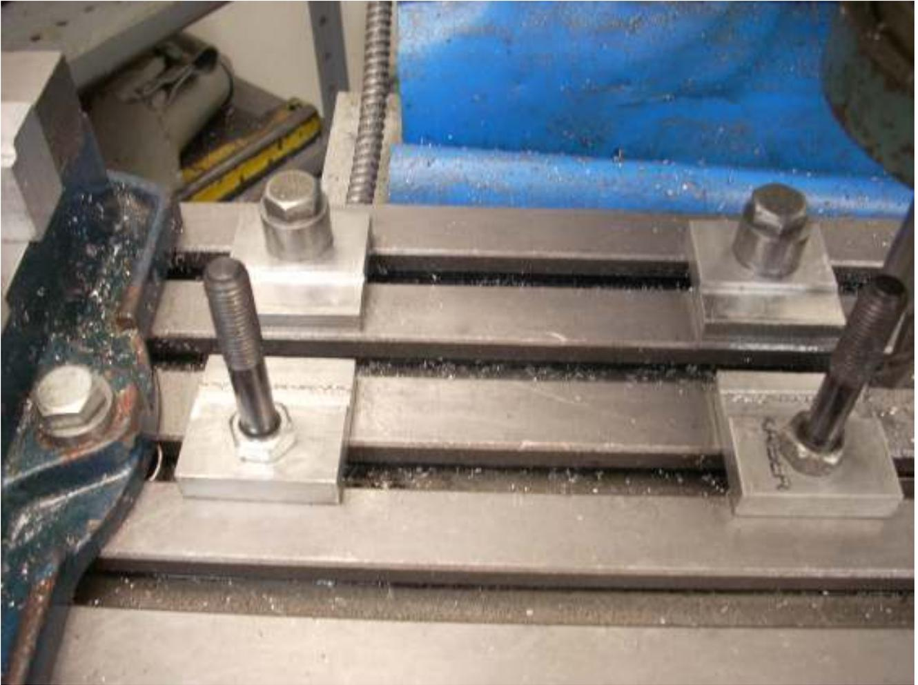
The accuracy of the shaper will depend on having a cross slide that is true. The best way to do this is to machine supports in place, clamp down the casting, and then verify all is bedded right with a DTI.
