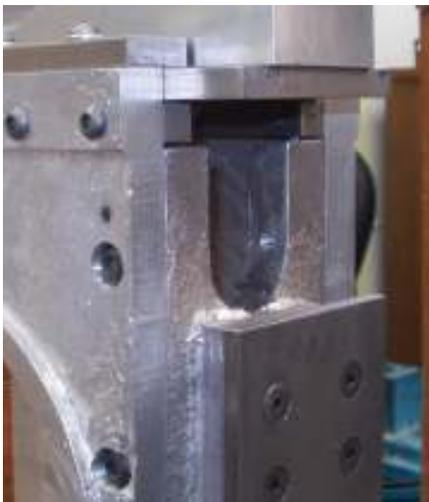
The clamps are holding a piece of scrap  $\frac{1}{4}$ " x 3" CRS plate that was left over from the part screwed onto the front of the shaper column. When assembled, the vertical slide will engage this plate.
