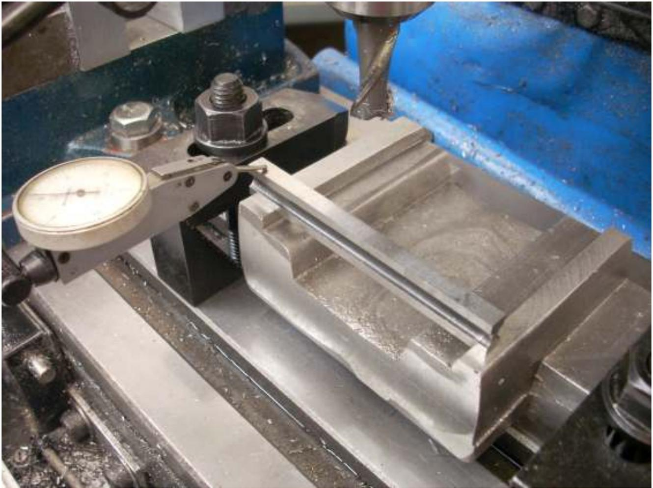
To verify that primary reference 1 is in contact with the table, I want to check from side to side and from front to back on secondary reference 2. The bump I get from falling off of one top surface can cause error in my DTI reading so I prefer to take a known good parallel and place it on both horizontal faces. Then I can run the DTI all the way across without any bumps. It read all zero. I moved the parallel to the back and read zero all the way across there too.
