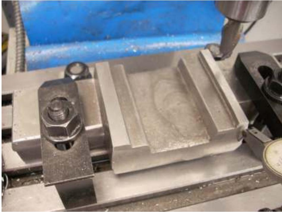
Next came a careful cleaning of all surfaces both on the mill and on the casting. I pressed the casting both against the back supports and the table before tightening the clamps. There is a lot of contact area here so no need to crunch down hard. That will just distort the casting and could crack it.
