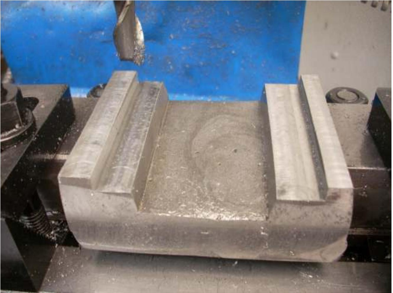
Milling the vertical slide went well. My main concern was that the right clamp support was close to  $5/16$ " wide rather than the  $1/2$ " specified by Gingery. This was due to excessive taper in the pattern. I had plenty of metal for the support pads so milled down the top faces until I had at least  $0.02$ " of metal around the sides of the holes. More on this later.
