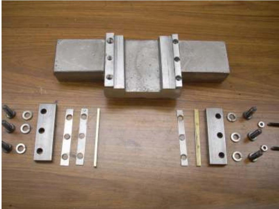
An exploded view is always fun to see. You can barely make out the ends of the gib screws on the right. The ends were pointed on my lathe. I still have some fine tuning to do with shims but that will wait until I fit the assembly to the shaper.
