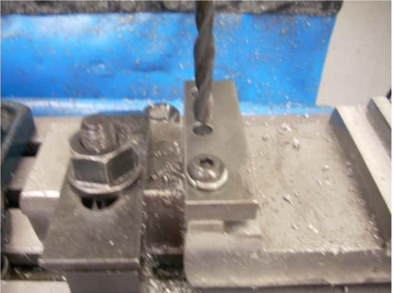
With the first screw in place and just snug, I use the clamp to locate the next hole using my clearance drill. I do not change the X axis position but rather swing the clamp and move the Y
