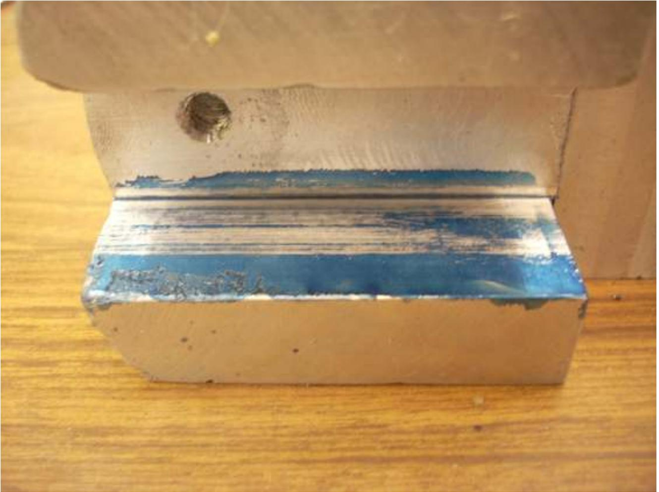
Using the bluing as a guide, I gently used a clean file to remove most of the bluing in the area I want to reduce. The process takes around 0.0005" of metal as it takes the bluing.
