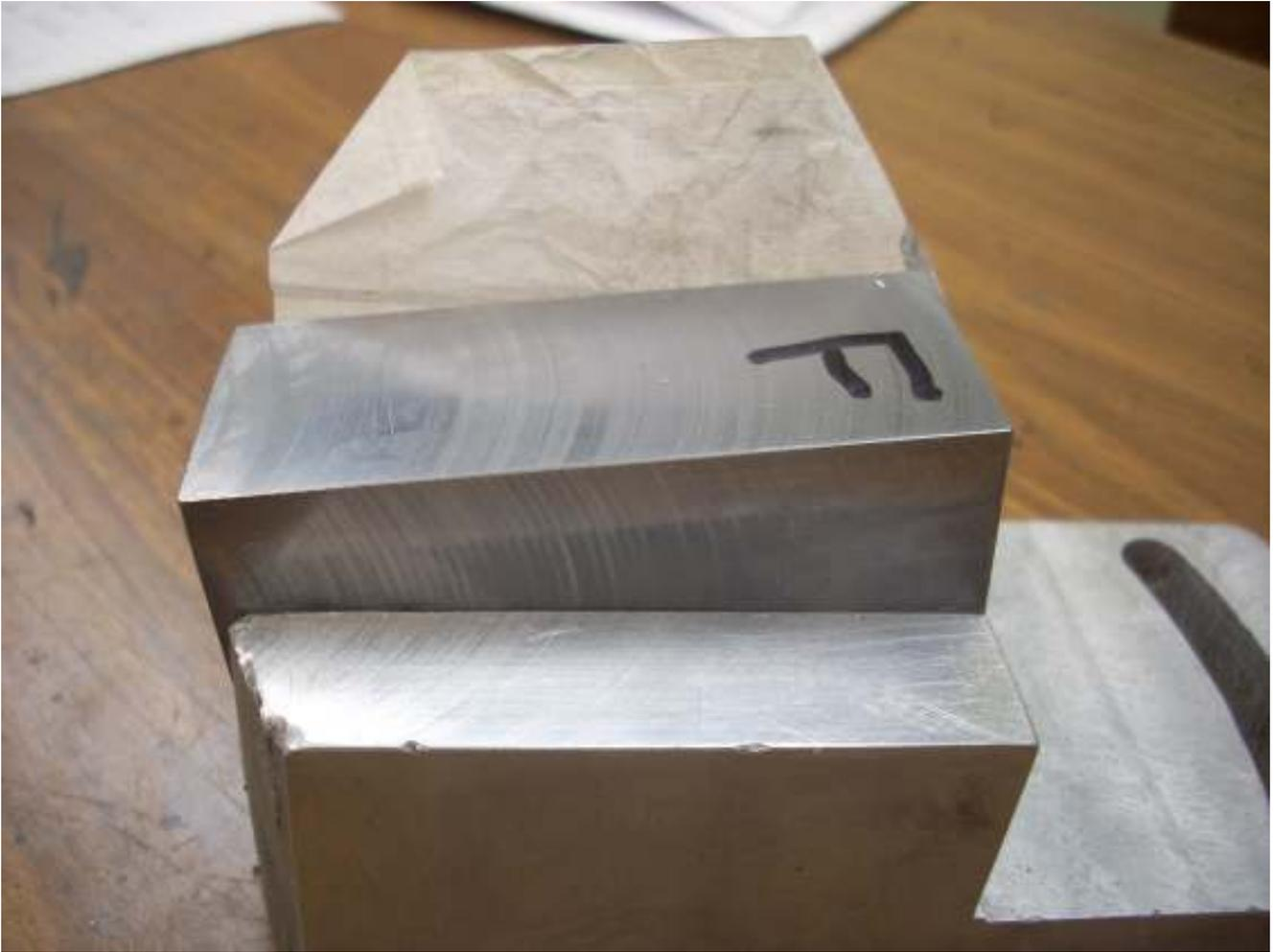
I took a piece of 0.001" cigarette paper and placed it between the clapper and the box. As expected, the clapper only went in about half way on the right. The fact that the clapper went into the box a bit more on the left says that that end is a little wider.
