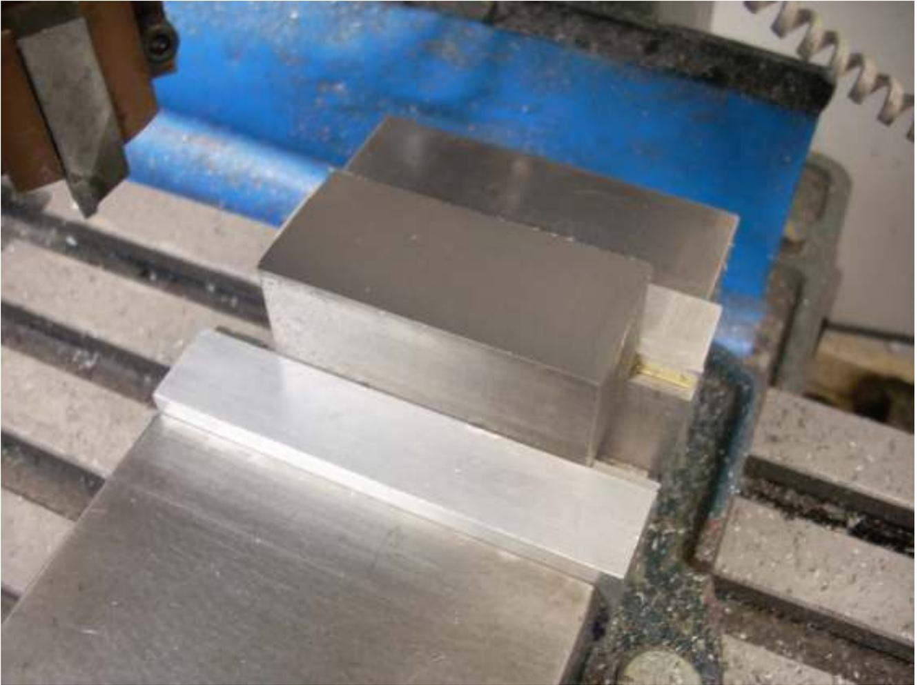
The block is now clamped and ready to be squared up. The top face is shell milled using plenty of cutting oil. The 12L14 contains lead which is a nice lubricant but I figure a little bit of oil can't hurt.
