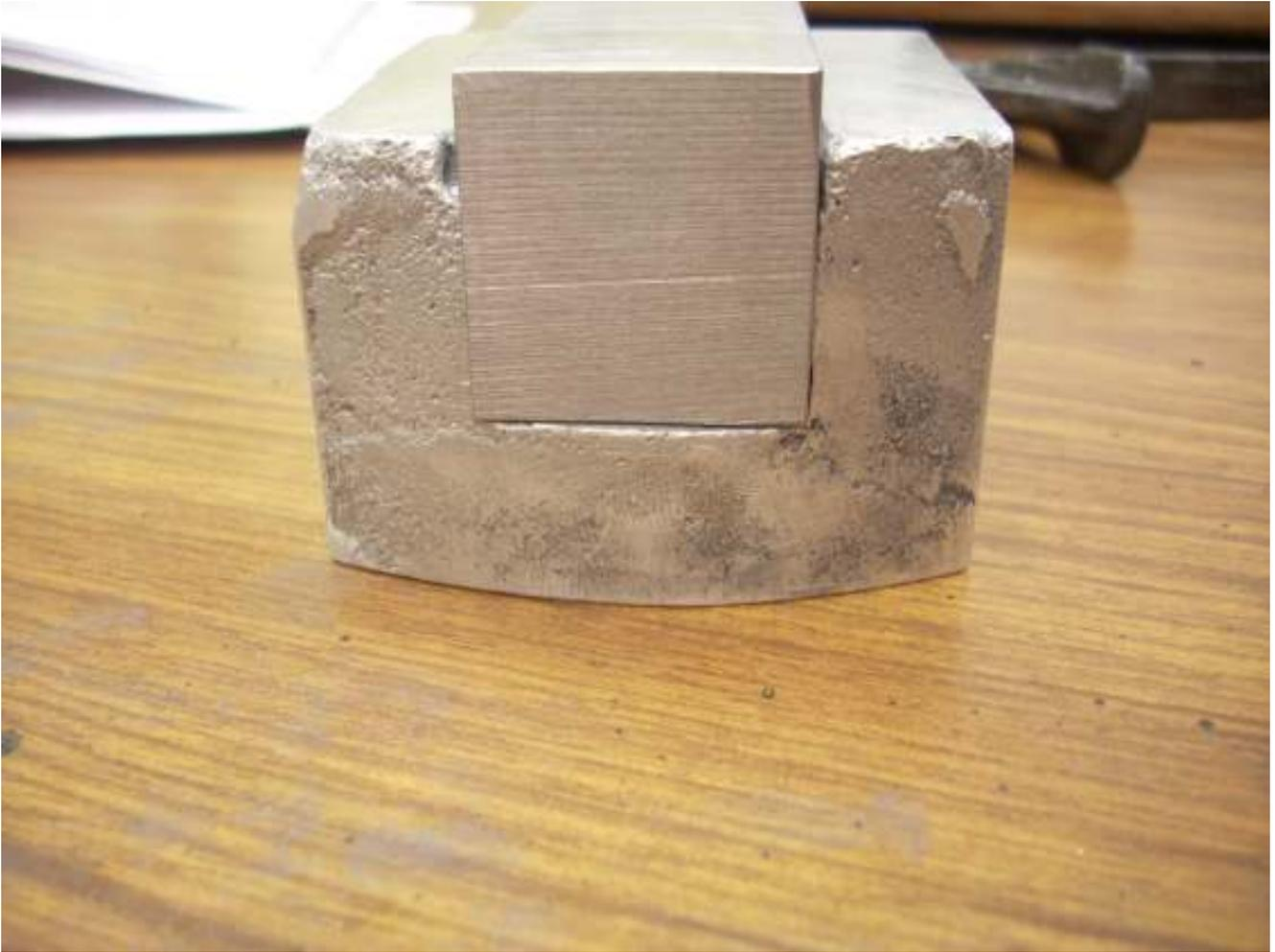
You may recall that before lapping the block went in half way. This tells me that the top half of the box is slightly wider than the block. The bottom half of the box is now a snug sliding fit to the box.
