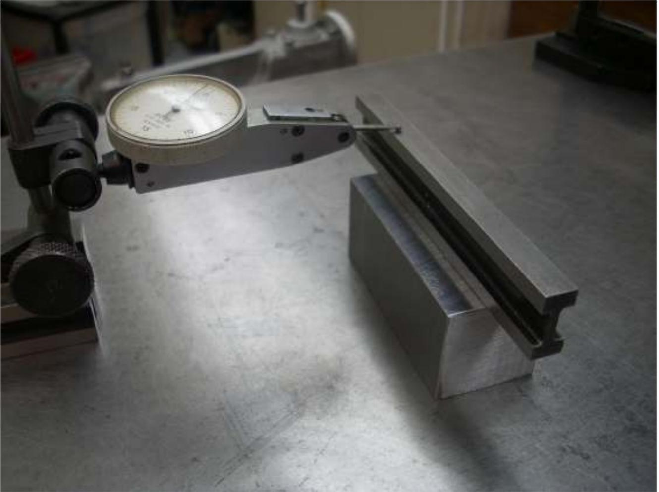
Next I wanted to verify that opposite faces are parallel. The DTI is run on the parallel so I don't get a bumpy ride on the relatively rough finish of the block. These sensitive DTIs sure do make me look bad. Anyway, I saw less than 0.0005" of variation from one end of the block to the other. The block was rotated 90° and the test repeated and passed.
