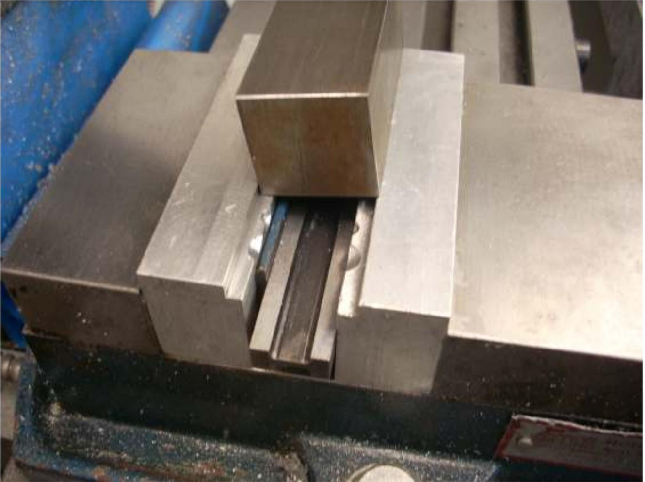
After sawing off a block of 12L14 steel, it was time to cut fresh surfaces on my soft jaws. The jaws are clamped to packing such that the jaws are about as far apart as they will be with the block in place. This step minimizes any error along the vise ways.
