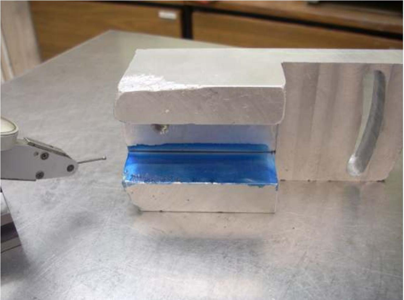
I use my DTI to find where metal must be removed. As expected, the bottom of the box is narrower than the top.
