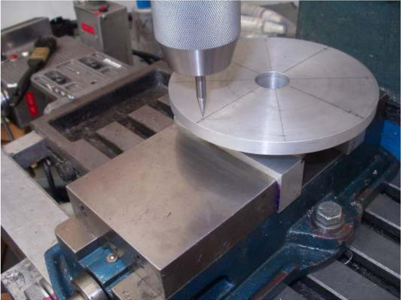
The flange was simply clamped into my mill vise. This is a first for me. I have never had a need to drill a bolt circle before. The job was made exceedingly easy because I own a Shumatech DRO. It has a bolt ring function built in. I simply had to tell it the radius of the ring, number of bolts, starting angle, and stopping angle. The starting and stopping angle are equal which means that I want the 8 bolt holes to cover a full 360 degrees.
