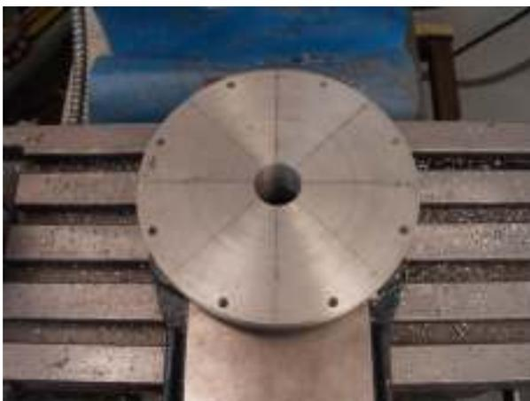
The holes were all drilled with a #7 so I could spot through to the bolt ring on the column.
