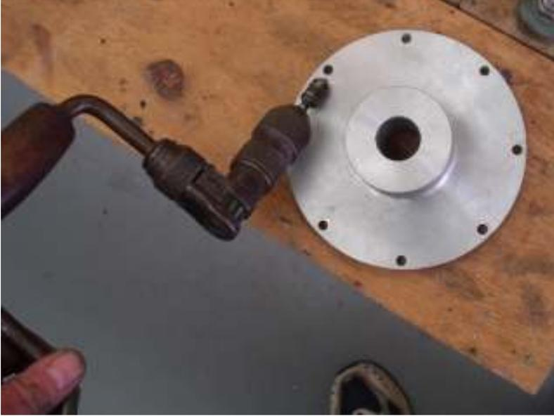
I used a countersink permanently fitted to an old brace and bit to clean up each hole top and bottom.
