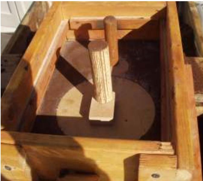
The sprue has been fitted to the gate. I added a block of wood between the disk and riser to provide more space to hold molten aluminum in hopes of preventing a shrink void. If you are familiar with the casting of this part, you may notice that I am not following Gingery's plan of placing the riser on the end of the hub. It seemed to be unnecessary effort to me. If my approach fails, I am out a bit of time. If it works, I have avoided hassle plus learned something new.
