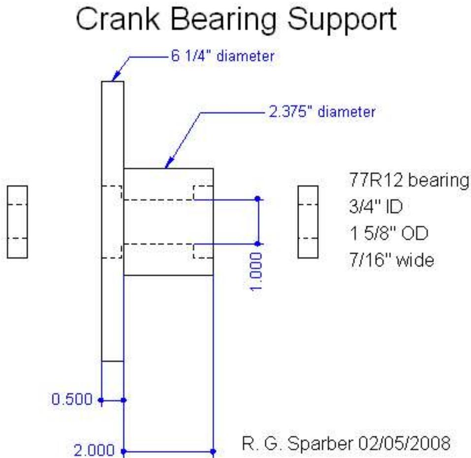
I had already made the pattern assuming ball bearings and decided to just use it. The result is that the hub is larger in diameter than required. So far I don't see any harm in that. The only deviation from the
