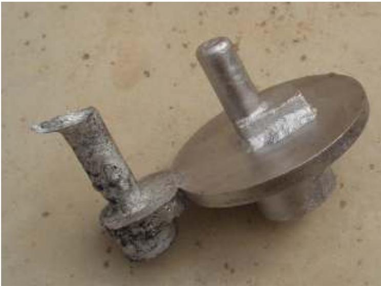
The sprue and riser are visible here. Note that the sprue has a slight taper on its body. This was formed with a tapered sprue cutting tool formed from 4 wires attached between two disks of different diameters. The top of the sprue has a larger angle taper which was cut after the body was cut.
