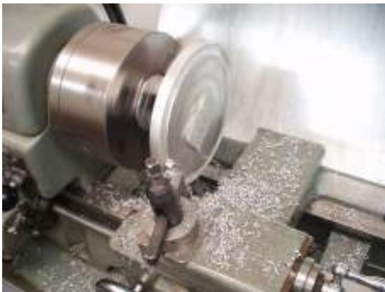
The part is held in a 3 jaw chuck and the edge cleaned up first. I then faced the plate removing the remnants of the riser. To my surprise, the plate was not all that flat. I ended up having to take about 0.04" from the face before it was true.
