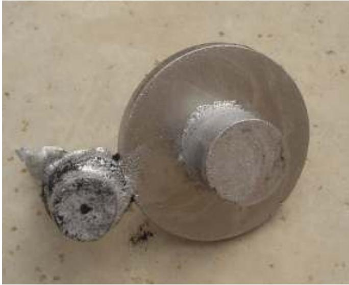
Well, I got away with it! No shrink voids at all. You can see the sprue still attached to the edge of the plate.
