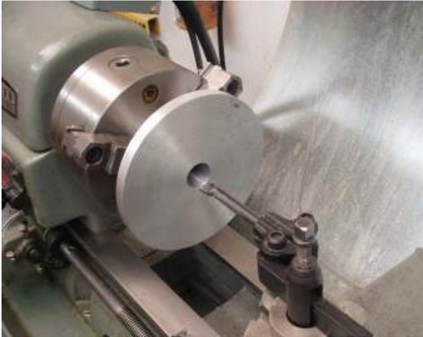
After facing the plate, I step drilled the center until I could fit in my boring bar. Then I opened the hole out to 1.000". I ended up at 1.002" but still had a slight interference fit with the bronze bushings. Luck was with me. This bar has a lot of spring in it so it is very easy to open the hole too much.
