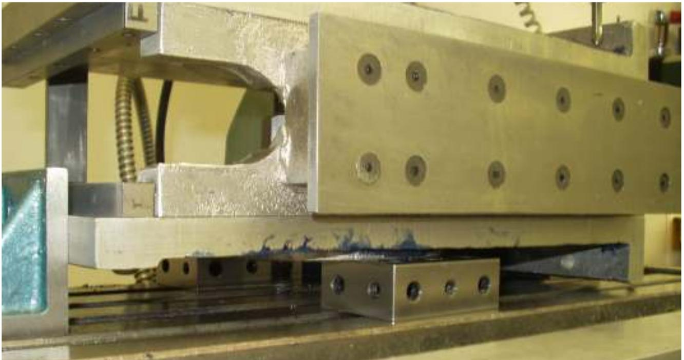
The bolt rings are secondary reference surfaces and sure came in handy. I put down two 1-2-3 blocks and clamped the casting to them. You can't see it here, but I have a clamping bar pressing on the top of the lower side plate. A second clamping bar presses on the top of the upper side plate. This second bar is to insure that the top plate does not lift up. Angle plates press on the sides just in case the casting tries to turn.
