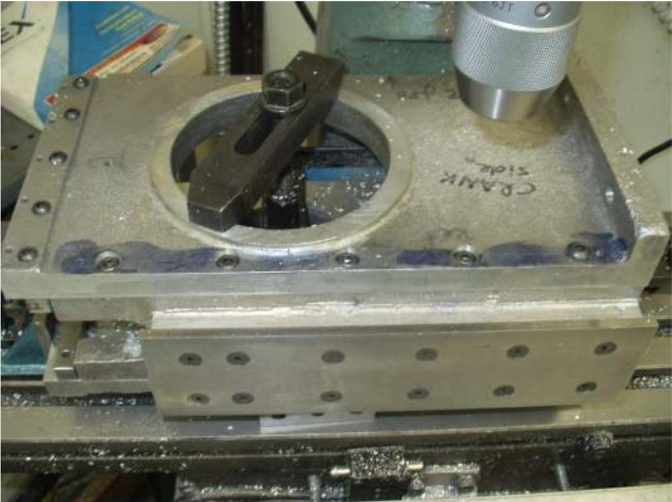
You can see that all but the right most screw sits in a counterbore. That last screw will be replaced by a much longer screw at a later date. The lower end of the table's vertical feed is supported by a small casting held in place by that screw.
