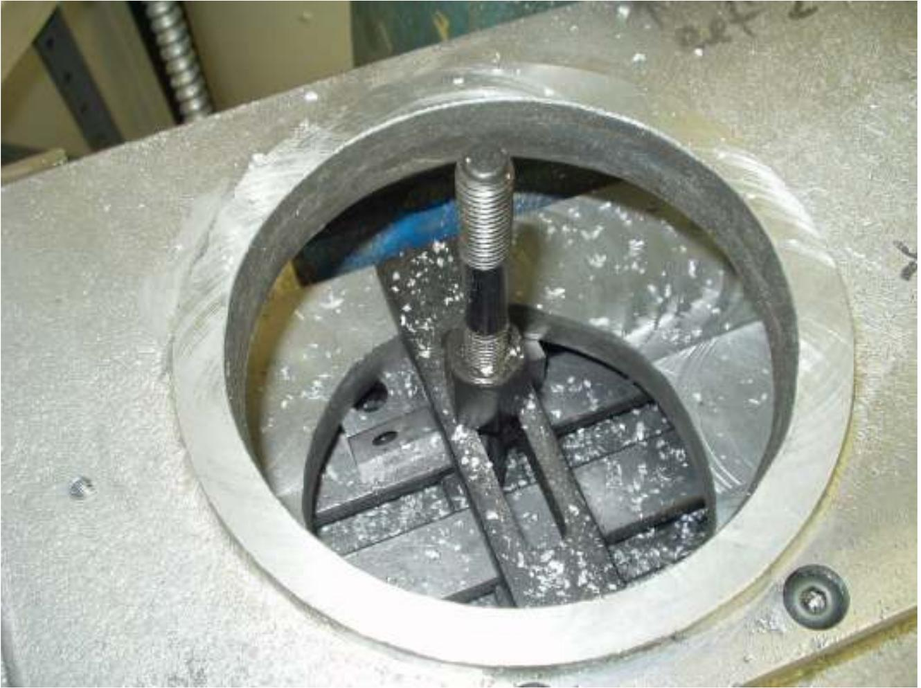
Here is a clear view of that lower clamping bar plus a good view of a counterbored screw.
