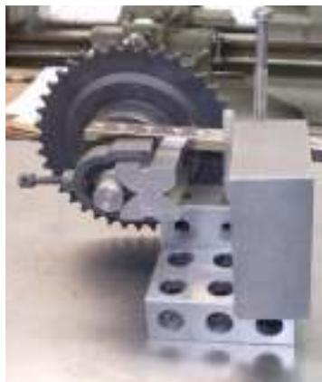
Next the sprocket was laid out. This was done by fitting it to a piece of scrap  $3/4''$  round stock. The round stock was then clamped to a V-block.
