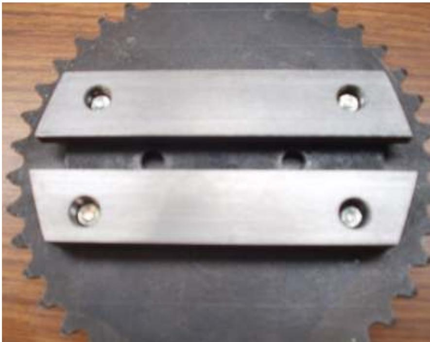
The attachment steps are repeated and the second bar screwed into place. As a final alignment step, all 4 screws are loosened and the parallel placed in the slot. Using my vise to apply gentle pressure on the bars and therefore on the parallel, I tightened all four bolts. My gap is now a precise  $5/8$ " wide and parallel.
