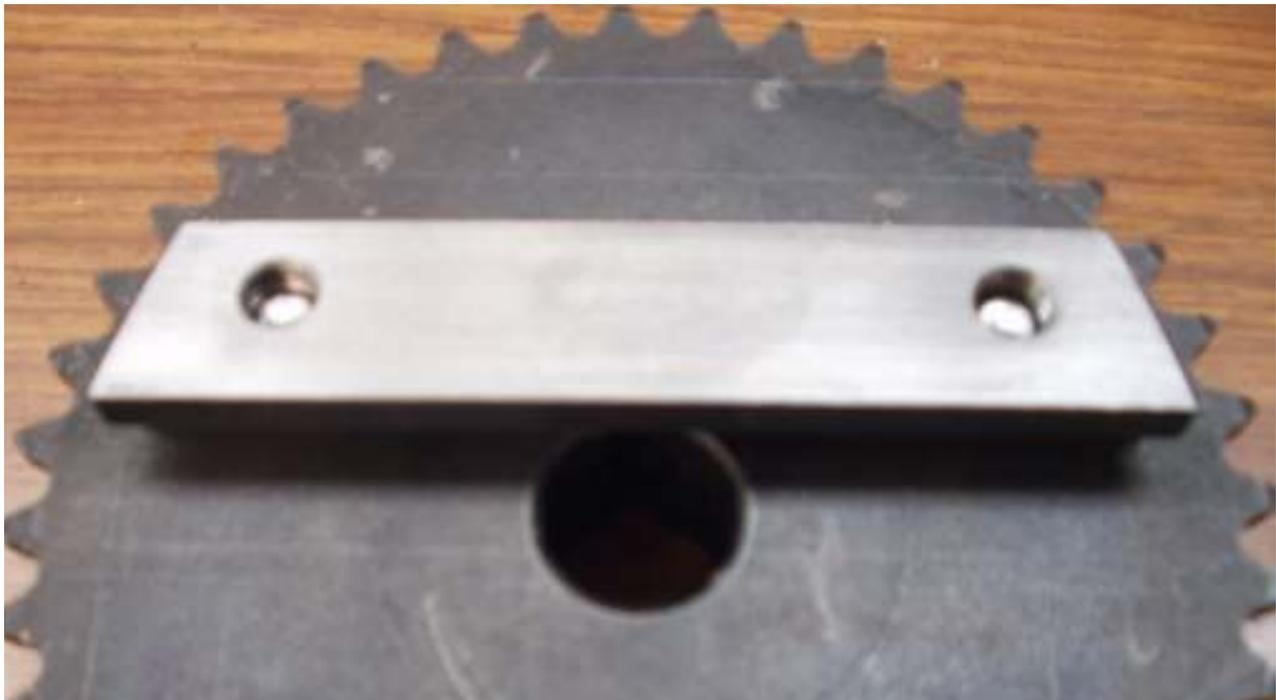
The bar is then secured to the sprocket using two grade 5 bolts and lock washers. The position of the second bar is more critical than this first bar. The gap between bars must be uniform. This is rather easy to do as long as it is not measured.
