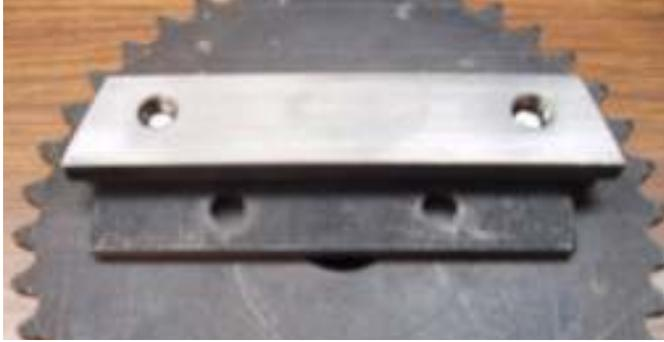
I want the distance between the bars to be  $5/8$ " as measured against the sprocket. This is accomplished by just placing a  $5/8$ " parallel down and pressing it against the first bar.
