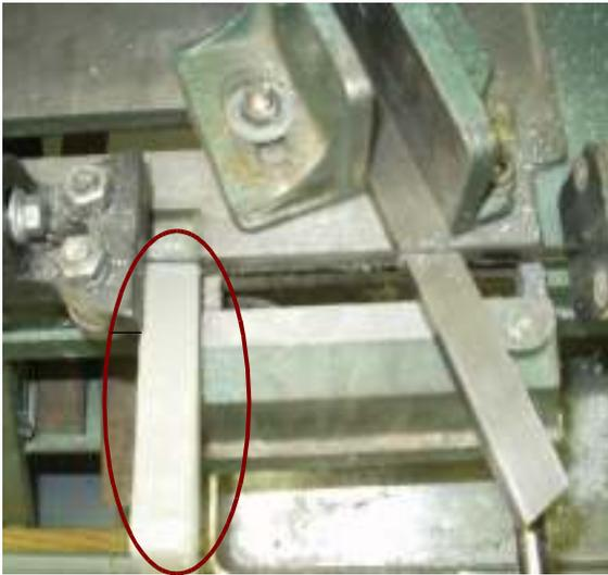
One thing of note here is the block of paraffin wax on the left side of the picture circled in red. My bandsaw blade teeth first cut across this wax and then cut the CRS. In this way cutting lubricant is freshly carried into the cut. The cut end of the bar had an even coat of wax on it indicating that there was plenty of wax present.
