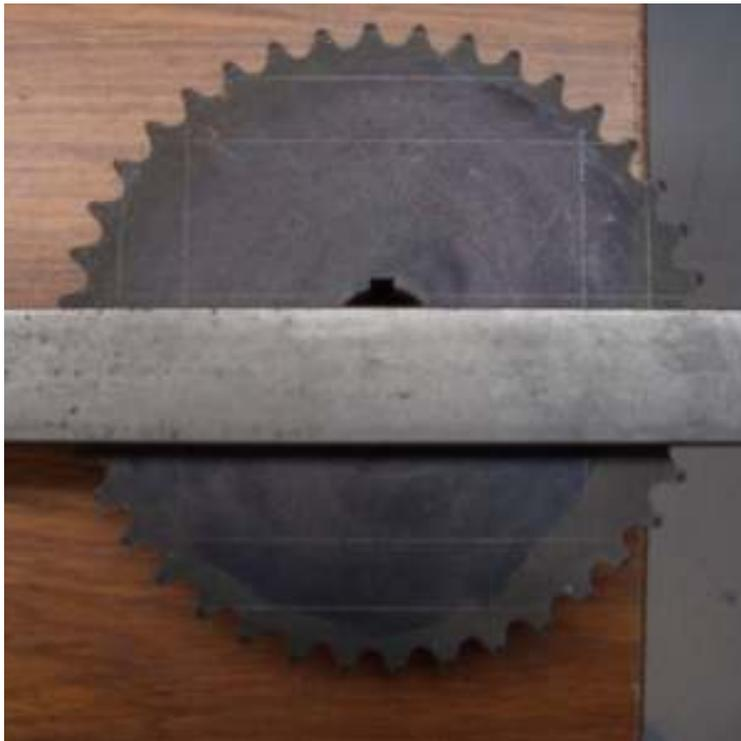
The next step is to place the first bar. Since each bar has a step in it, lining up this bar by eye is difficult. Instead I placed a straight length of CRS on the scribed line as a fence.
