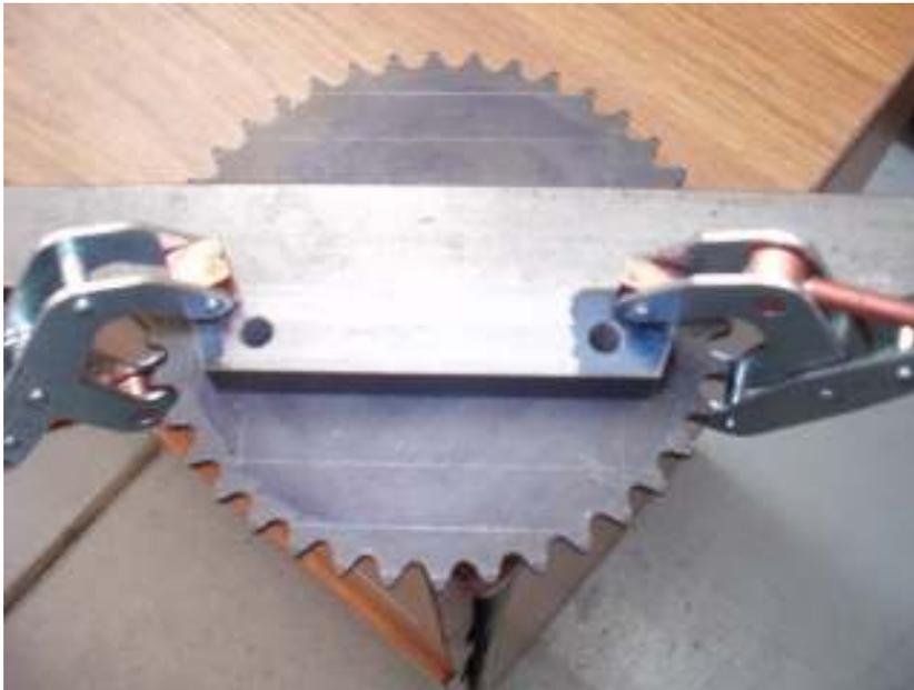
The first bar is then clamped in place against the fence. This bar's placement should be as good as I can get to the scribed line but is really not that critical.
