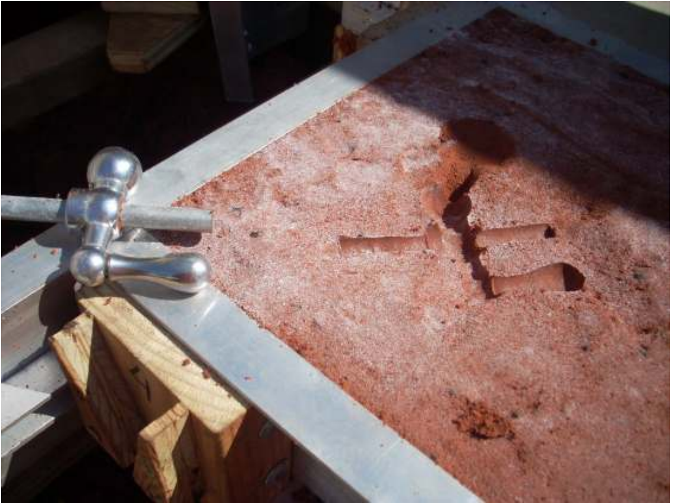
Here is the cavity formed in the drag. The gate has been cut from the ball over to the sprue imprint.
