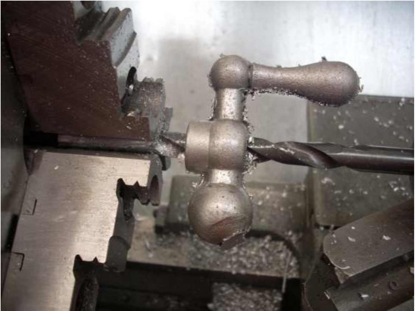
I drilled until the ball handle was cut free from the cast in rod.
