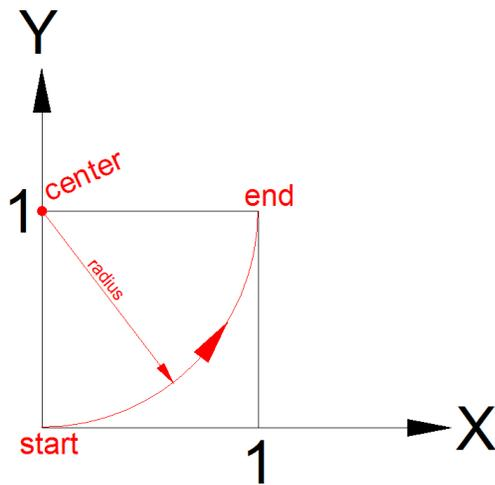
Here is an example of one possible arc. It is drawn on the XY plane with the center located at  $X=0$ ,  $Y=1$ . It starts at  $X=0$ ,  $Y=0$  and ends at  $X=1$ ,  $Y=1$ . This means it is moving in a counterclockwise direction. Given the defined center and both starting and end points, the arc must have a radius of 1.
