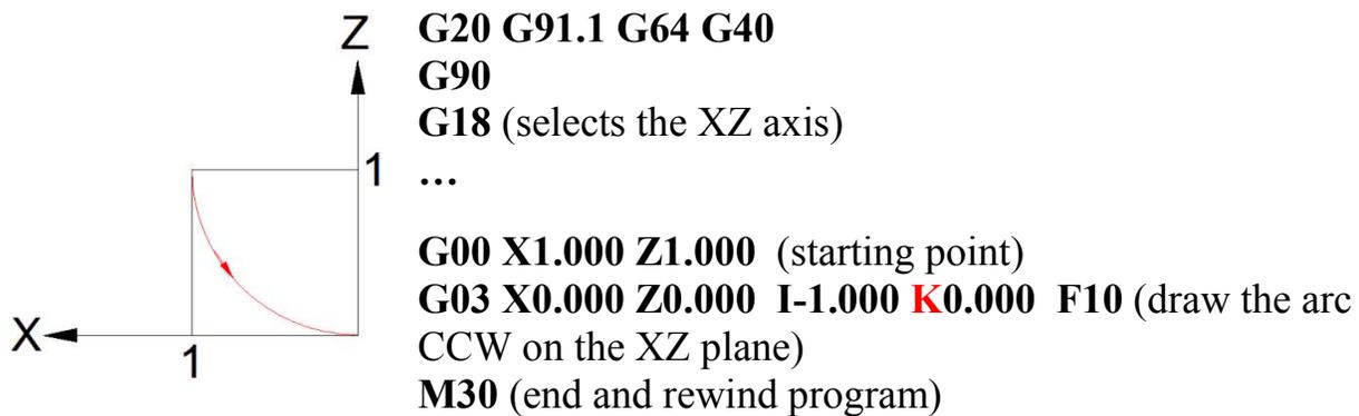
The start of the arc is at  $X=1, Z=1$ . The end of the arc is at  $X=0, Z=0$ . The center of the arc is at a -1 offset from the start along the X axis and at zero offset along the Z axis. If the flip in the direction of the X axis confuses you, please refer back to page 4.
