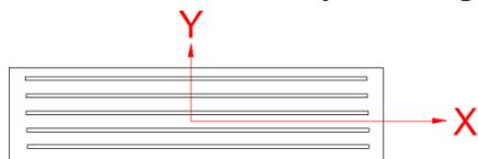
Thinking about my mill spindle relative to the table, a positive X movement causes the Center Of Rotation (COR) to move to the right relative to the table. A positive Y movement causes the COR to move from the front of the mill towards the column.
