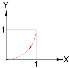
A word about the definition of clockwise and how it relates to the three planes. Consider the case of a clockwise rotation on the XY plane.
