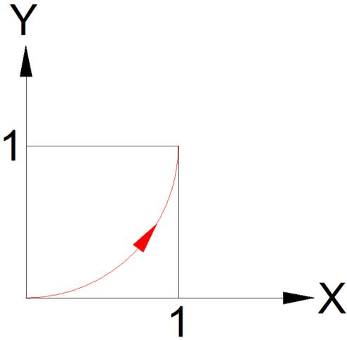
**F10** is the feed rate. Else ware<sup>2</sup> I have specified that I want to use inches and not Metric so the "10" means *inches* per minute.
