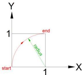
Notice what happens when we just change from counterclockwise to clockwise. The center of the arc moved from  $X=0, Y=1$  to  $X=1, Y=0$ .
