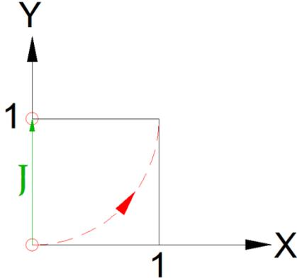
The next line of the program tells Mach3 that we are working in the XY plane. This is done with the **G17** command. If I were to specify a plane different from the one defined in the arc command, Mach3 will stop interpreting the arc command and flag an error.
