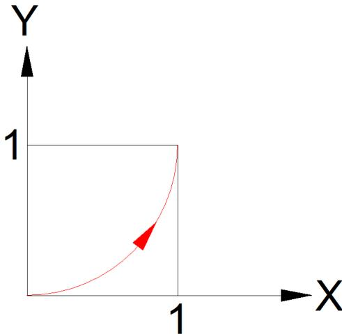
Here is where things start to look a bit strange. But stick with me because this approach actually makes a lot of sense. **I0.000 J1.000** specifies the center of the arc with respect to the *starting* point,  $X=0, Y=0$ . In other words, **I0.000** and **J1.000** are incremental rather than absolute. They tell Mach3 the increment between the starting point and the center of the arc.
