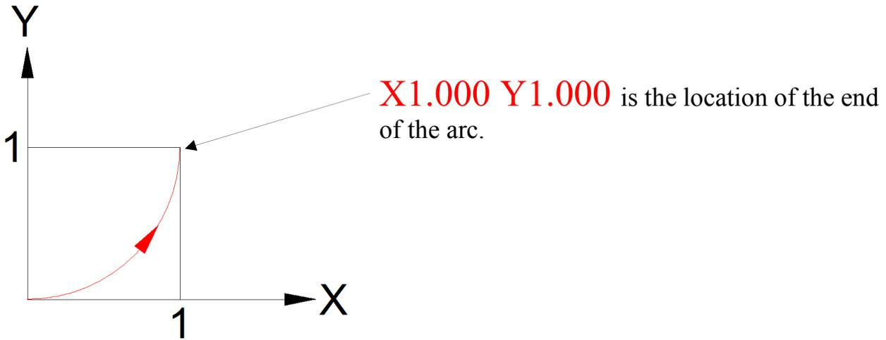
So far, we know the starting point of the arc because it was defined by a previous G-code instruction. The end point of the arc is specified within the arc instruction. We also know the direction the cutter following this arc will move. What is not yet specified is the center of the arc.
