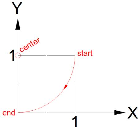
That **I-1.000** is telling Mach3 that the center of the arc along the X axis is to the left of the start. Moving to the left along the X axis is a negative move.
