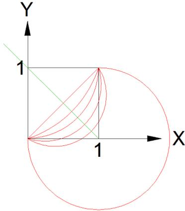
Here I have held the start and end points of various arcs constant and changed the center of the arcs along the green diagonal line. Notice that I generated a family of arcs. The straight red line passing through the center of the square is for an infinitely large radius. The longest arc is with its center on the X axis.
