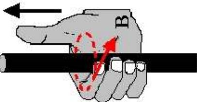
An alternate way to think about clockwise relative to a plane is the "right hand rule". Visualize the axis point out of the plane in the positive direction. Then point your thumb along this axis in the negative direction. Your fingers will curl in the clock wise direction.
