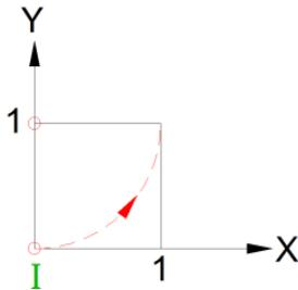
An **I0.000** tells Mach3 that the center's X axis position is zero distance along the X axis from the start point. Since we started at  $X=0$  and move a distance of zero, the X location of the center of the arc is also at zero.
