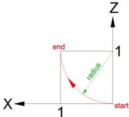
Walk around to the back of the mill. Then use your X-ray vision to look through the column. OK, you are now looking at the XZ plane in the negative Y direction. But wait! Isn't my arc now moving in a clockwise direction?
