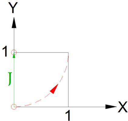
Similarly, **J1.000** tells Mach3 that the arc center's Y axis position is 1 inch along the Y axis from the starting point. Since we started at  $Y=0$  and move a distance of 1 inch, the Y location of the center of the arc is at 1 inch.
