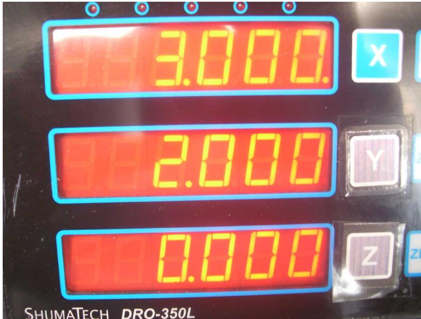
I have now cranked the X axis so my spud is 3.0005" to the right of my origin and my Y axis 2.0000". These are the exact value on the display. Please do not confuse the precision of the numbers with the absolute accuracy of the DRO. That is a different can of worms<sup>3</sup>.
