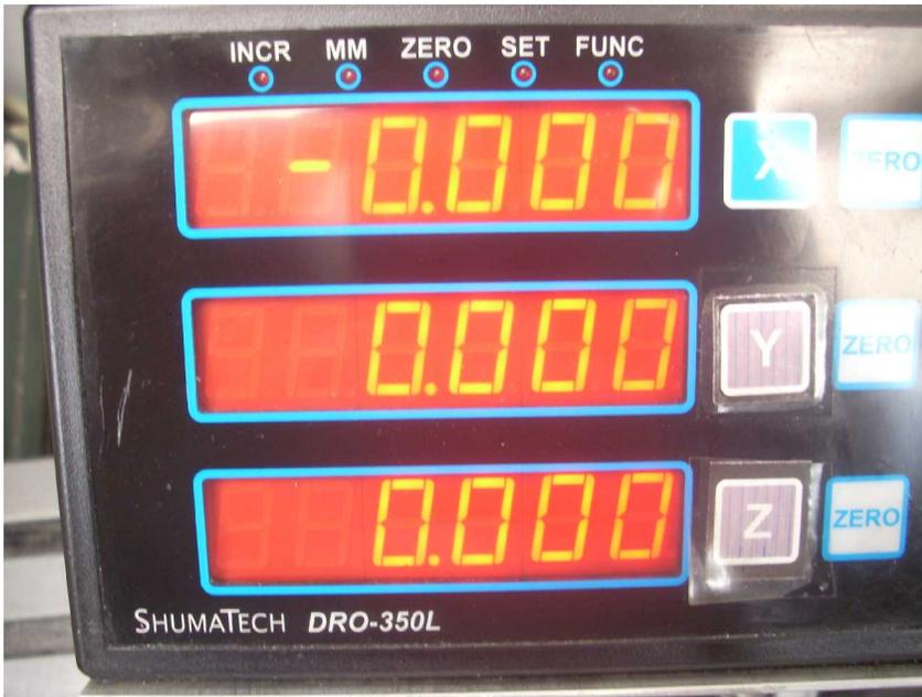
Sorry about the glare, but you can hopefully see that I now have my X and Y axes zeroed. My X axis shows a negative sign in front of my zeros while the other two axes are positive zero. This is not important. Both mean zero.
