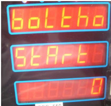
We are being asked to define the starting angle for the circle. Because I have my X axis set to [reverse [no and my Y axis set to [reverse [yes, hole 1 will be in the front and sequence counterclockwise. My angle will start in the front and also go counter clockwise.
