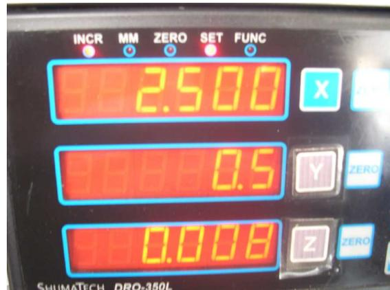
Say I want to move my Y axis INCR 0 such that I am at +0.5000". I first press the Y preset button and then input .5. the display shows 0.5" but internally it will be stored as 0.50000".
