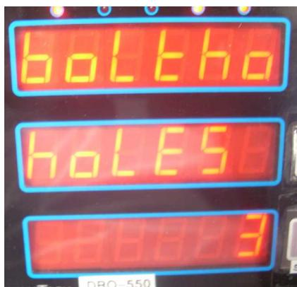
I chose 3. Sure hope I never need to enter 99! It could be handy if I was chain drilling a large hole. In fact, if you used a 2 flute end mill instead of a drill, you could use this function to rough cut a disk without using a rotary table.
