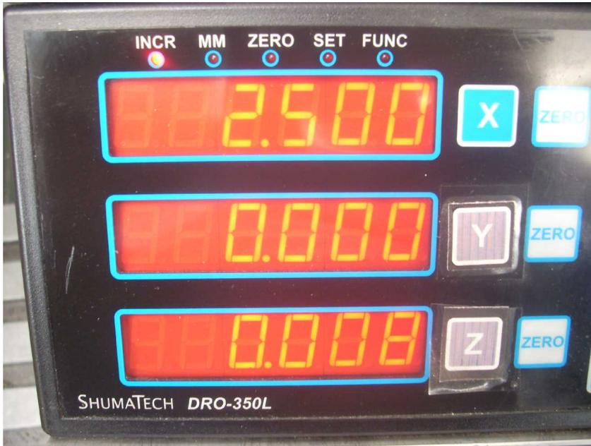
You can see from the LEDs that we are now in INCR mode. Our INCR X value is now 2.5000". The INCR Y value just happened to be zero and INCR Z was 0.008". The change to the INCR X axis has no effect on the Y and Z axes.
