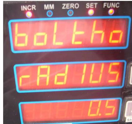
And at what angle do you want the arc of holes to end? If you just press Enter, the holes will be equally spaced around the entire circle.
