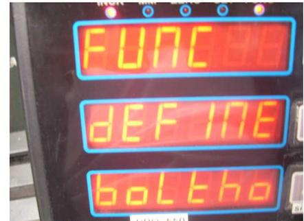
It is time to define the bolt hole circle pattern. I press FUNC, then push the Y preset until I see [define in the Y display. Then I press the Z preset until I see [bolt hole. Pressing Enter starts the function.
