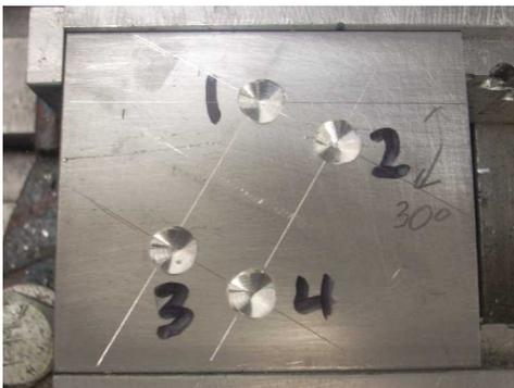
I have scribed lines between centers plus marked out the angle. Note that the 4 hole array has been rotated by 30 degrees. The holes are each 1/4" in diameter. The distance between holes 1 and 2 is 0.5". Between holes 1 and 3 is 1.0".
