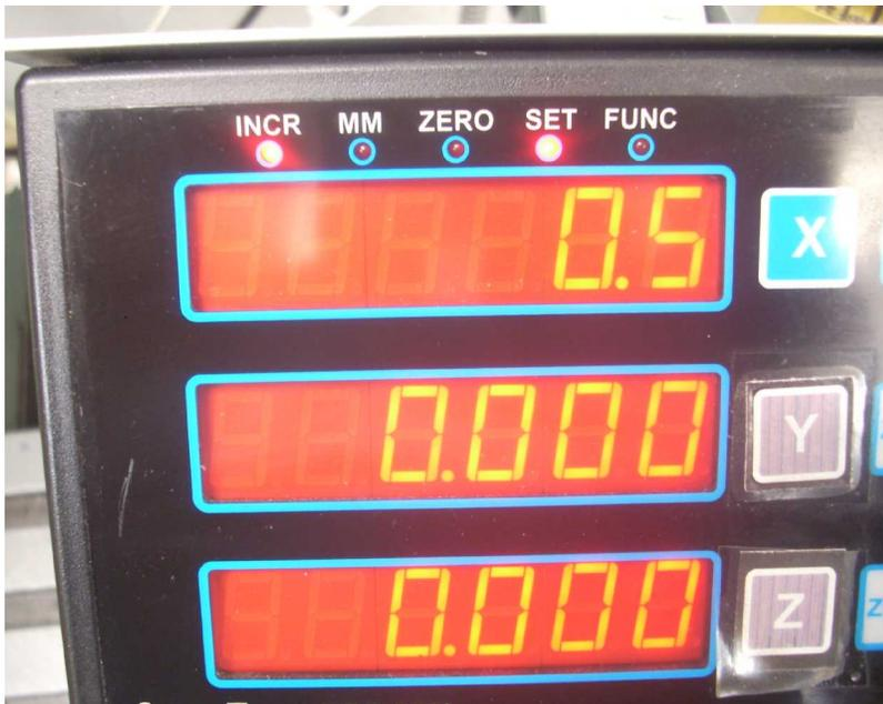
Now, let's do it again but this time looking at the DRO. I start out at an ABS X = 3.0000". I press the X preset button and input ".5" which displays at "0.5". Internally it will be stored as 0.50000".
