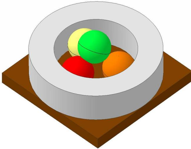
Take 4 balls of identical diameter and place them in a known diameter hole that is perfectly round.
