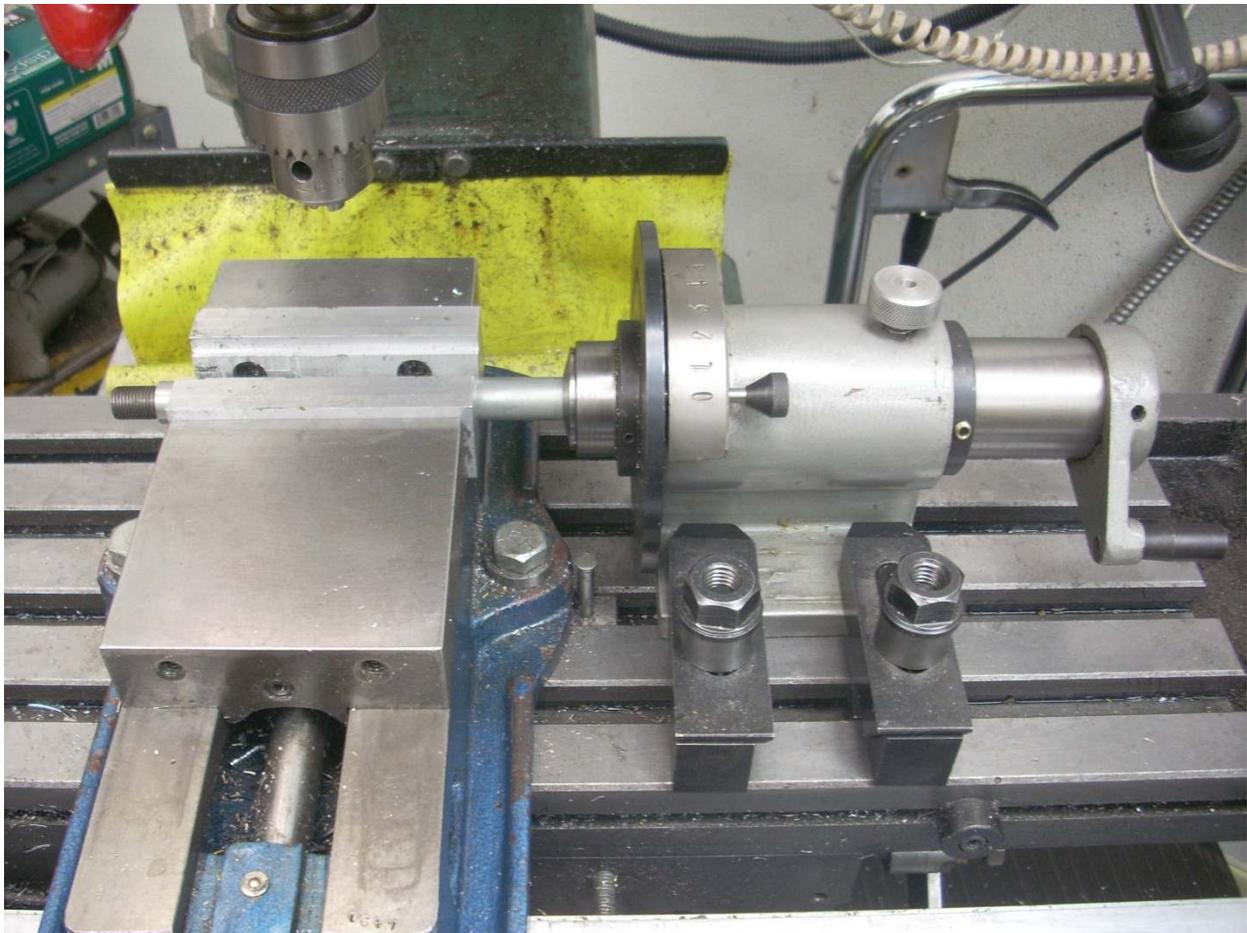
I will use my 5C collet spinner to position the 3 holes exactly  $120^\circ$  apart. The first step is to align the center of rotation of the spinner with the X axis of my mill. Since my vise is already aligned, I just chucked up a piece of  $\frac{1}{2}$ " bar stock and clamped it in the vise and spinner. Then I tightened the clamps on the spinner.
