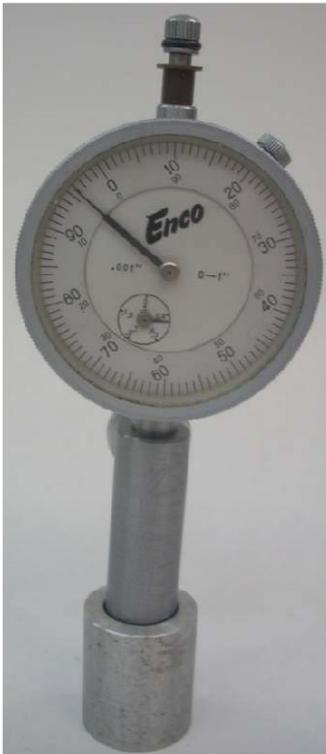
I placed a spacer in the calibrated ID cylinder to raise the gage up so it would contact the upper ID. The gage reads 0.004" and not 0.0045" because it is not straight.
