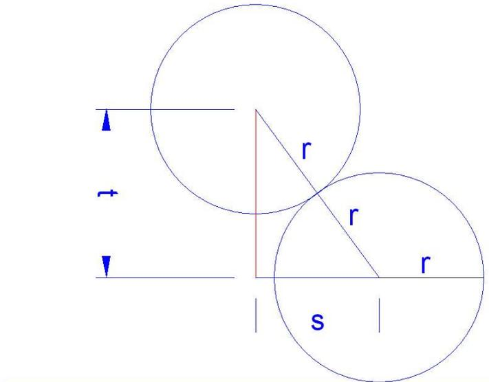
Looking again at the figure, note that I have a new value for  $t$  but the same value for the hypotenuse,  $2r$ . So I can calculate the new value for  $s$  by rearranging equation 2.
