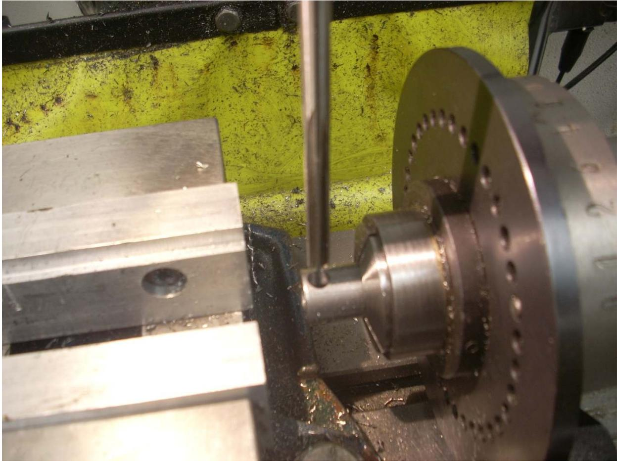
The body was then clamped in the spinner using a 5/8" 5C collet and the spinner's rotation locked. I used my DRO to find the centerline of the part and the end. Then I moved in 0.175" and locked my X and Y axes. For each hole I started with my spot drill, then a 7/32" drill, and finally my reamer. Rotated the part 120°, locked the spinner, and repeated the process two more times.
