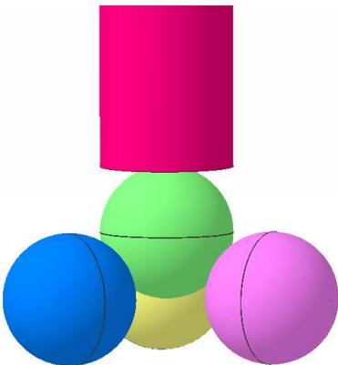
As the top ball is lowered, the bottom three balls move out. The precision of the instrument depends on the precision of the balls plus the holes that guide these balls in the body. All holes are reamed for a close sliding fit and precisely set  $120^\circ$  from each other.
