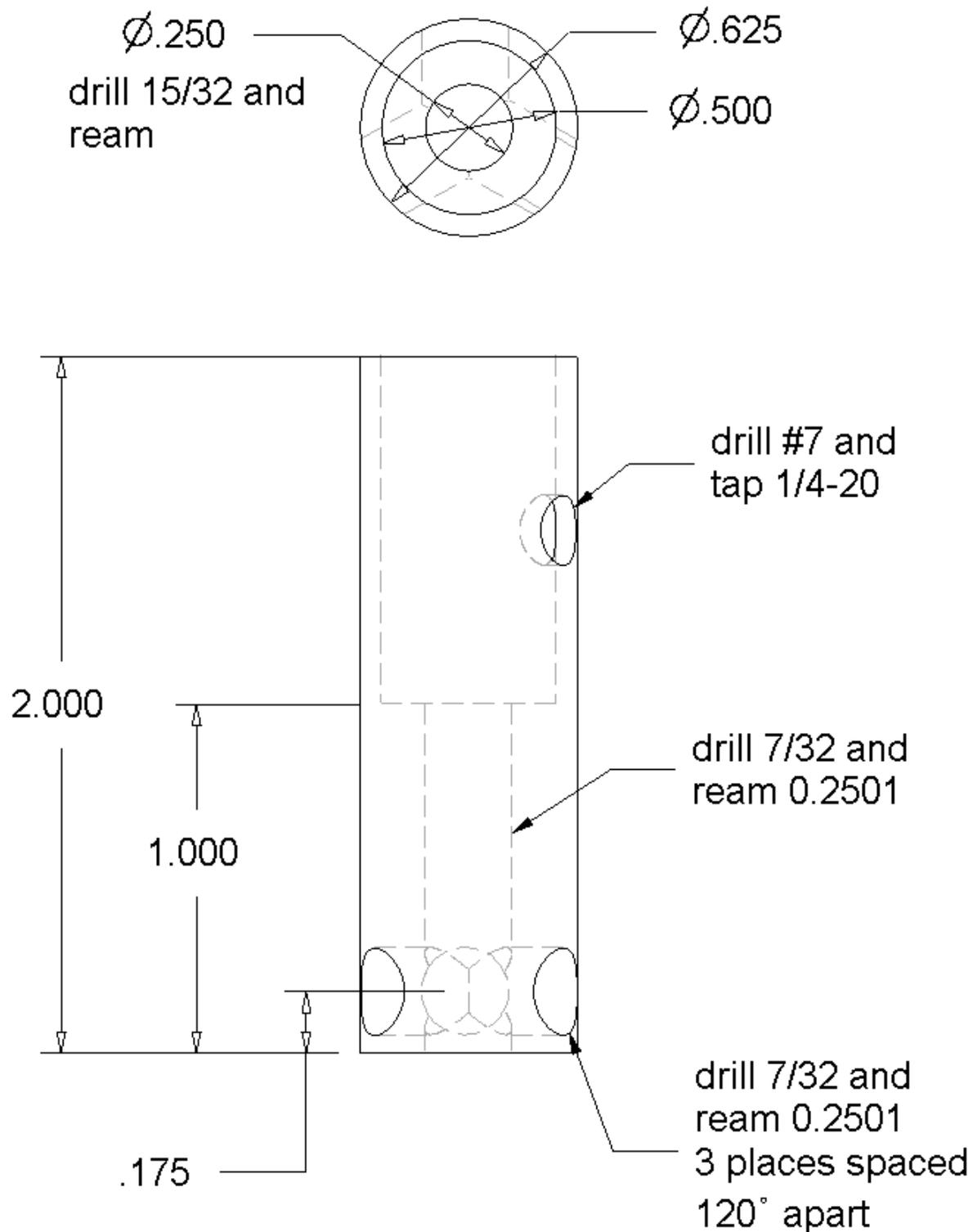
The gage is shown to be 2" long but by placing a longer push rod down the center, you could make the gage just about any length you want.
