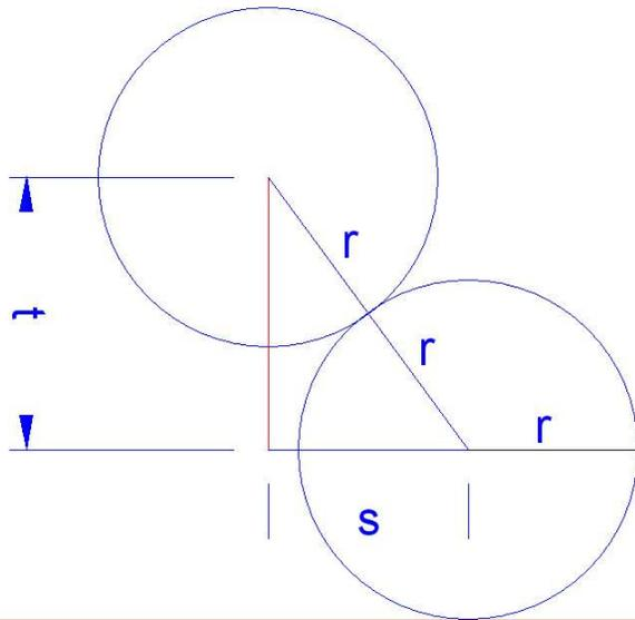
A side view of just one of the 3 bottom balls and the top balls is shown here. All balls have a radius of “r”.
