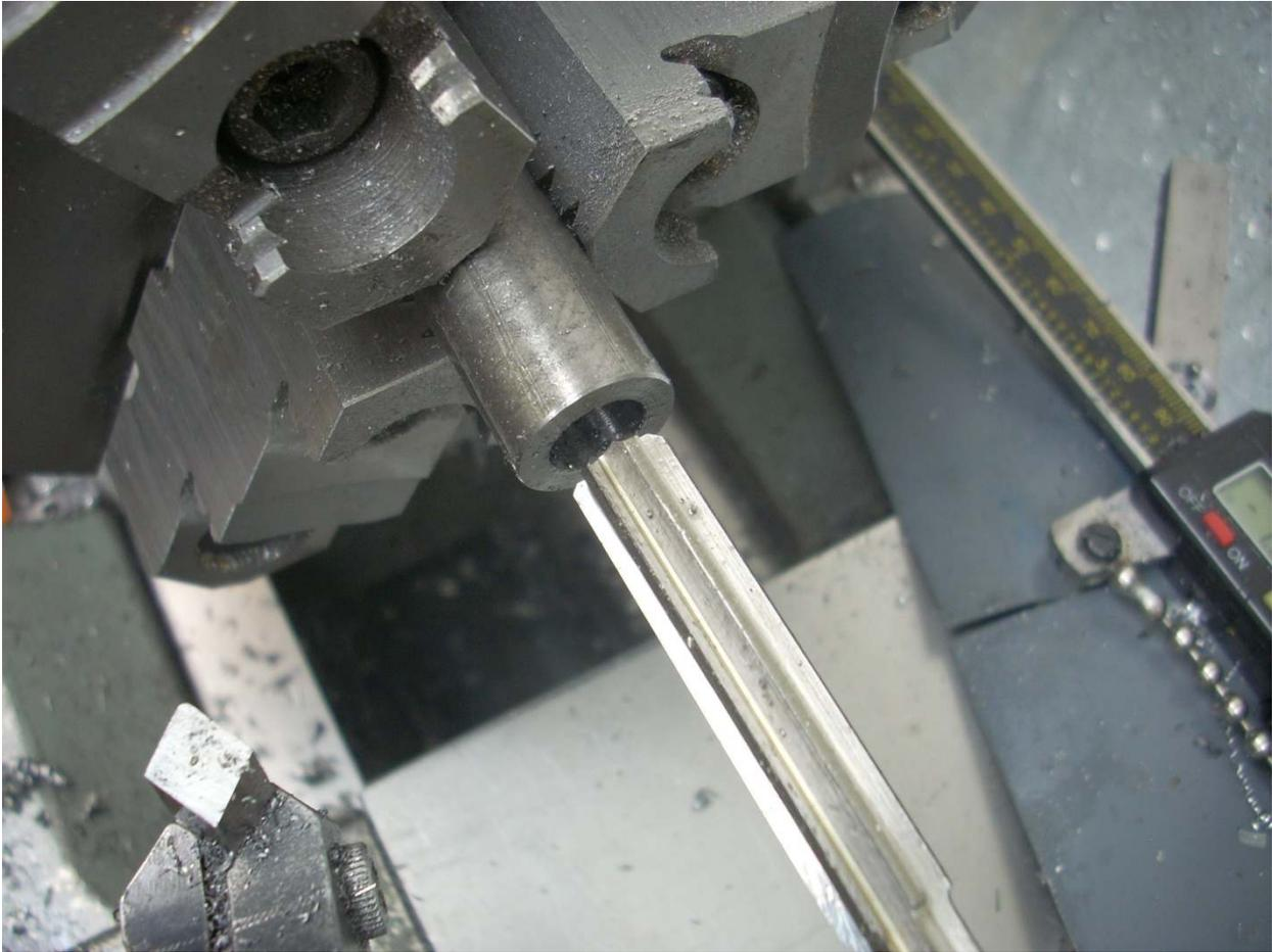
After facing the end of the body, I drilled  $7/32$ " and reamed to 0.2500. It was a bit snug so I have specified using a 0.2501" reamer. I then drilled  $15/32$ " to a depth of 1" and ran a 0.500" reamer as shown here.
