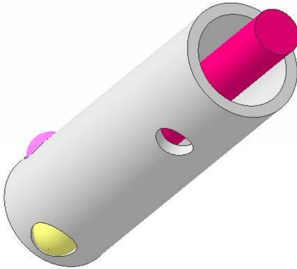
The red cylinder in the center is my Dial Test Indicator push rod. At the bottom you can see two of the 3 balls that contact the ID being measured. The hole in the side of the body takes a locking screw for holding the DTI in place.
