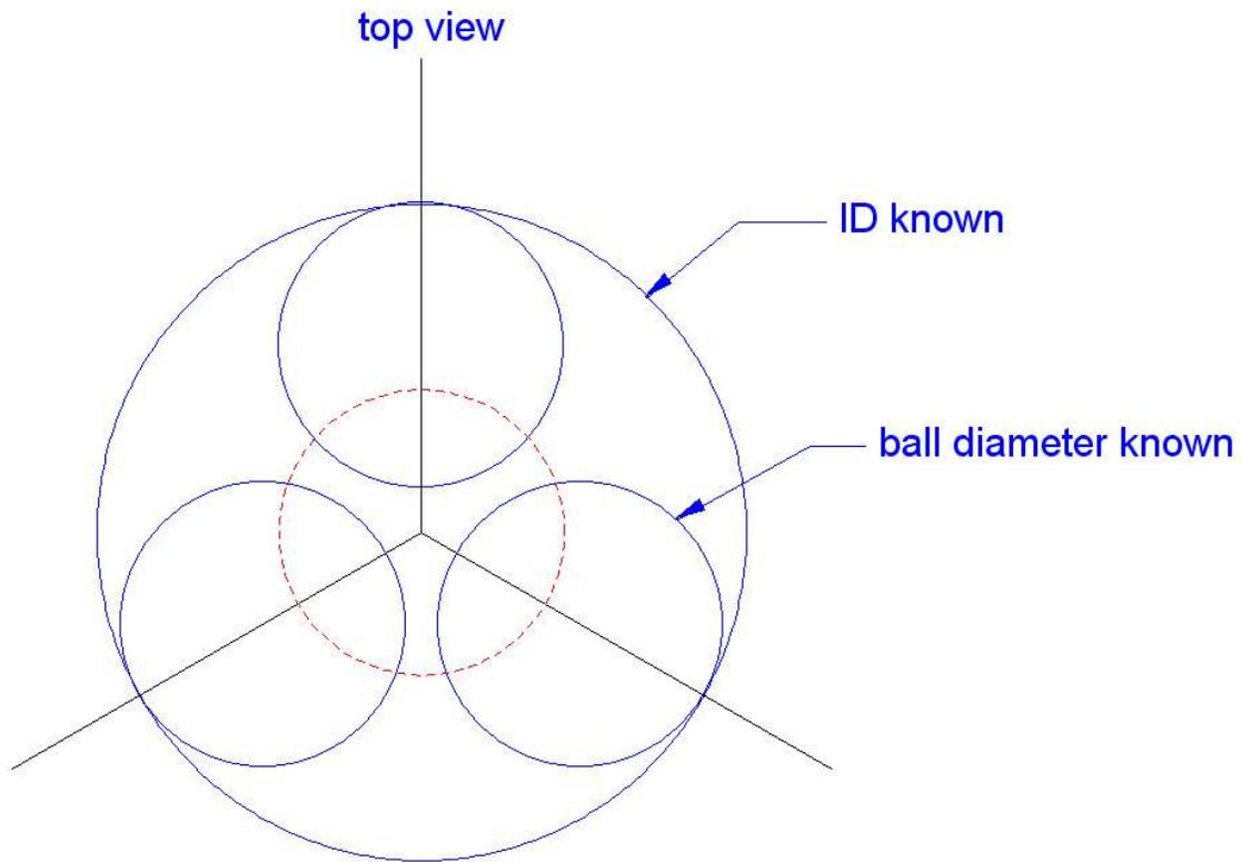
Here is a top view of the 4 identical balls. The bottom 3 balls are on a plane and the forth ball rests on top (shown as a dashed red circle). The 3 balls are constrained by a cylinder with a known ID as shown.
