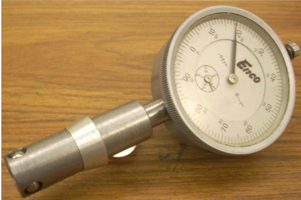
The collar was made of aluminum. The hole down the center should be a close fit to the body of the gage. The taper angle is not critical but I chose to set my compound at 10° and it seems to work well. Do take care when cutting the taper
