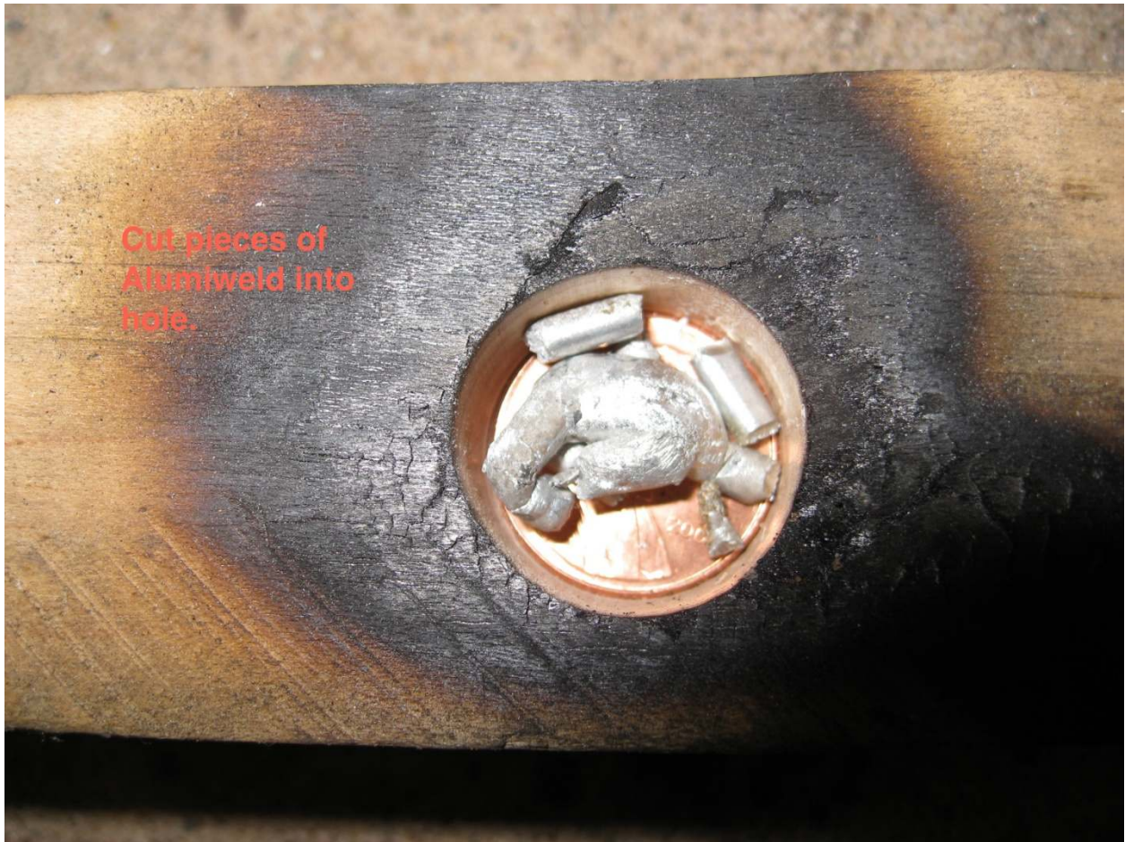
Using the torch, the aluminum brazing rod is melted into the mold a little at a time.
