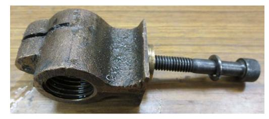
Here is the Y axis nut with cap screw.
