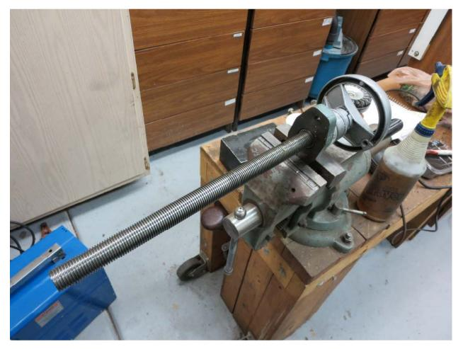
I clamped the Y axis lead screw with handle into my bench vise. This makes cleaning and inspecting the threads easy.
