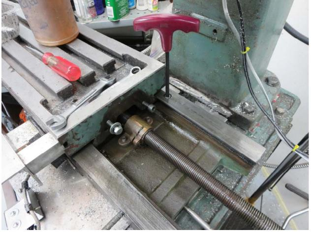
Danger: if your mill is not secured solidly to the floor, moving the table over this much could cause the mill to fall over. You may need to support the left end of the table.
