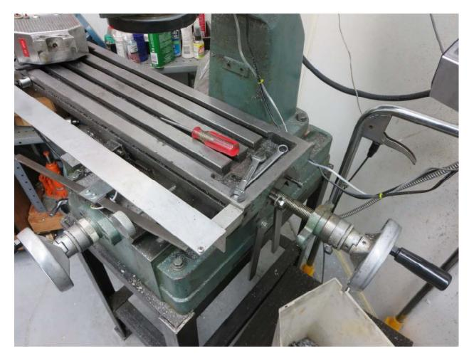
You can now turn the crank on the right side of the table a few turns to get it out of the way. No need to completely remove the X axis lead screw.
