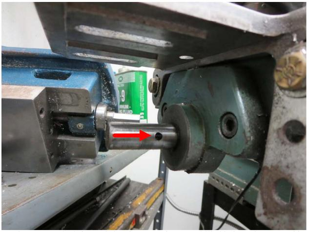
Moving over to the left X axis bearing, note the cross drilled hole (red arrow). This hole is tapered. Use the original roll pin to locate the larger diameter end of this hole. Have the larger diameter facing towards you.
