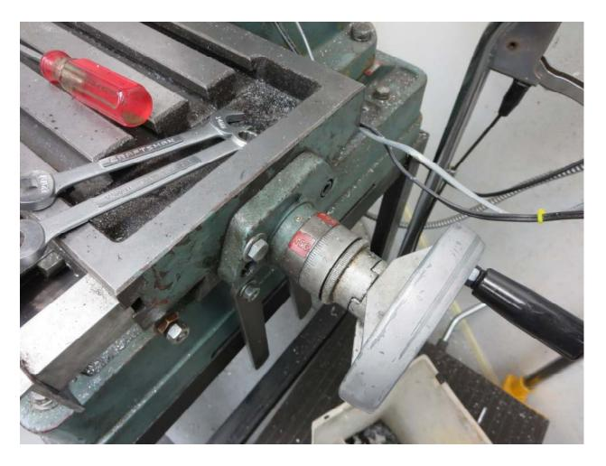
My right bearing probably doesn't look like yours. I have one original cap head screw and one head hex screw<sup>3</sup>. Remove both screws.
