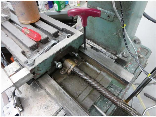
Reinstall the Y axis nut but leave the bolt a little loose.
