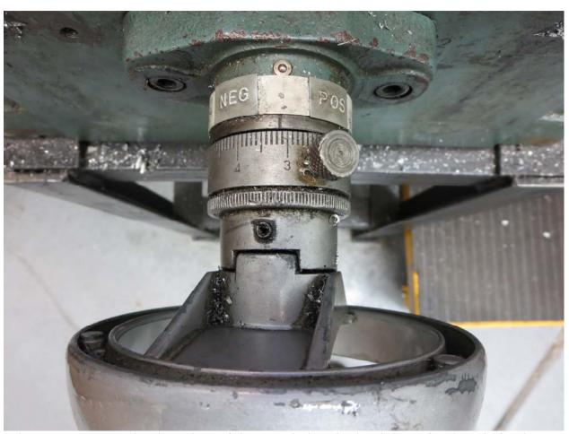
When you reverse the direction of the Y axis hand wheel, how far does it freely turn before the table moves? This backlash might be due to worn threads but it is more likely due to a loose nut<sup>2</sup>.
