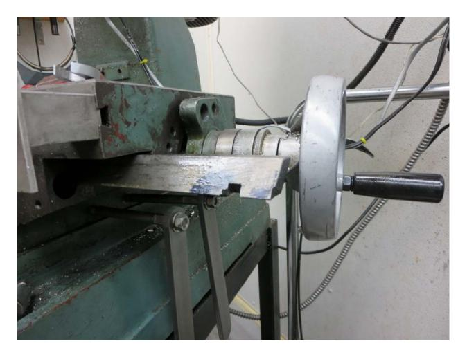
Next, unscrew the right X axis bearing retaining bolts and slide out the gib.
