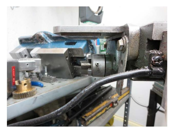
My left X axis bearing has a power feed on it. Those are the bits laying on the shelf all the way to the left. The original crank coupler is still on the shaft. Drive out the roll pin and this coupler should slide right off. No need to remove the bearing.
