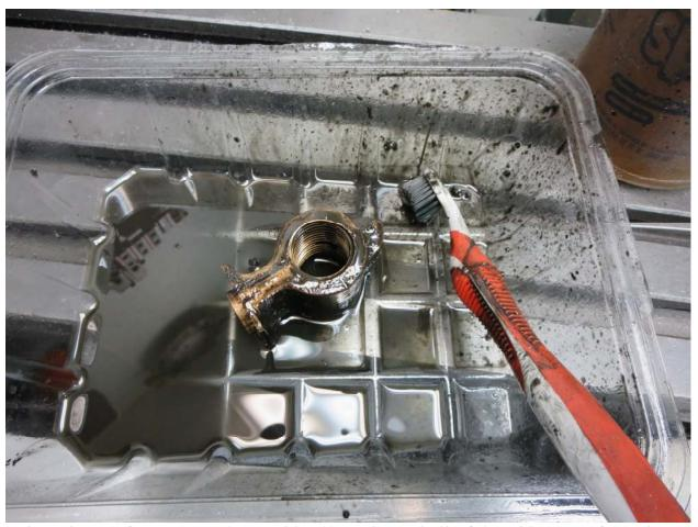
Using plenty of WD-40 and a toothbrush, I cleaned all of the old grease from the Y axis nut. Only then can you clearly inspect the threads for wear and damage. Mine didn't look half bad even though I have owned this mill/drill since 1990.
