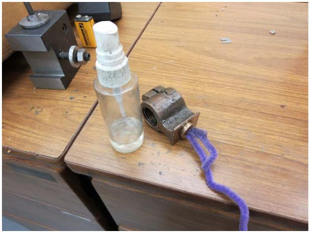
I used alcohol and a pipe cleaner to remove all grease and oil from the threads of the screw hole. I then cleaned the cap head screw with alcohol and toilet paper. Be sure all thread surfaces are clean and dry.
