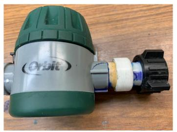
Using PVC primer and cement, I welded the parts together.
