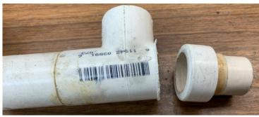
I chucked up a scrap with a T in it. A short length of pipe stuck out the end. Then I turned the end for a tight fit into the body of the timer before parting it off.
