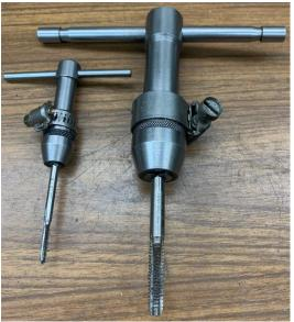
When I finally paused and thought about the problem, the solution jumped out at me: hose clamps!
