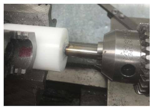
Here is your 10 seconds of excitement. While you push the tailstock towards the headstock, turn the 3 jaw chuck counterclockwise by hand. As long as the end mill is hot enough, it will easily screw itself into the plastic. There will likely be a little smoke and maybe a brief flame
