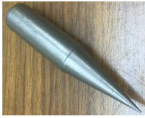
No, I have not changed my hobby to cooking. In metal working, a spud is a piece of round stock with a point on the end. You chuck it into the mill spindle and use it to roughly locate a point by eye. Rather useful and easy to make on a lathe.
