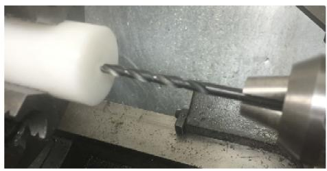
Then I drilled in about an inch using my 11/64" drill. Acetyl cuts like butter but tends to contract after the drill is removed.
