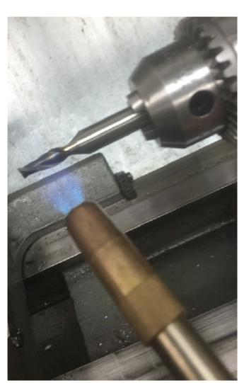
Here is where having a scrap end mill will save you time. You must heat the end mill to above 400° F.
