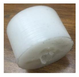
The resulting puck has molding flash on one end and a drilling burr on the other. I just cleaned this up on my belt sander.
