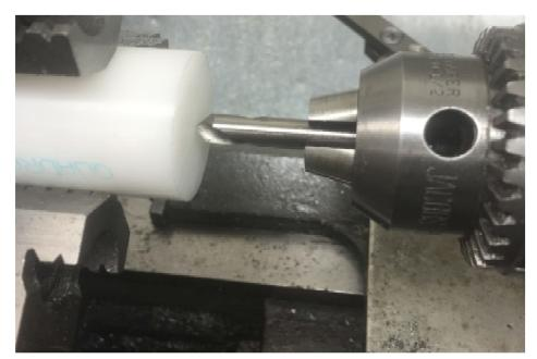
With a 2" length of Acetyl mounted in my lathe's 3 jaw chuck, I faced the end and then spot drilled.
