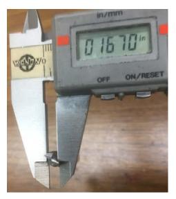
First, I measured the minimum diameter of the end mill. It was 0.167". I needed to remove enough plastic so it would not block this central core of metal. An 11/64" drill (0.1719") seemed about right.
