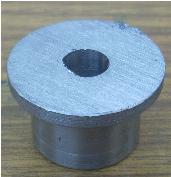
All that is left is to face this end and deburr it.
