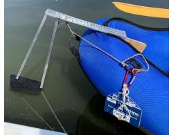
I'm still in the proof-of-concept stage as I move towards my final design of a skeg. Here you see it installed on my Sevylor Colorado kayak which is an inflatable. My previous design strapped under the kayak and had too much drag plus was hard to install and remove once in the water. The design you see here is much closer to the commercial design with a few important differences.
