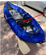
Without the skeg, when I stop paddling, my kayak rotates around where I sit and ends up pointing in the opposite direction. I figure that the further the skeg is from this pivot point, the more effective it will be in keeping me pointing correctly.
