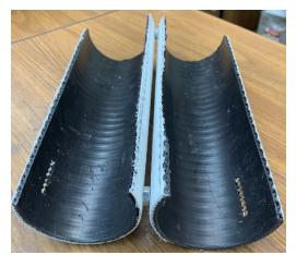
My second iteration involved cutting the pipes both axially and radially. At half the length and by being open, I figured the drag should be reduced. But as I looked at that corrugation, I knew it was still a problem. In fact, I never even tested this version. But it did get me thinking.
