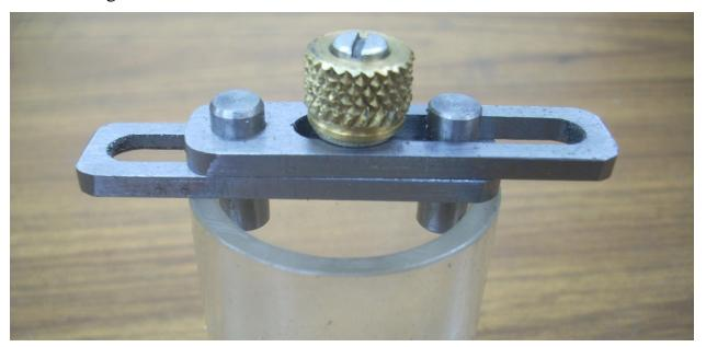
The gage is dropped into a hole, and the pins moved apart until they contact the walls. A little wiggling of the gage will guarantee that the pins stay on a diameter of the hole. Then the knob is turned to prevent further motion.
