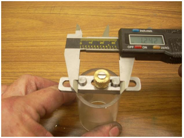
Then use a micrometer or caliper to measure between the pins as shown here.
