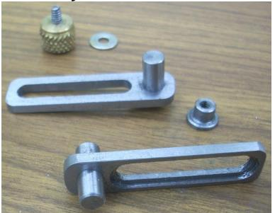
The pins should be a snug fit in the reamed holes. Use your mill or drill press to hold the Loctite coated pins and drive them squarely into the blades. The pin pressed into the Top Blade should extend 1/8" above the top surface. The pin pressed into the Bottom Blade should extend 1/4" above the top surface. Wipe any excess Loctite from the pins before letting them set up for 2 hours.
