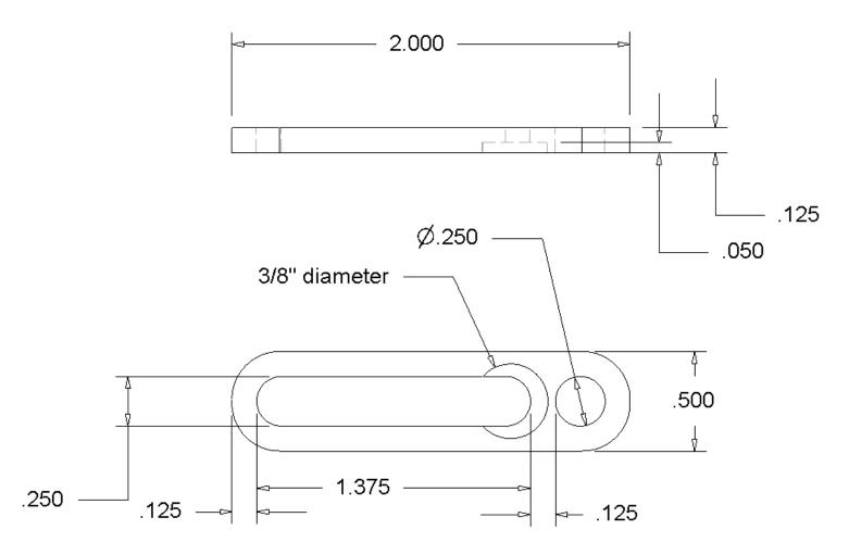
This part is identical to the Top Blade except for a 3/8" diameter recess at one end of the slot that is 0.05" deep.
