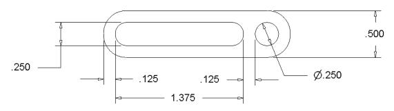
I cut the slot by first chain drilling with a "C" drill and then ran a 2 flute ¼" diameter end mill as my finish cut. The ¼" pins should be a sliding fit to the slot so some filing may be needed to smooth the sides. The 0.250" hole was first drilled with the "C" drill and then reamed with a ¼" reamer. It should be a snug fit to the pin which will be secured with Loctite® Red.
