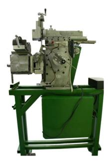
In the ideal case, a metal shaper could not be much simpler. A cutter moves back and forth across a surface while the tabling carrying this surface moves side to side<sup>2</sup>. The machine cuts a flat surface.
