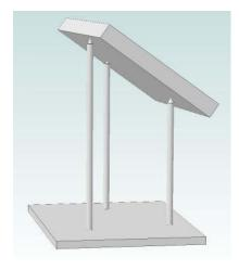
Then I can measure the height of each nail which tells me the Z axis value. The tip of each nail will therefore have a unique (X,Y,Z) value which must be in contact with the bottom plane of the plate.
