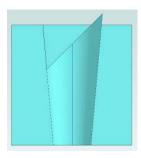
I'm still a novice with Alibre<sup>®</sup>, my 3D drawing program. You may notice that the cutting edge's tip is above the top face of the cutter blank. This is a problem with my use of the draft function. It is even more noticeable with the front view. However, this view does a good job of showing you the 5° relief.
