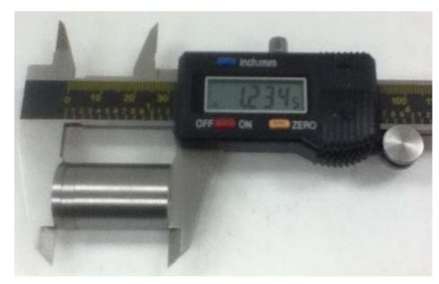
If you have a caliper of questionable accuracy but decent repeatability, you can use a stack of spacer blocks to measure within the resolution and repeatability of the caliper.
