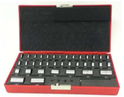
I was able to buy a 36 piece spacer block set for around \$40 during a past sale at Enco. This set enables me to make thicknesses between 0.150" and about 3" in steps of 0.001" within an accuracy of around ± 0.0001" per block used.
