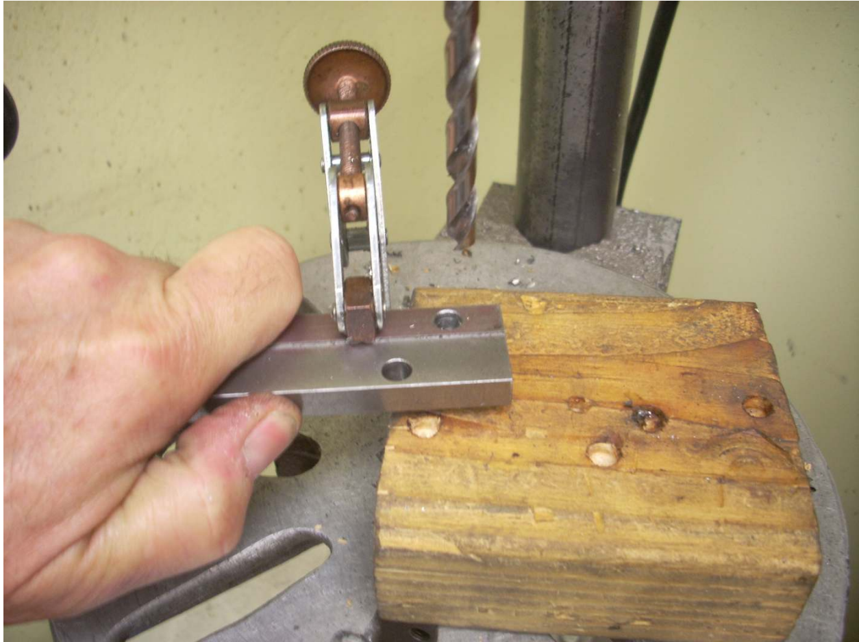
Then I used my 1/4" drill to match drill through gib plate and top gib.
