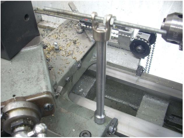
The modified universal simply snaps on top. I can always unsnap it if I need this extension. It is equally easy to swap in a different length extension.
