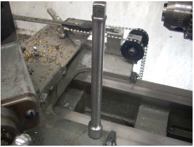
The 3/8" extension fits nicely onto the square locking bolt and is long enough that I clear the nearby compound and tail stock.
