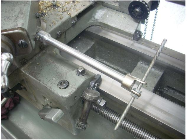
The tool is long enough for me to access the compound's locking bolts regardless of the angle of the compound.
