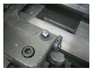
My lathe uses these 3/8" square locking bolts on the apron and compound. An *acceptable* wrench came with the lathe but somehow, I lost it a few years ago. Since then I've been using a 3/8" combination wrench which has also been *acceptable*.
