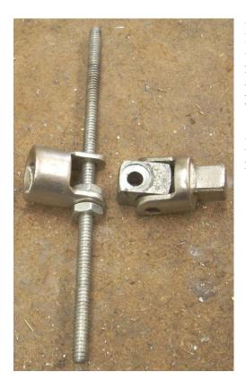
I drove the spring pin out of the universal. Then I took the female part and ran a 10-24 threaded rod though the ears. This is a proof of concept. I plan to machine a bar to go between the ears if this works out.
