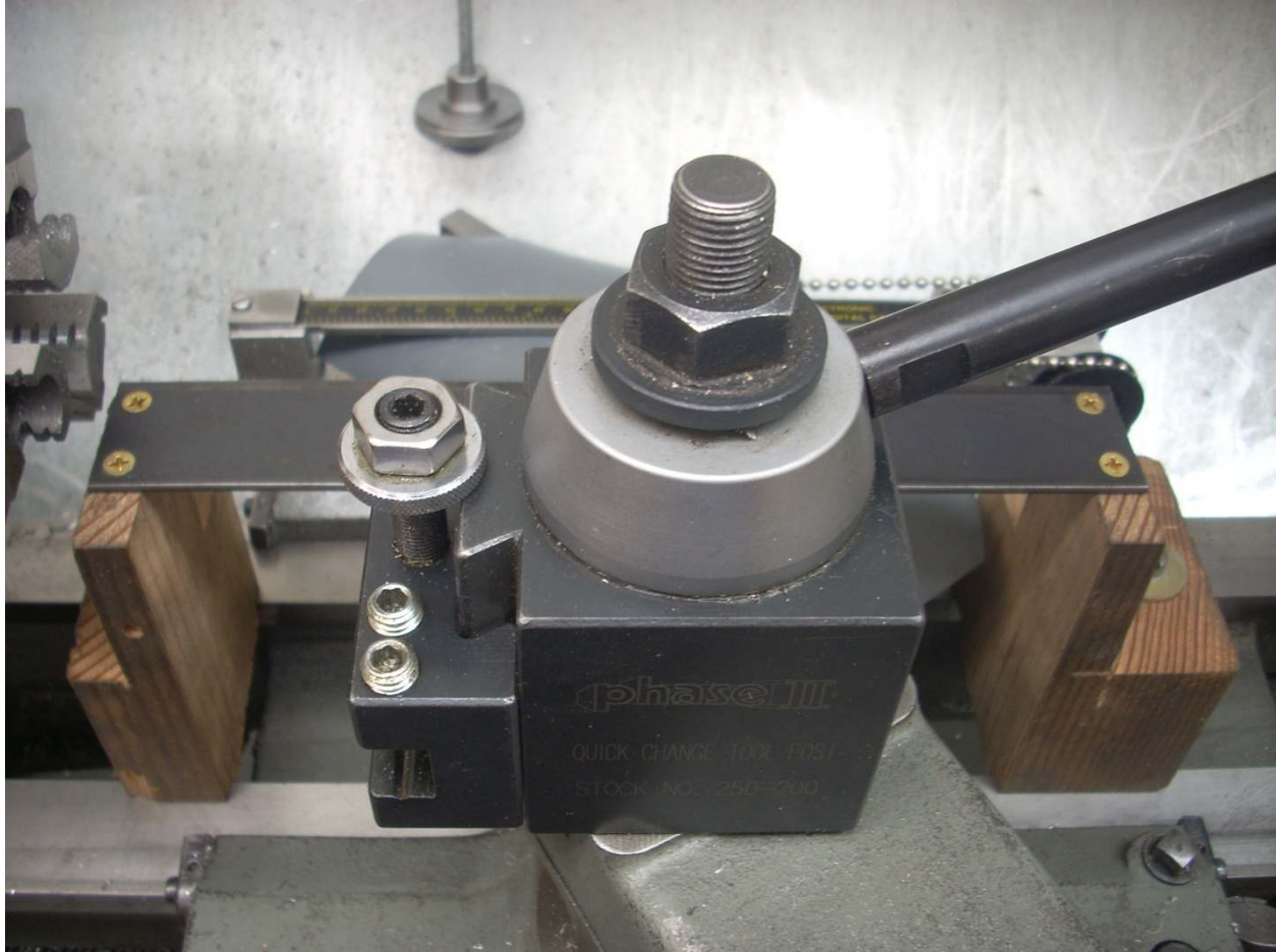
The follower table is mounted over the apron. The bolts in the blocks of wood engage bars that clamp the underside of the ways.
