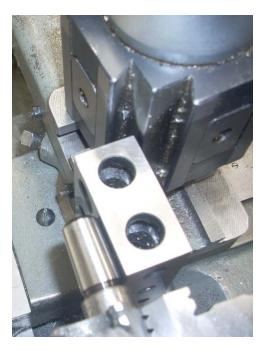
I am using a 1-2-3 block to align the ways of the compound to the taper. When no light is seen between the block and the taper, I lock the compound into position.
