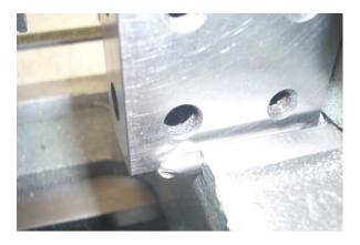
You can see a centering drill set into the dovetail. The 1-2-3 block contacts it.
