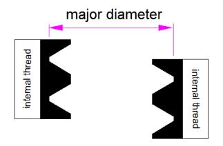
The final step is to verify and machine, if necessary, the major diameter. If the cutter has the correct profile, there should not be a problem here.
