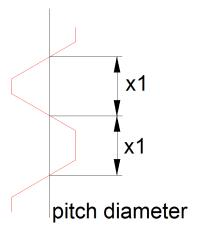
The internal thread is also defined partly by the pitch diameter. There is a minimum and maximum value.
