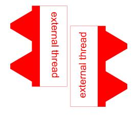
Next, take in the entire cross section of the bolt. Since this is a ramp wrapped around a cylinder, the right profile must be offset by half from the left profile. If they were lined up, the ramp would have no slope and it would be impossible to advance position as the bolt was turned.
