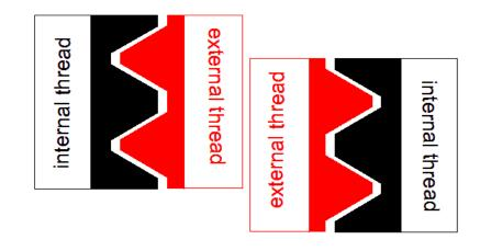
Looking at a cut away picture, we can see how the bolt's external thread engages the nut's internal threads to create a working "system". Although I show white space separating the
