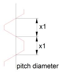
Adjust the diameter until  $x_1$  equals  $x_2$ . Then the pitch diameter will have been found. If the pitch diameter of a bolt is too small, insufficient thread engagement will result. If the pitch diameter of a bolt is too large, it might bind up in the nut.
