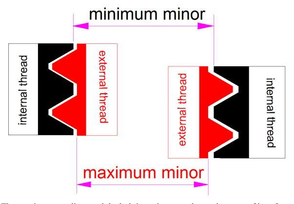
The previous case discussed the bolt jamming onto the nut because of interference at the major diameters. Now we will look at the possibility of jamming at the minor diameter.
