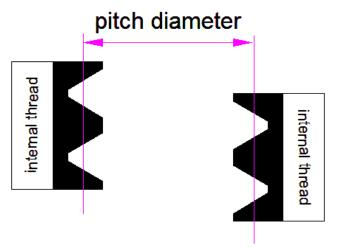
This should be followed by cutting the thread until the pitch diameter is in spec.
