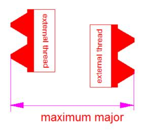
If it is smaller than the minimum, not enough thread will engage and the bolt may pull out of the nut when under axial load.
