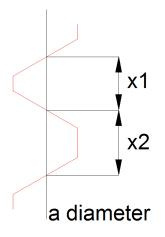
Pitch diameter is a rather odd duck in my opinion. It is a diameter determined by measuring thread features. Say this red line is the surface of an external thread. I measure the width of the groove or recessed part of the thread at a given diameter. Call this width  $x_1$ . Then I measure the width of the ridge at this same diameter. Call it  $x_2$ .
