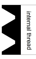
Sawing the nut in half across its face shows us the entire cross section. The right profile is offset by half from the left profile.
