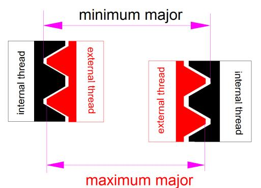
Consider the case of a bolt that is at its maximum major diameter. It must fit into a nut with a minimum major diameter. Even in this worst case situation, it all has to fit and not bind up.
