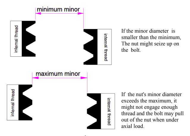
For a ¼-20 nut with a 2B thread class<sup>3</sup>, the minimum major diameter is 0.2500". The maximum major diameter is indirectly specified using other parameters that will be presented later.
