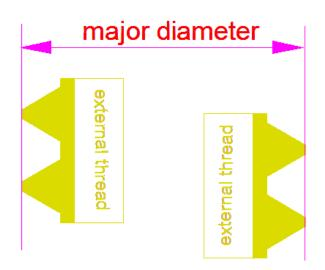
There are many ways<sup>5</sup> to single point cut a cylinder but the threading table implies to me that one should first turn the major diameter.
