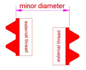
The final step is to verify and machine, if necessary, the minor diameter. If the cutter has the correct profile, there should not be a problem here.
