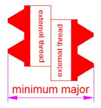
The diameter of the bolt measured from outside flats is called the major diameter. There is a maximum and minimum major diameter specified.
