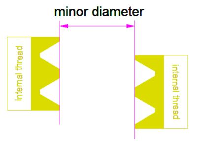
Again, following the threading table, I would start by drilling or boring the minor diameter.
