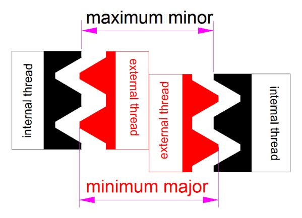
For a  $\frac{1}{4}$ -20 nut of thread class 2B at maximum minor diameter and a bolt of thread class 2A at minimum minor diameter, the engagement is 0.2500" - 0.196" = 0.054". This is the overlap between nut and bolt derived from subtracting diameters.
