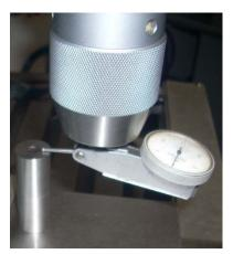
I then stacked a 1.0000" +/- 0.0002" spacer block on top and brought my DTI down until it again read zero. The DRO flickered between 0.9995" and 1.0000". So the error in the Z axis is most likely in the dial and not the DRO.
