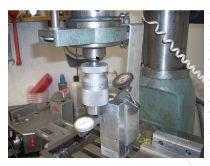
This first test looks at movement between the spindle and the quill. My DTI has been fitted into the drill chuck. I then rigged up some scrap aluminum that clamps to the lower spindle bearing which clamps to the quill. This aluminum contacts the DTI's finger. Note that the pressure exerted by the finger is tiny so this support is more than strong enough.
