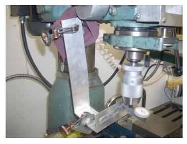
Next I moved my scrap aluminum so it was supported by the head. I am using a very strong magnet that was dug out of an old hard drive. In order to make it easier to pull off of the head, I have put down an old rag to separate them.
