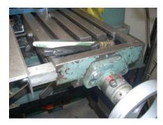
First I locked my X axis and turned my X axis feed handle unit I ran out of backlash. It is hard to explain, but it should be difficult to turn the handle further but you also don't want to force it *REAL* hard. If a "reasonable" amount of force causes the lock to slip, you may have a problem.
