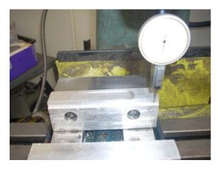
The first thing I did was check my fix softjaw<sup>3</sup> with a DTI attached to the spindle. Since it is cut in place and not moved, any error is due to play in my X axis ways and spindle. The DTI showed less than +/- 0.00025" of variation across the surface. No complaint there. This face was side milled so I do expect some variation.
