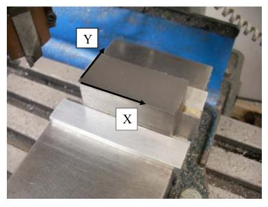
It is common practice with Computer Numerical Control (CNC) to define the Y axis pointing towards the back of the machine. Often the origin is on the left end of the *movable* jaw. As the Y value increases, we are moving across the part and away from the front of the machine.
