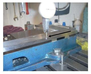
I then ran the DTI along the edge parallel to my Y axis. I saw less than +/- 0.0001" of needle movement over 4".
