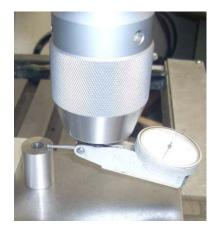
I attached my DTI to the spindle and brought it down on the end face of a spacer block. I then zeroed my DTI and DRO.
