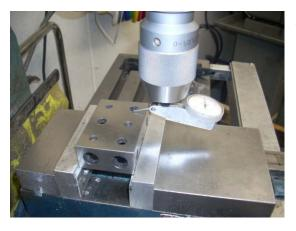
Next, position the DTI's finger so it is referencing the top of the block. With just finger pressure, lift up on the spindle and see if the DTI needle moves. Then push down and see if the DTI needle moves. Any motion could indicate that the spindle bearings has excessive play.
