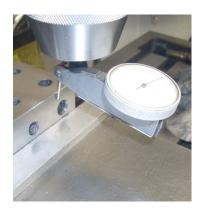
I have the DTI in the drill chuck with the Z axis locked. I then zeroed the DTI needle with the finger pressing on my block. I pressed on the front of the spindle and noted how much the DTI's needle moves. I then pulled on the spindle while monitoring the DTI to finish this part of the test. You should see movement if you push/pull hard enough. But light pressure should not cause any movement of the DTI's needle.
