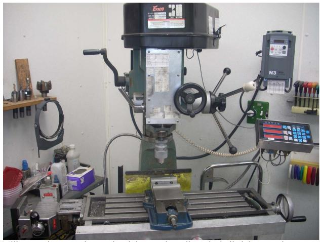
Mills come in many sizes and weights yet they all can be boiled down to the same simple model. All mills have a table that moves left and right along what is called the X axis. The table can also move front and back along the Y axis. Filling out the set we have the ability to change the distance between table and cutter along the Z axis. This distance can be changed by moving the quill and, on some mills, the knee.
