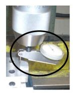
You will need a finger style Dial Test Indicator and a means of connecting it to the spindle and to other surfaces near the axes. You will also need a way to stop the spindle from rotating. I just use a small wedge of wood that jams between the front of the belt cover and the pulley. Just remember to remove it before starting up the motor.
