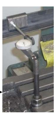
Now I slowly but firmly apply pressure to the front left and back right corners of the table in an effort to rotate it about its center. I first push and then pull in order to sweep through any play in the X axis ways.
